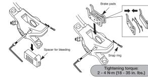
2. Depress the brake lever so that the rotor is being clamped by the pads, and then tighten the
