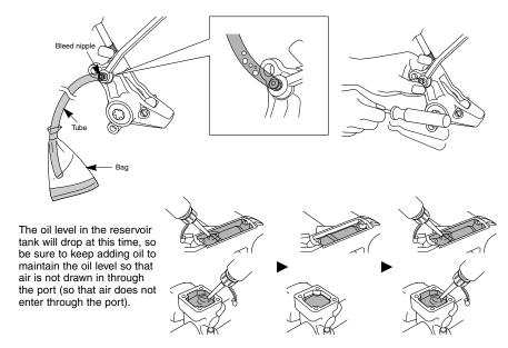
6. Once air stops coming out from the bleed nipple, temporarily tighten the bleed nipple.
