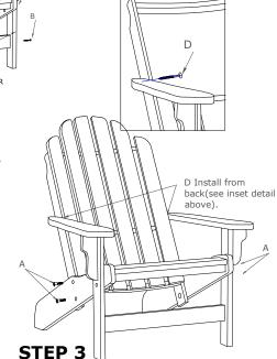
Bolt back assembly to base assembly using 2 bolts (A) on each side as shown. Attach arm to seat back using Large Head Screws (D).
