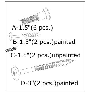
Attach spreader to legs with screws (B) as shown. Bolt legs with arms to base assembly using bolts (A).
