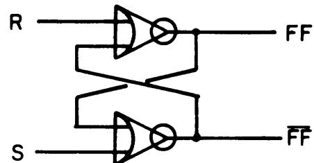
DC Flip-Flops may also be implemented and shown as BUFFER LATCH circuits:
