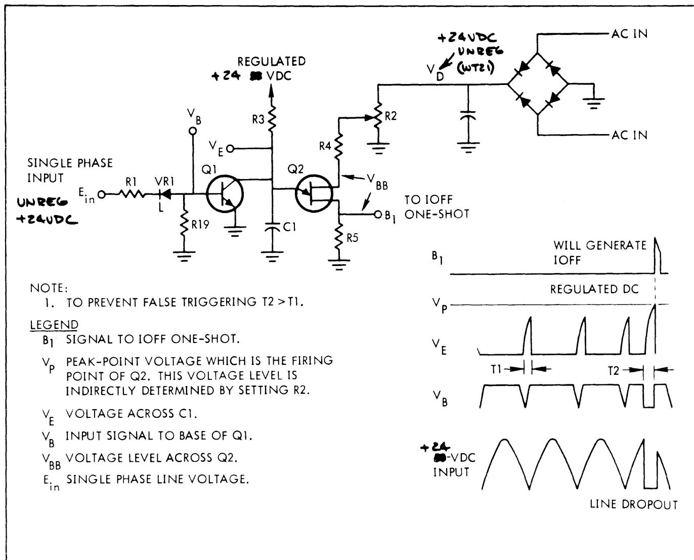
Figure 3-646. Single-Phase Detection
