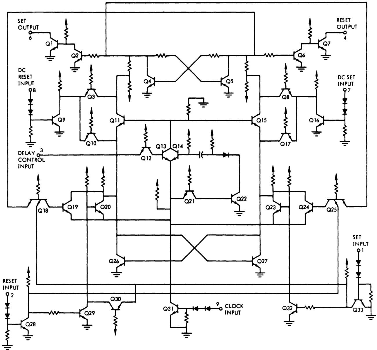
SDS311 Flip-Flop Schematic Diagram
