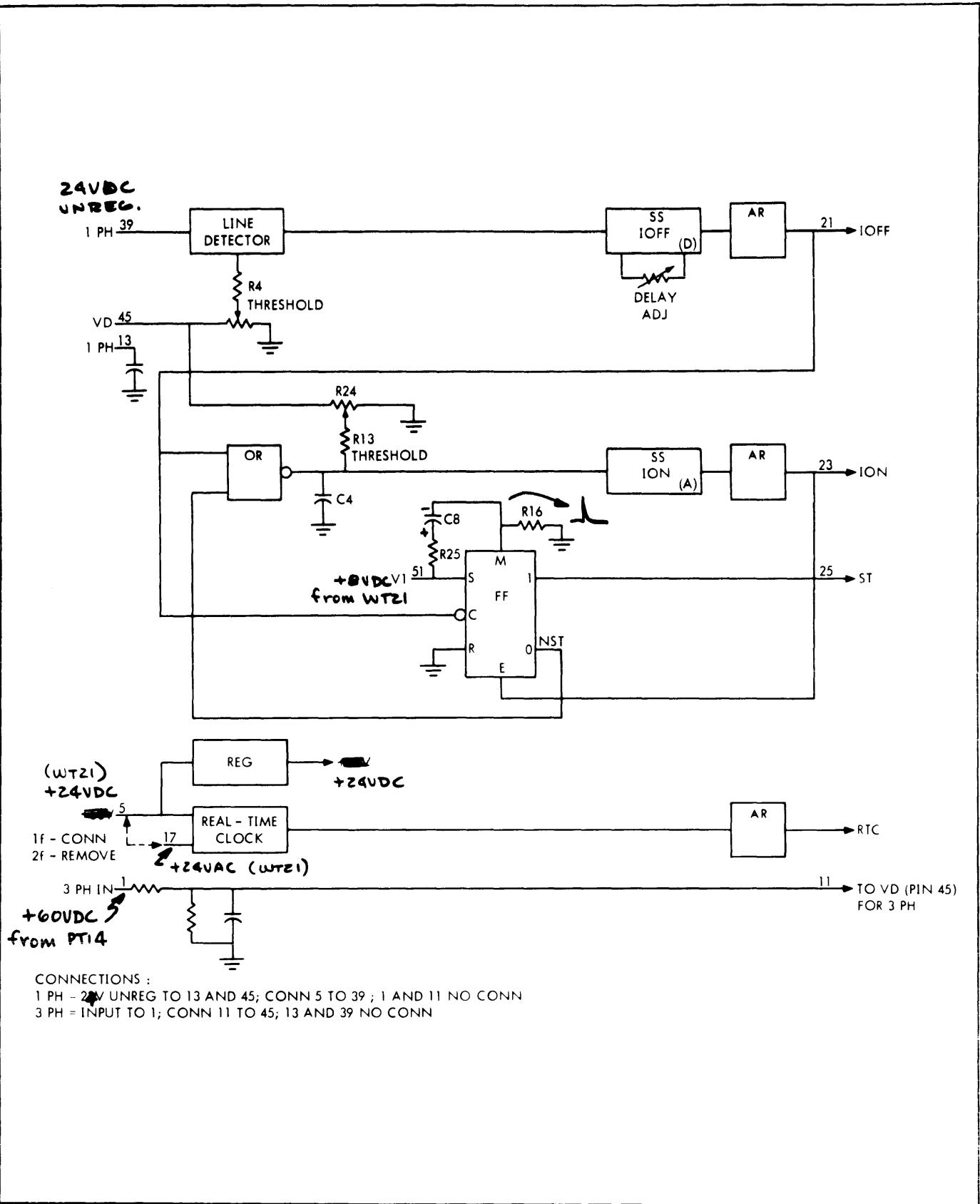
Figure 3-643. WT22 Line Detector, Block Diagram
