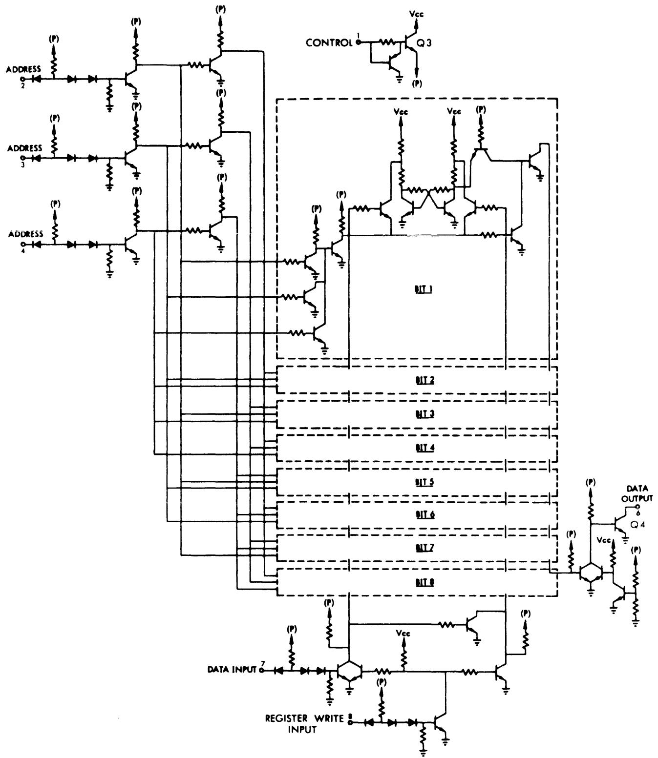
SDS304 Memory Element Schematic Diagram
