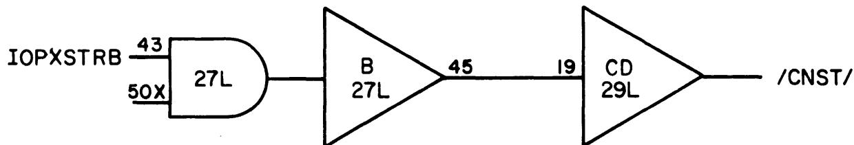
If a logic function must use more than one logic line, then each successive logic line is followed by its own pin line. Each pin line will indicate which module location the following pin numbers relate to, even though all of the pins are on the same module. Thus:
