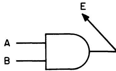
"E" means that the output of this circuit is an extension to the input of another circuit at some point other than its "normal" input.
