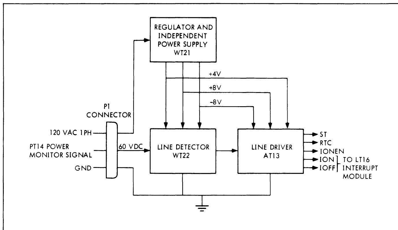
Figure 3-640. Power Fail-Safe Feature, Simplified Block Diagram
