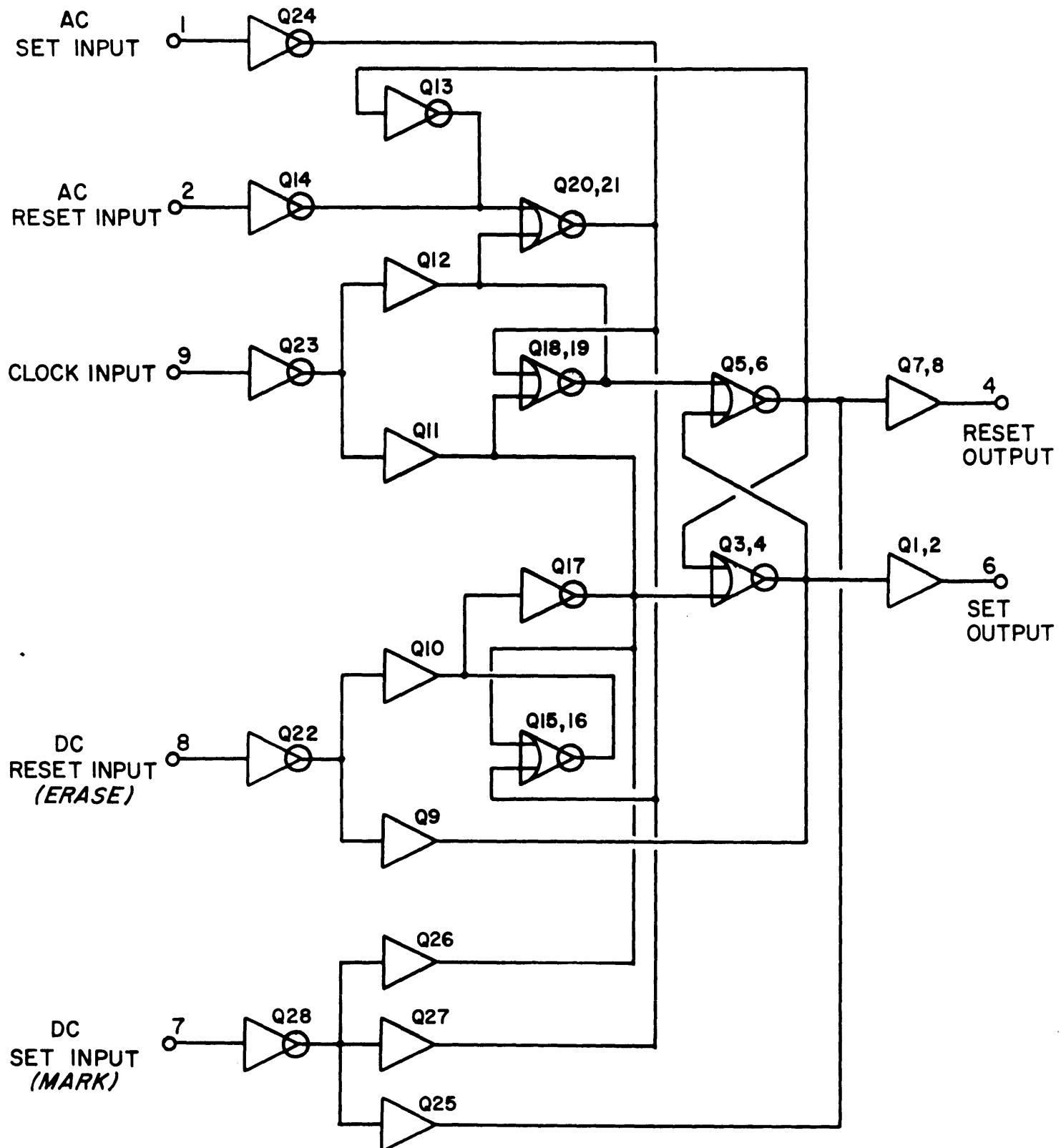
SIMPLIFIED LOGIC DIAGRAM, SDS 307
