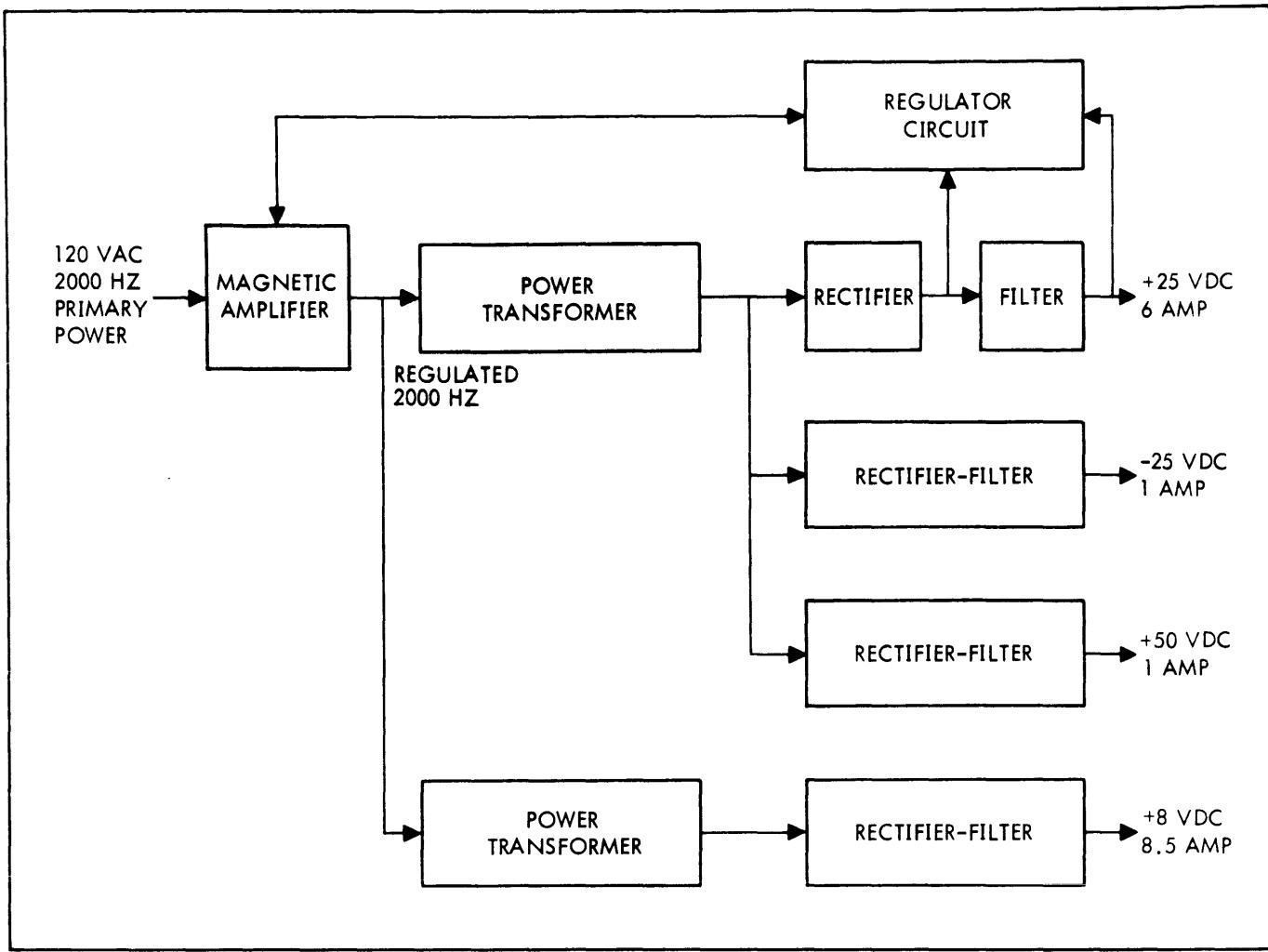
Figure 1-2. Power Supply Model PT-18 Functional Block Diagram
