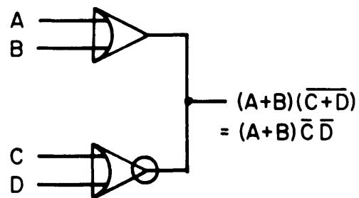
Note: If one element has a OVDC output (output transistor conducting), then the output line is clamped at OVDC.
