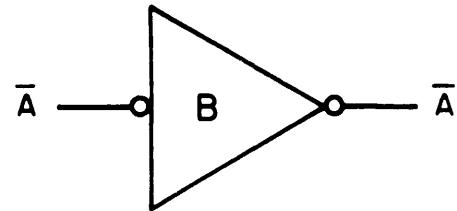
"O" symbol indicates a logic "0"(0VDC), its absence indicates a logic "1"(+4VDC)
