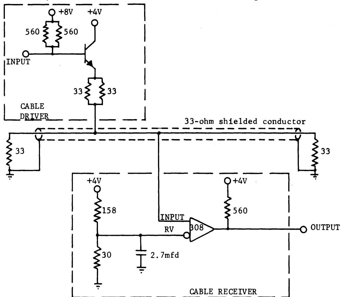
The input to the SDS 308 represents a high impedance to the line, causing a load of approx. 50 microamps to be absorbed. One Cable Driver can drive up to 25 Cable Receivers, however, the limit of 200 feet lengths for the 33-ohm cable normally is reached before this number of Cable Receivers can be connected to the cable.
