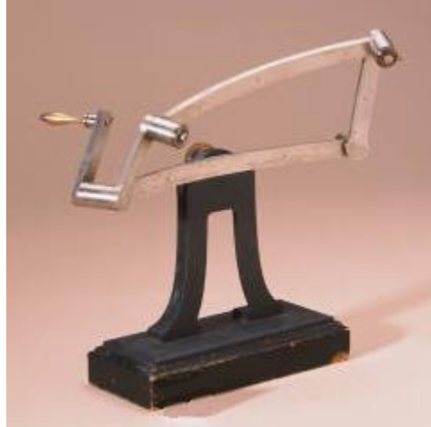
Figure 3: a mechanism with four joints; at most three can be mobilizers unless you break one of the bodies.
