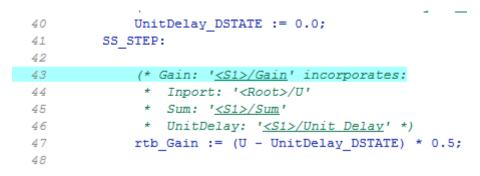
In the report, the highlighted tag S1/Gain indicates the beginning of the generated code for the block. You can use the same method to trace from other Simulink, Stateflow and MATLAB objects to the generated traceability report.
