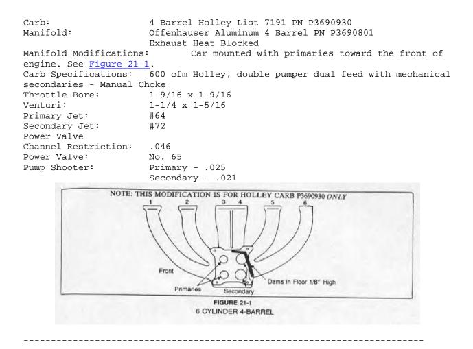
Note: For general multi-purpose or brackets, the previous carb set-up is recommended. This package is for all-out racing only.
