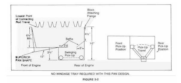
The in-car clearances should always be checked carefully before making the pan. The important items to watch for are header clearance, steering linkage clearance, K-member clearance, and ground clearance. The K-member will interfere with the front requiring a notch in the front of the pan or in the K-member. Any notch put in the pan should be kept to an absolute minimum or eliminated completely if at all possible.
