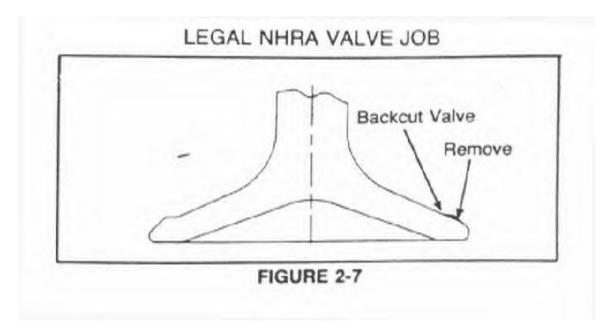
Backcut angles vary from 20 to 35 degrees depending upon the engine. Backcut valves are available for the 6 cylinder engines (see section 2). Backcutting the valve tends to make the valve seat narrower, for which we strongly recommend that bronzewall valve guides be installed in the head.
