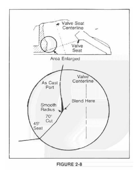
This sharp edge should be removed very carefully with a hand grinder so that it blends smoothly into both the cast port and the 70 degree machined cut. It is very important to keep to a minimum the metal removed and to maintain the 70 degree cut - although it may be narrower than it was originally. Extra caution should be used on the port's "short side" to keep as much radius as possible.
