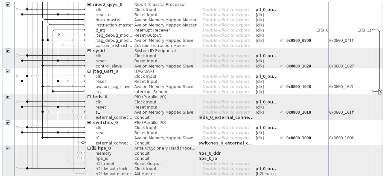
Figure 9-13. Adding the "Standalone" HPS to the System
