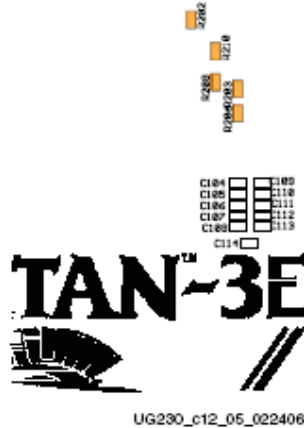
Figure 15-5: Location of Termination Resistor Pads on Bottom Side of Board Using Differential Outputs
