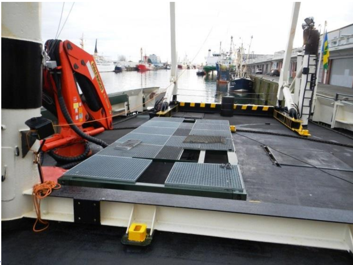
Aft deck with Palfinger Crane and fittings for 3 x 20 feet containers
