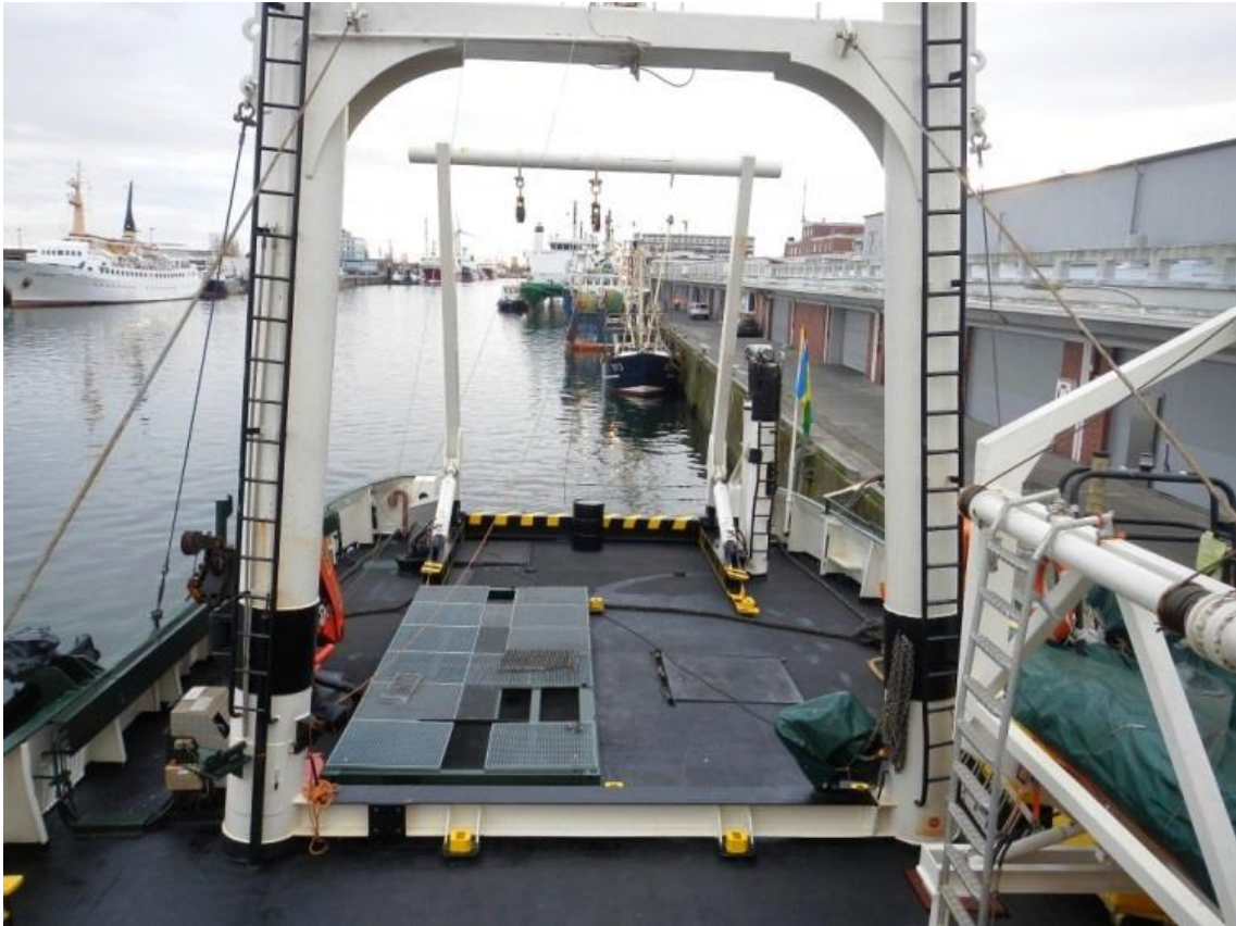
Aft deck with A-frame for 8 ton
