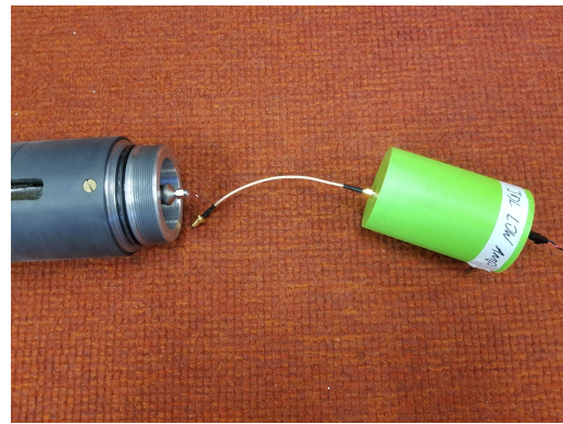
(b) Using a SMA cable, only needed for the IDL pulser.
