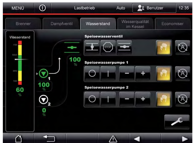
Representation of the setting level for a feedwater control valve
