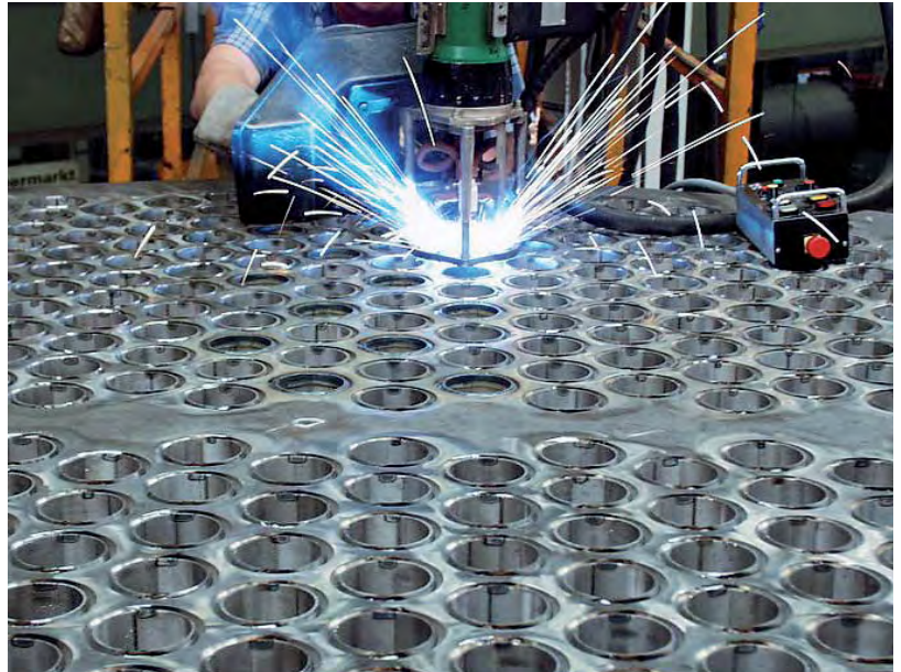
Welding the smoke tube with mechanical welding equipment
