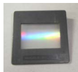
diffraction grating (300 or 600 lines/mm)
