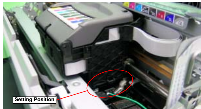
Figure 5-11. Moving the Carriage Unit
