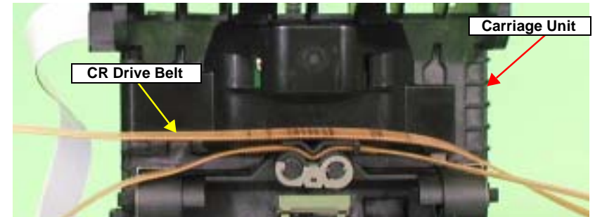
Figure 4-69. Removing the CR Drive Belt
