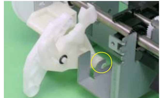
Figure 4-94. Removing the Left CD-R Release Lever Sub Assy (2)
