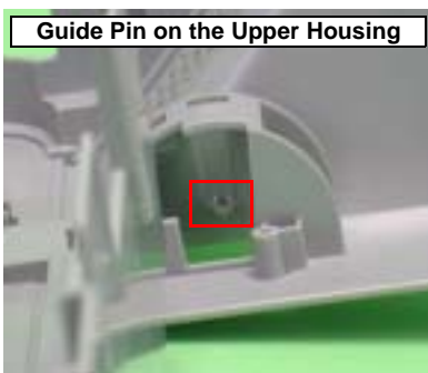
Figure 4-10. Removing the Printer Cover
