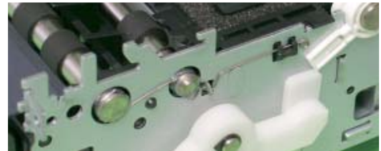
Figure 4-115. Reinstalling the EJ Grounding Spring
