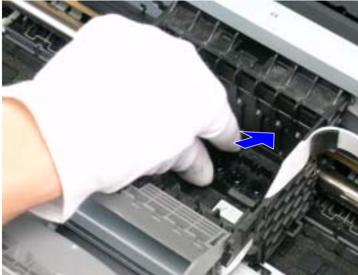
Figure 4-37. Reinstalling the Print Head (2)
