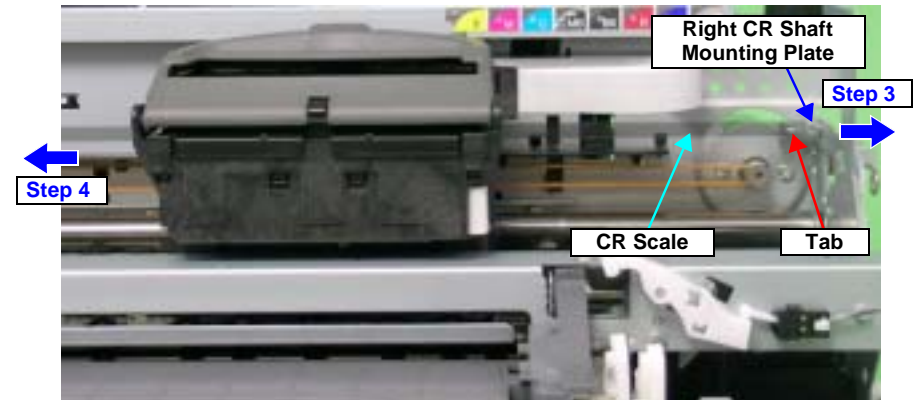
Figure 4-38. Drawing Out the CR Scale
