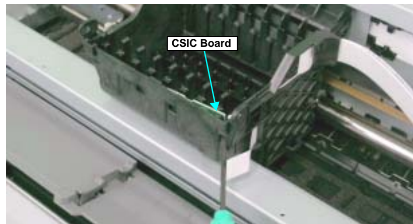
Figure 4-81. Removing CSIC Board
