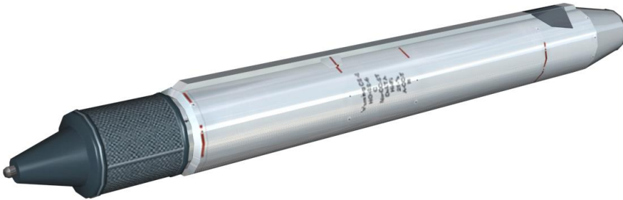
Figure 92: S-25 Unguided Rocket in its Launch Tube
