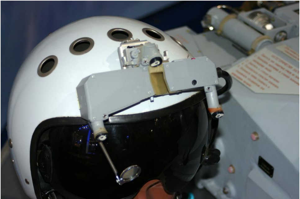
Figure 19: "Shchel-3UM-1" Helmet-mounted Target acquisition System
