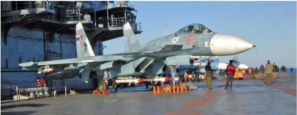
Figure 22: Su-33 on the Kuznetsov deck with two R-27ERs under the inlets and two R-73 under wings
