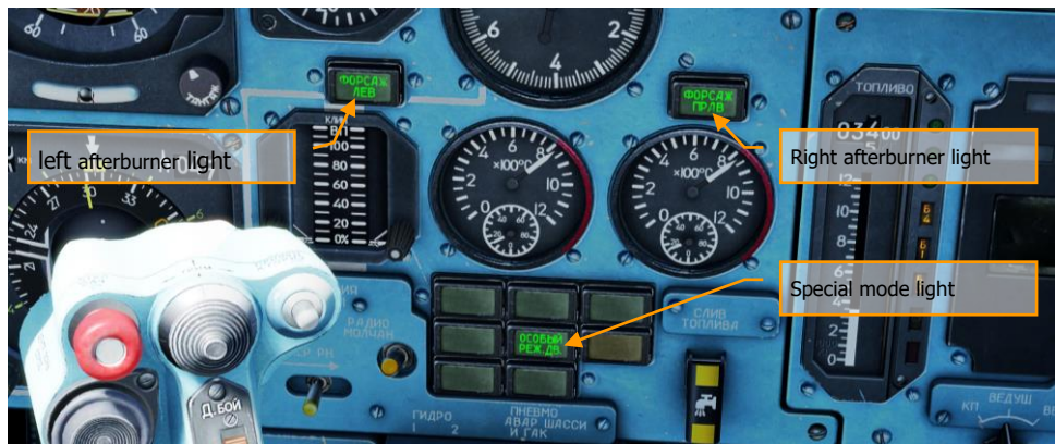
Figure 93: Afterburner and special mode lights
