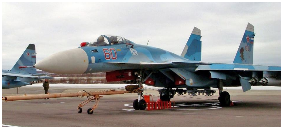
Figure 23: MBD3 multi-bomb racks under inlets and B8 rocket launchers on double racks under wings
