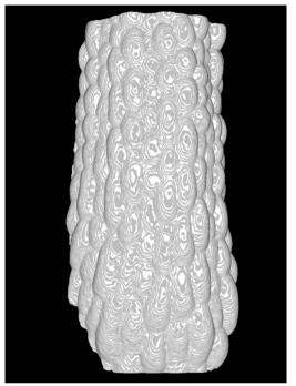
Good: Smooth continuous surface Gaussian Blur = 3 Threshold = 15
