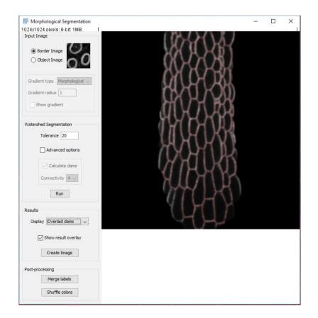
4. The automatic segmentation in step 3 may not be adequate (over- or under-segmentation). Check the segmentation and if necessary, re-run it. You can empirically find the best "Watershed Segmentation Tolerance" value (see image above in the red rectangle, in this case the value was changed to 20) and re-run the segmentation as many times as necessary. When you are satisfied click "OK" in the window below.
