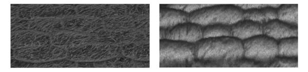
Left is the x,y view (from the top in Fiji 3D viewer) while right is the y,z view (from the side), showing the anisotropic nature of the confocal signal.
