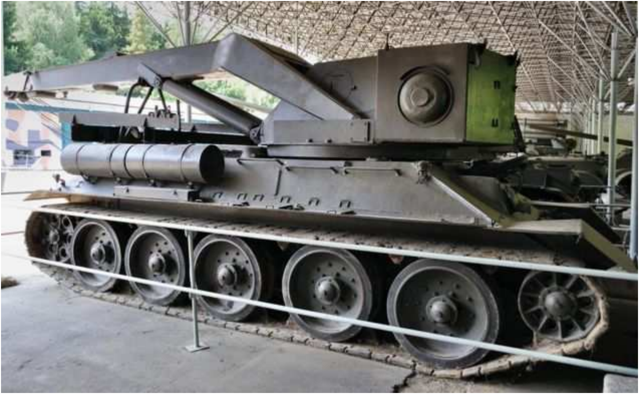
JT-34 – Army Technical Museum, Lesany (Czech Republic) Czechoslovakian version of turretless T-34 fitted with crane of high capacity
