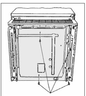
Figure 5-12: Bottom Cover Screws
