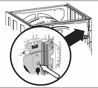
Figure 5-14: Residual Moisture Sensor and Screw
