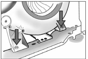
Figure 5-11: Fan Motor Bolts
