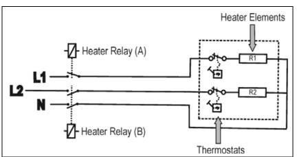
Figure 4-6: Heater Circuit
