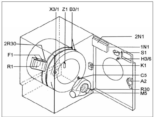
Figure 1-13: T 1576 Component Layout
