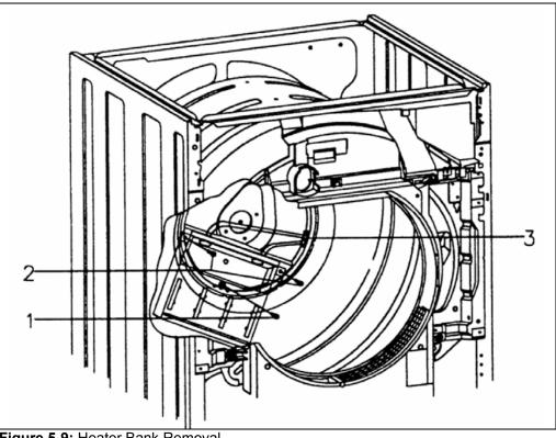
Figure 5-9: Heater Bank Removal
