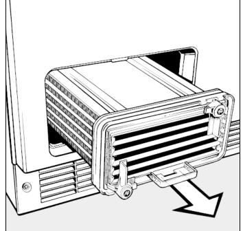
Figure 3-3: Removing the Heat Exchanger
