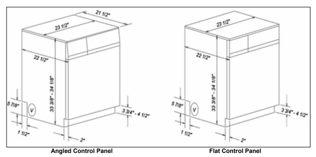
Figure 1-9: Dimensions, 5-Kilogram Vented Models
