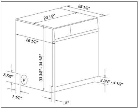
Figure 1-11: Dimensions, 6-Kilogram Vented Models
