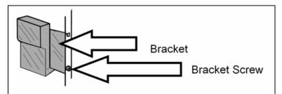
Figure 5-6: Heater Relay Bracket
