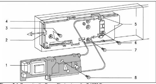
Figure 5-4: Removing the Power Electronic on the T 1576 Dryer
