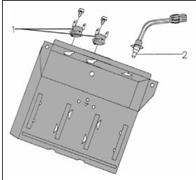
$1 \ \, Temperature \ \, limiters \ \, (2) \\ 2 \ \, NTC \ \, temperature \ \, sensor \ \, (T \ \, 1576 \ \, only) \\ (100 k\Omega \ \, @ \ \, 75^\circ F)$
