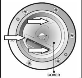
Figure 5-8: Heater Bank Cover Retaining Bolts
