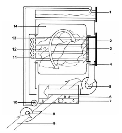
Figure 4-2: Condenser Dryer Airflow
