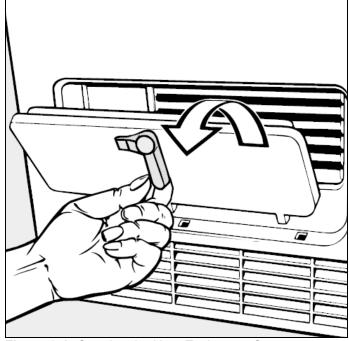
Figure 3-1: Opening the Heat Exchanger Cover
