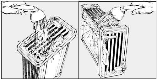
Figure 3-4: Cleaning the Heat Exchanger
