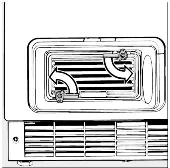
Figure 3-2: Positioning the Heater Exchanger Levers
