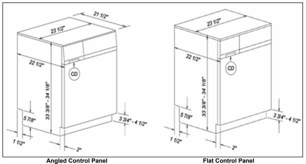
Figure 1-10: Dimensions, 5-Kilogram Condenser Models
