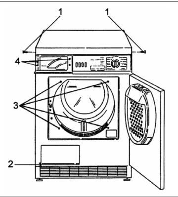
Figure 5-1: Lid Removal and Front Panel Access
