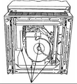
Figure 5-13: Condenser Fan Screws
