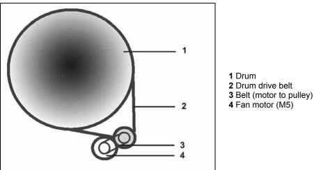
Figure 4-4: Drum Drive Belts and Reduction Pulley
