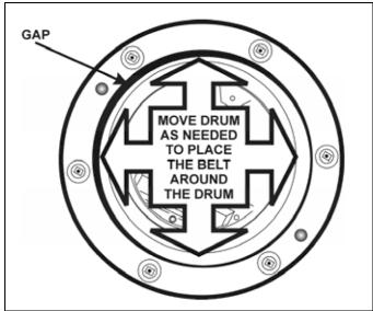
Figure 5-15: Positioning the Drum to Form a Gap
