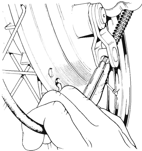
Fig. D12. Front brake cable abutment.
