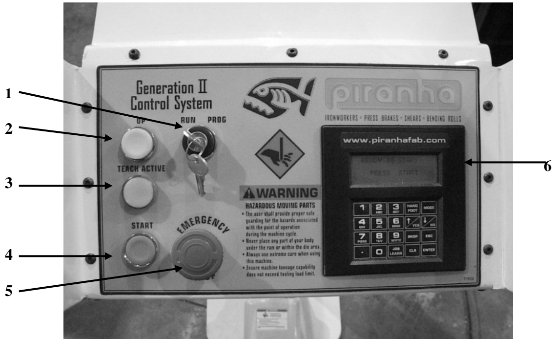
Fig. 8: Generation II Pedestal Control Unit
