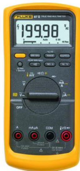
Figure B.1: Communal DMM (model 87V Fluke). Note that you may have a different model at your individual station, but the symbols for the settings are the same. The \Omega symbol (center position) allows to measure resistance. The yellow symbol with one vertical line, and another slightly curved one (next to the \Omega symbol) allows to measure capacitance. You must press the yellow function button to access it.
