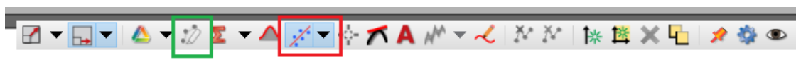
Figure 2.5: Graphing toolbar. The toolbar appears when moving the mouse to the top of the graph. The red boxed icon is the Curve fitting tool. Select the “Natural Exponential” function. The highlighting tool is boxed in green. This allows to select a smaller subset of data to apply the curve fitting.
