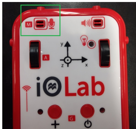
Figure 3.6: Position of the magnetometer on the IOLab (green box). Place the compass on top at this position to obtain precisely the direction of the magnetic field detected by the IOLab.
