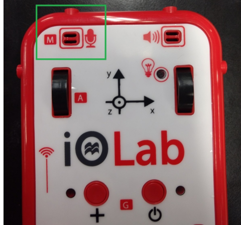
Figure 5.7: Position of the magnetometer on the IO Lab (green box). Place the compass on top at this position to obtain precisely the direction of the magnetic field detected by the IO Lab.
