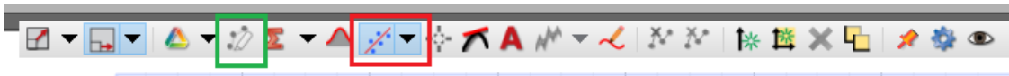
Figure 4.5: Graphing toolbar. The toolbar appears when moving the mouse to the top of the graph. The red boxed icon is the Curve fitting tool. Select the “Natural Exponential” function. The highlighting tool is boxed in green. This allows to select a smaller subset of data to apply the curve fitting.
