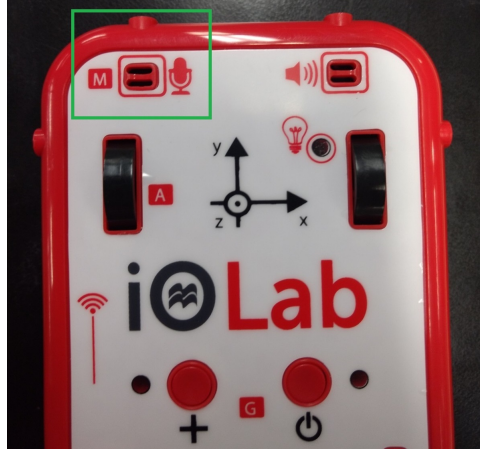
Figure 3.7: Position of the magnetometer on the IOLab (green box). Place the compass on top at this position to obtain precisely the direction of the magnetic field detected by the IOLab.
