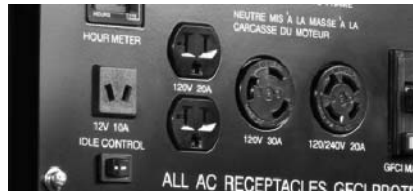
Full GFCI protected control panel makes generator OSHA compliant. Automatic idle control saves fuel and reduces noise by idling down engine when not in use
