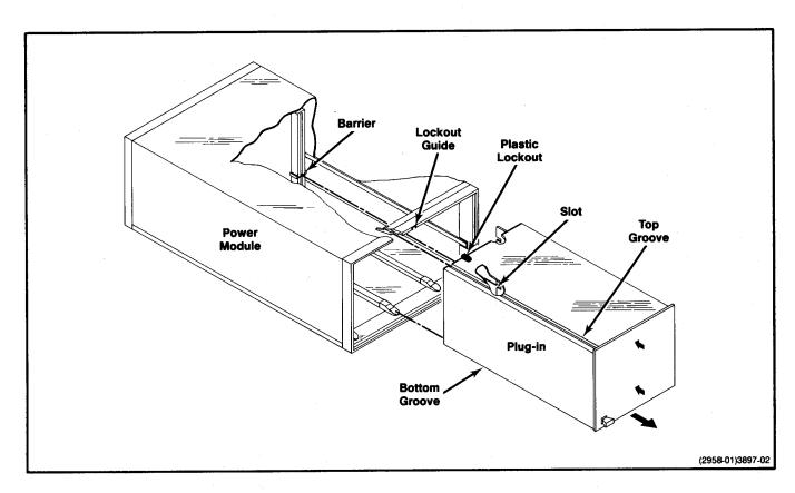
Fig. 2-1. Plug-in installation and removal.
