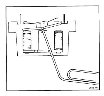
Fig. 5-2. Method of removing magnetic latch relay armature.
