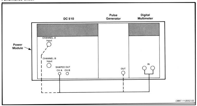
Fig. 4-1. Performance Check setup for step 3.
