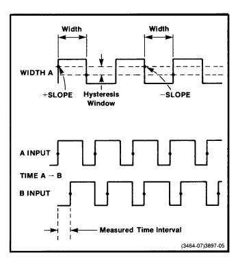
Fig. 2-5. Measurement examples for WIDTH A and TIME  $A \rightarrow B$ .
