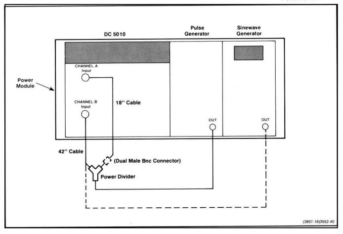
Fig. 4-6. Performance Check setup for step 15.
