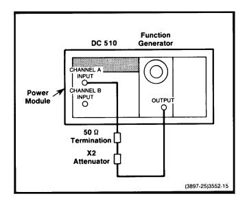
Fig. 8-4. Adjustment setup for steps 12 and 13.
