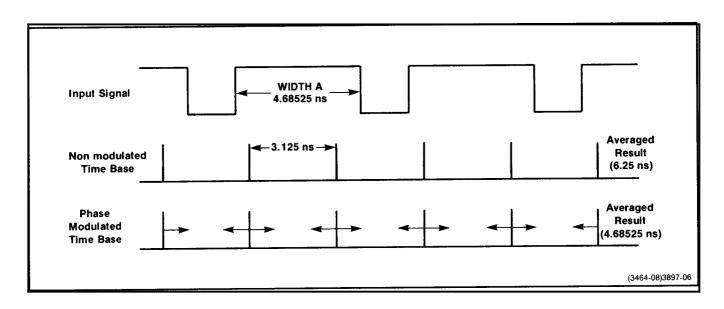
Fig. 2-6. Measurement example for synchronous input signals.
