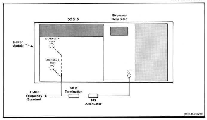
Fig. 4-5. Performance Check setup for steps 8, 9, 10, 11, 12, and 13.
