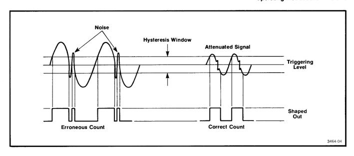
Fig. 2-3. Advantages in signal attenuation.
