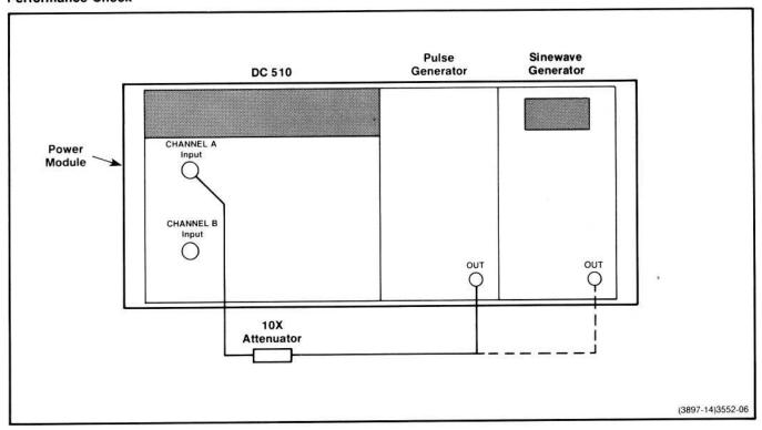
Fig. 4-3. Performance Check setup for steps 5 and 14.
