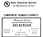
Chassis mounted components have no Assembly Number prefix—see end of Replaceable Electrical Parts List B | C |
