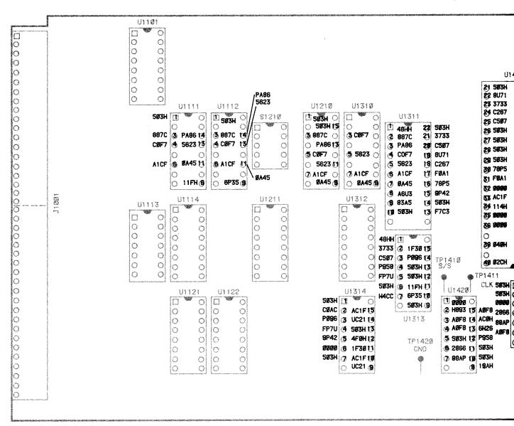
Fig. 8-7. Internal signature analysis "B" (Digital board)
