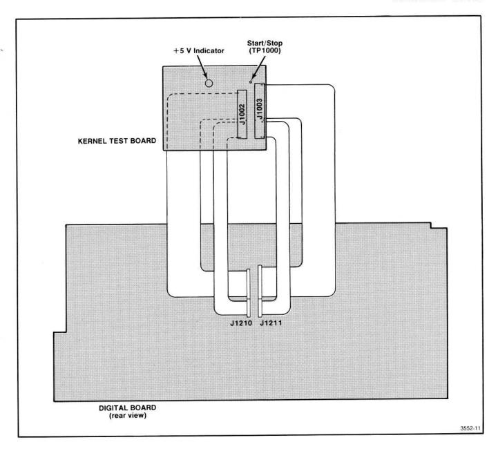
Fig. 5-8. Kernel signature analysis connections.
