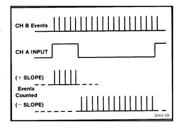
Fig. 2-7. Measurement example, EVENTS B DURING A.
