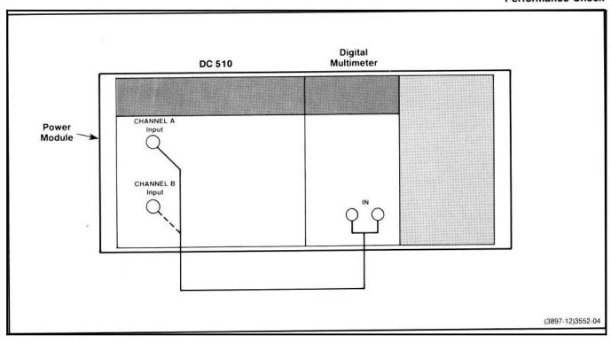
Fig. 4-2. Performance Check setup for steps 4 and 7.
