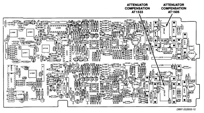
Fig. 8-1. Analog Board (A12).
