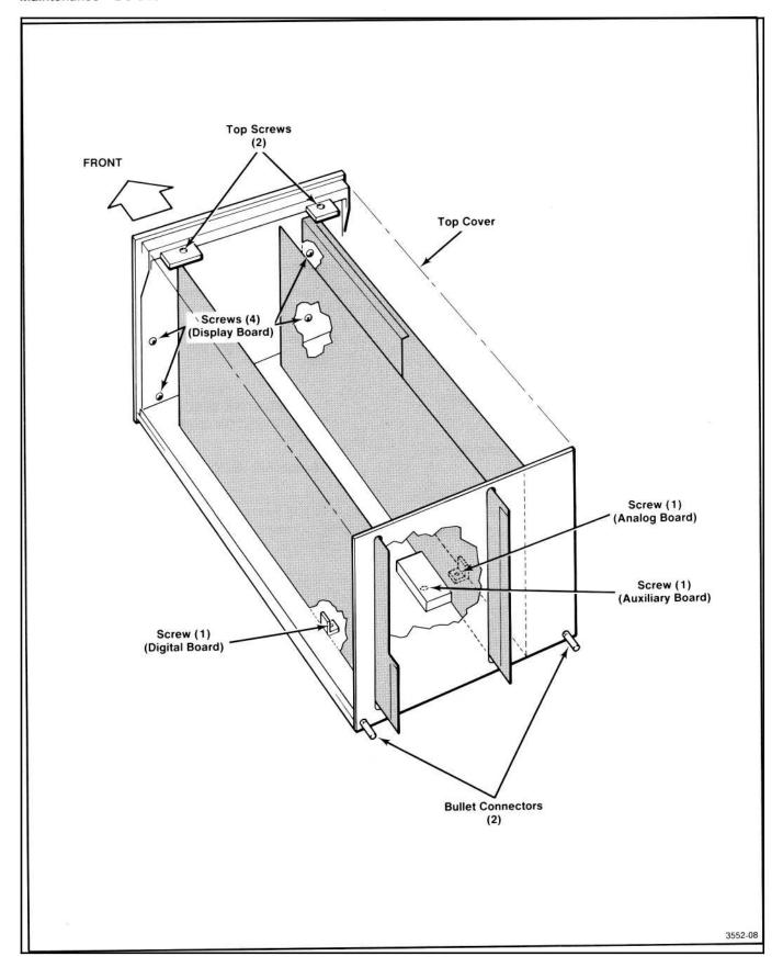
Fig. 5-1. Circuit boards removal and replacement.
