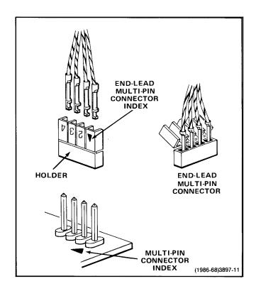
Fig. 5-5. Orientation and disassembly of multipin connectors.
