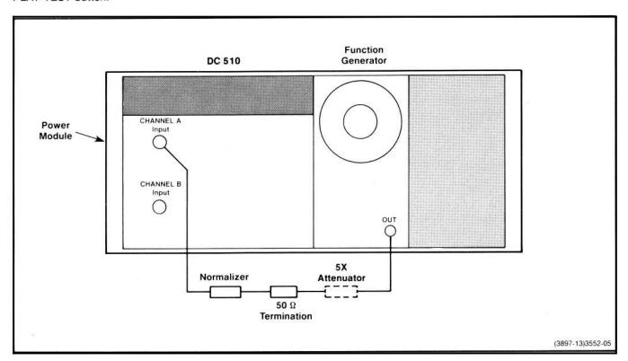
Fig. 4-4. Performance Check setup for step 6.
