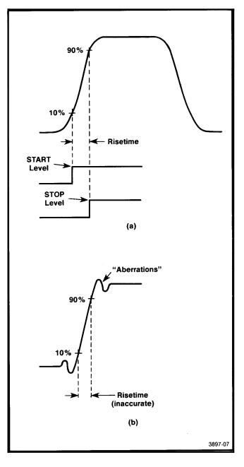
Fig. 2-8. Measurement example for risetime.
