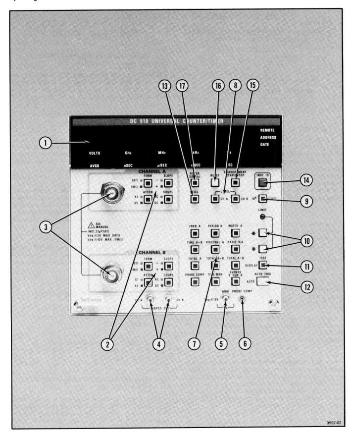
Fig. 2-2. DC 510 front panel display, controls and connectors.
