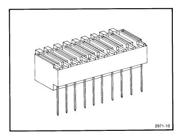
Fig. 5-4. Bottom entry circuit board pin socket.
