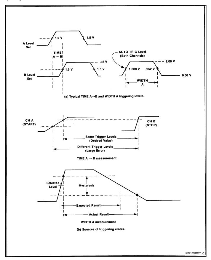
Fig. 2-4. Typical triggering levels and sources of triggering errors.
