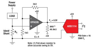
High-side current sensing techniques connect the current sense element between the supply and the load.
