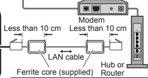
**Installing the Ferrite core**
