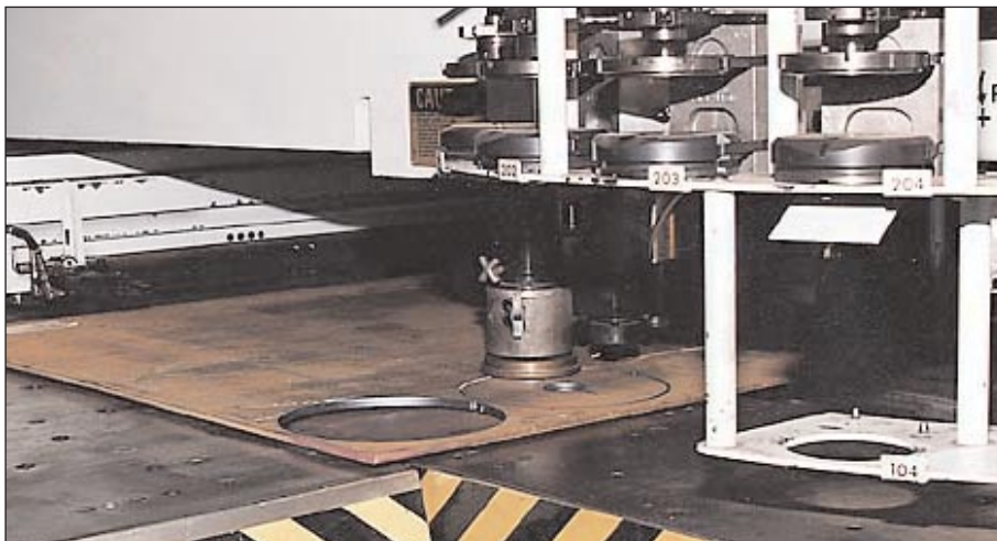
Dross-free parts cut with the 3700 ATC's TRUECut Oxygen Plasma Cutting System reduced part clean-up. Ninety percent of the parts from the Whitney go directly to welding, a press brake or other process.
