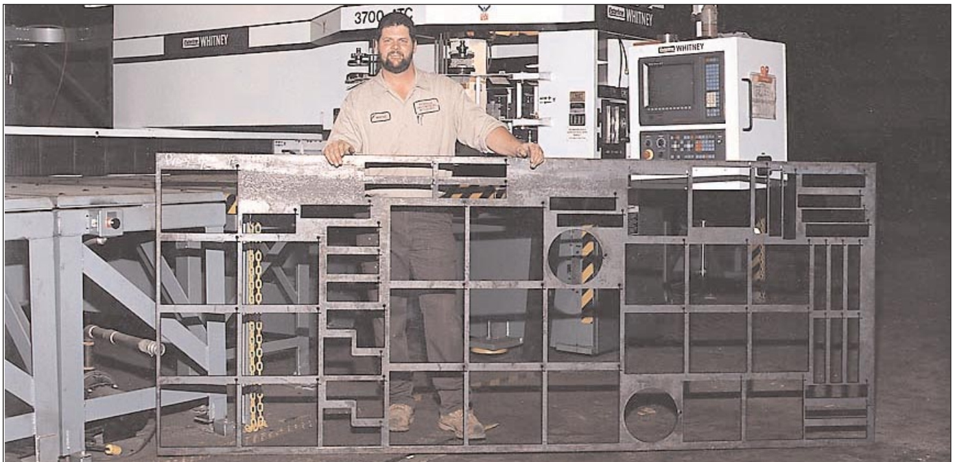
Wayne Tyler, T.I.W. 3700 ATC Operator, supports one of the skeletons showing the efficient plate utilization with the nesting capabilities of Building Block software. Wayne attended training at the Rockford, IL facility to learn how to run and maintain the machine.
