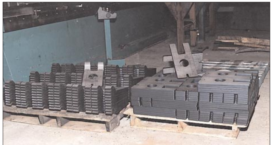
Parts shown are produced on the Whitney and go directly to the press brake for forming.
