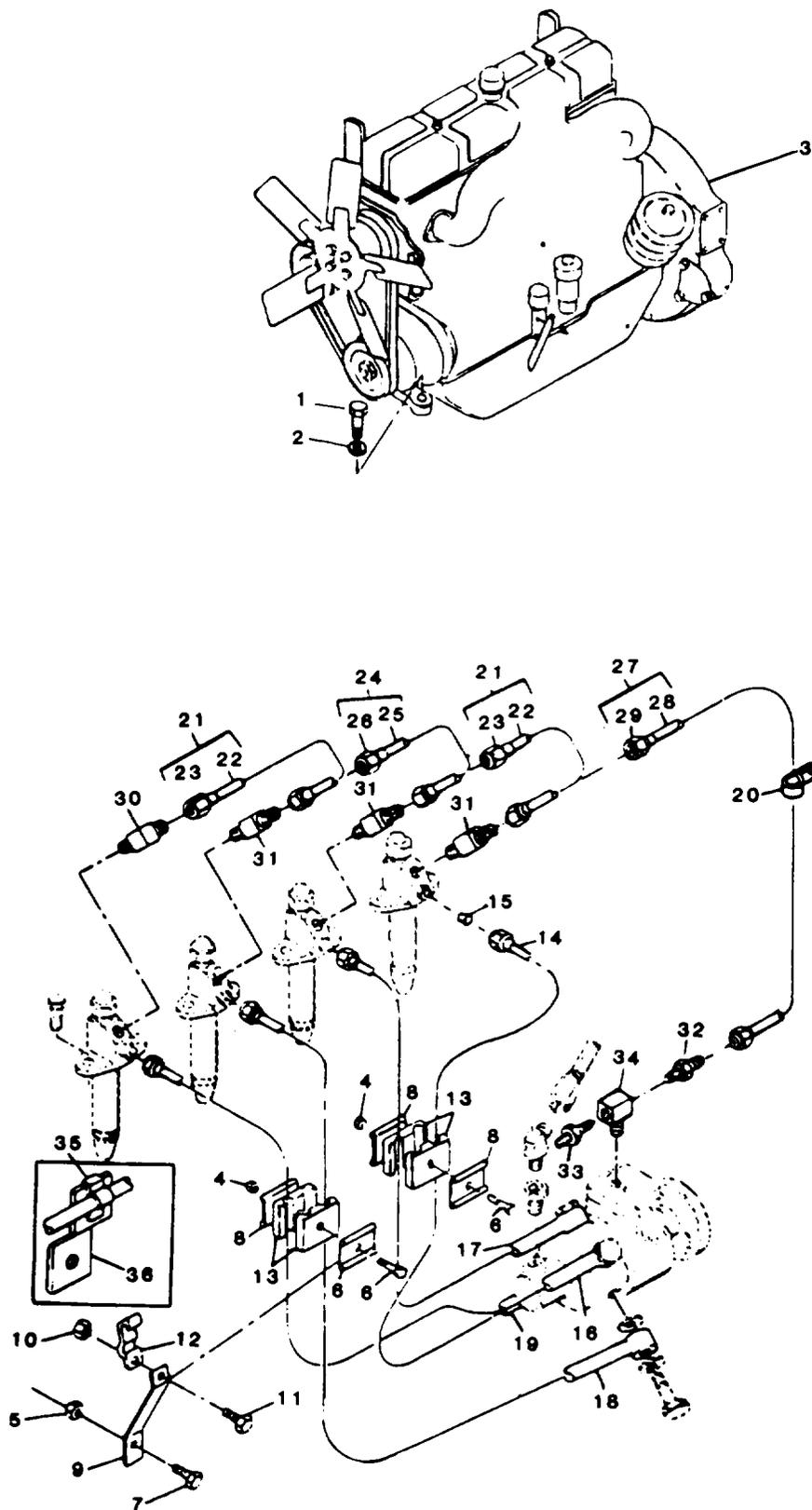
Figure 64. Engine Assembly and Fuel Injection System
