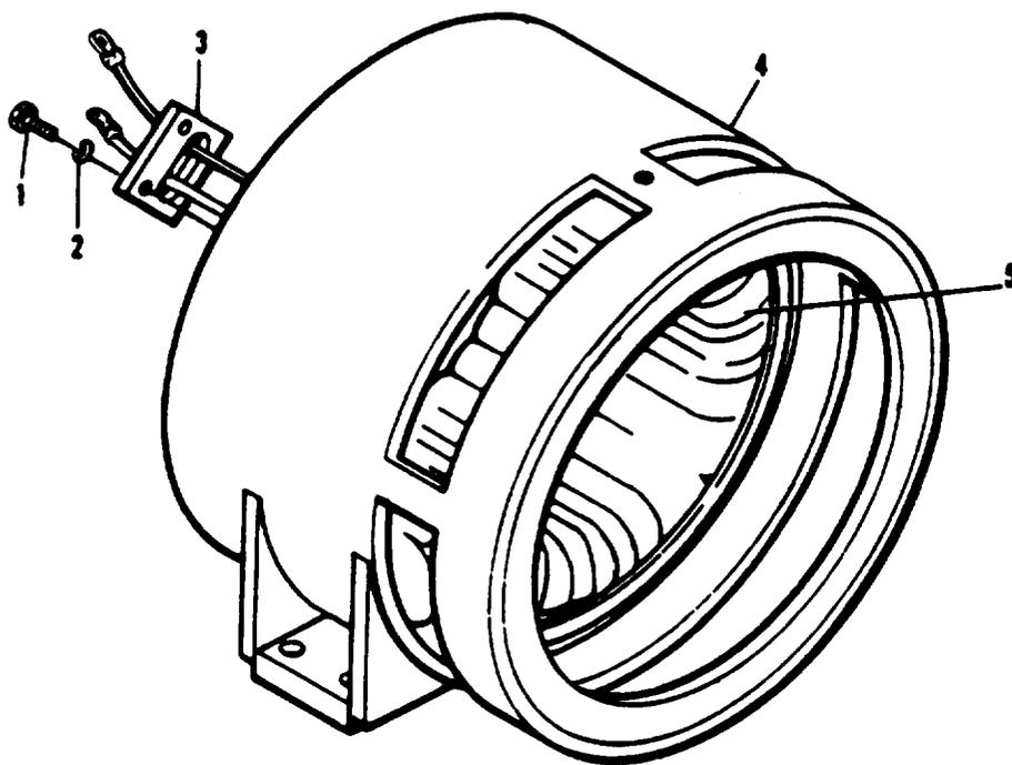
Figure 44. 50/60 Hz Stator Assembly
