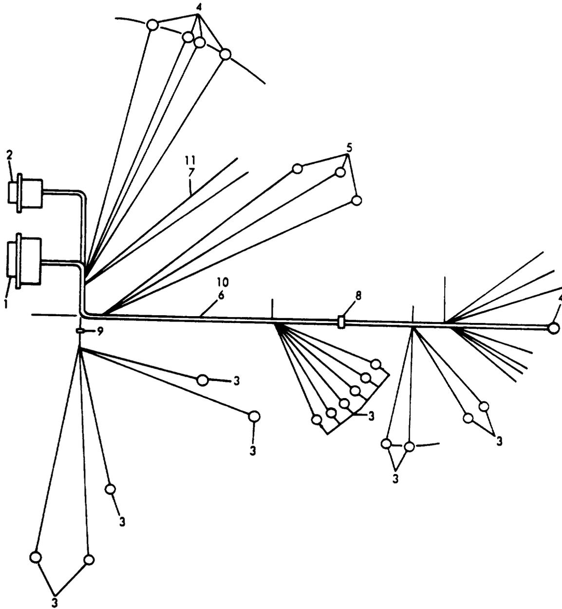
Figure 93. Electric Heater Control Box Wiring Harness
