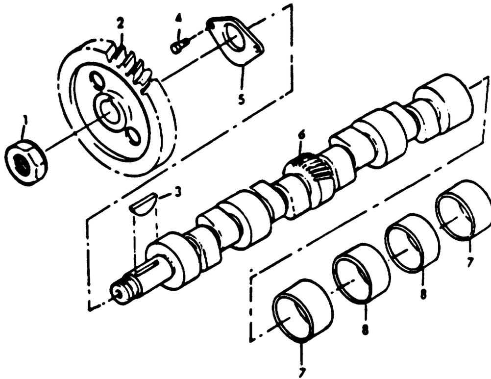
Figure 81. Camshaft, Timing Gear, and Bearings
