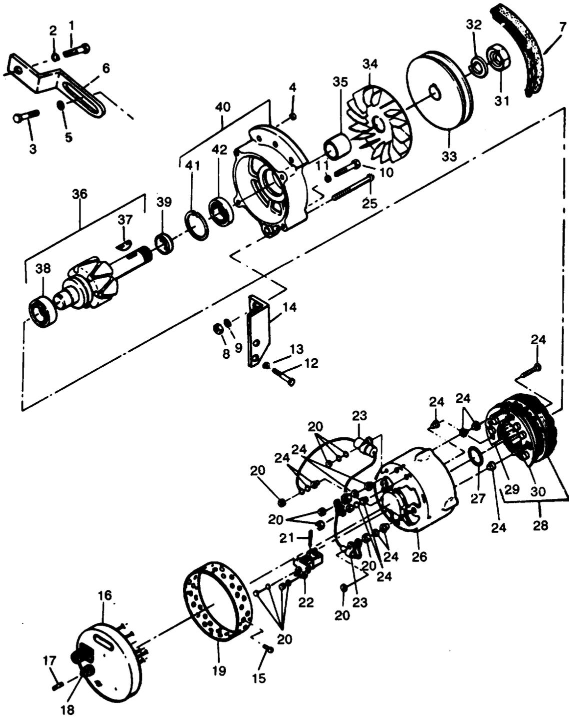
Figure 57. Battery charging alternator
