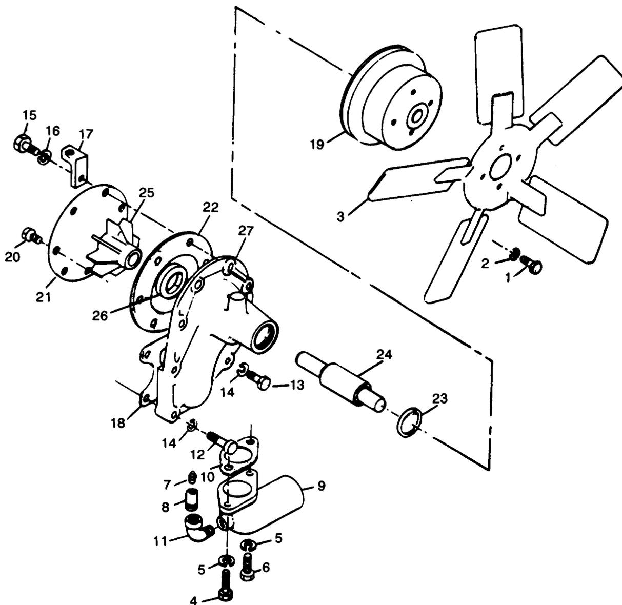
Figure 73. Fan and Water Pump Assembly
