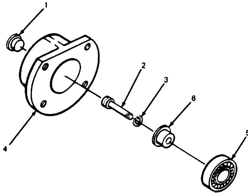
Figure 41. Bearing Assembly
