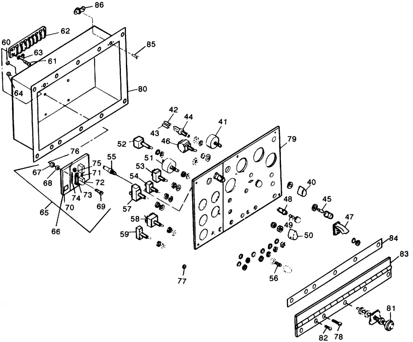
Figure 8. Control Cubicle Assembly and Manual Speed Control (Sheet 2 of 2)
