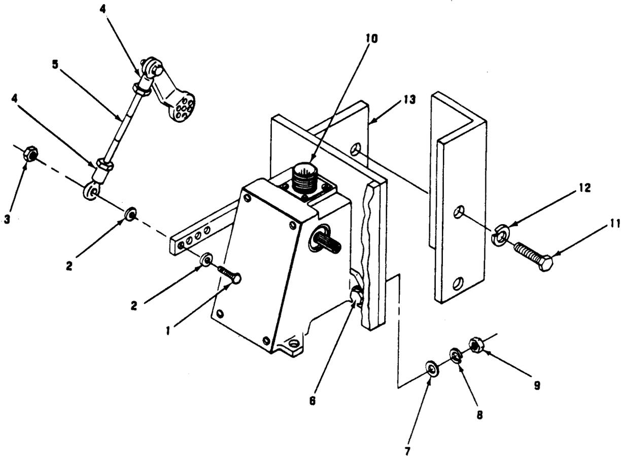
Figure 24. Electric Actuator Unit (400 HZ Sets Only)
