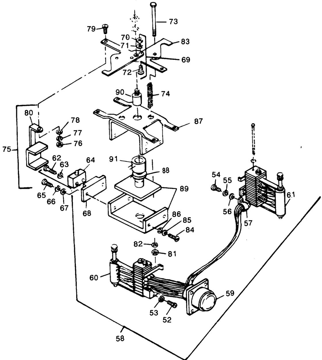
Figure 18. Main Load Contactor (Sheet 3 of 4)
