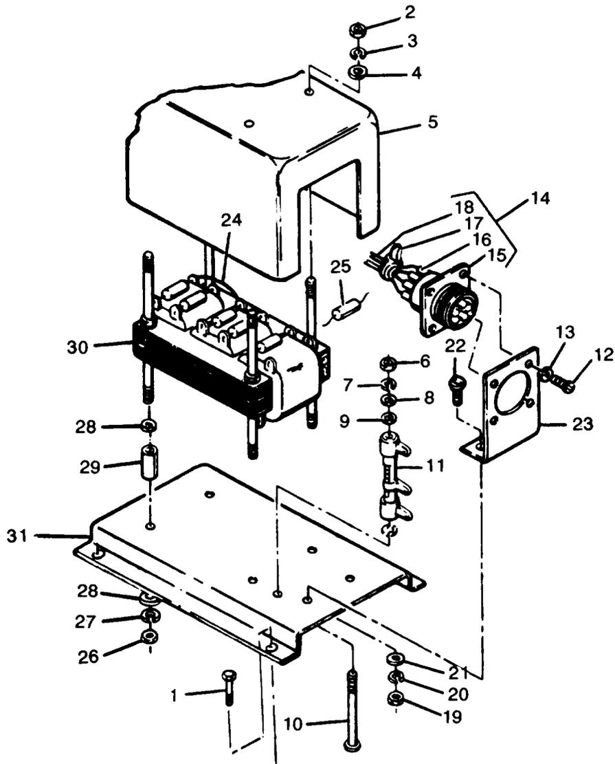
Figure 36. Load Measuring Unit
