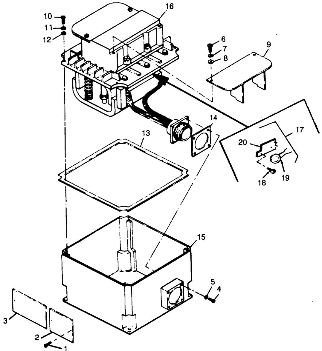
Figure 18. Main Load Contactor (Sheet 1 of 4)
