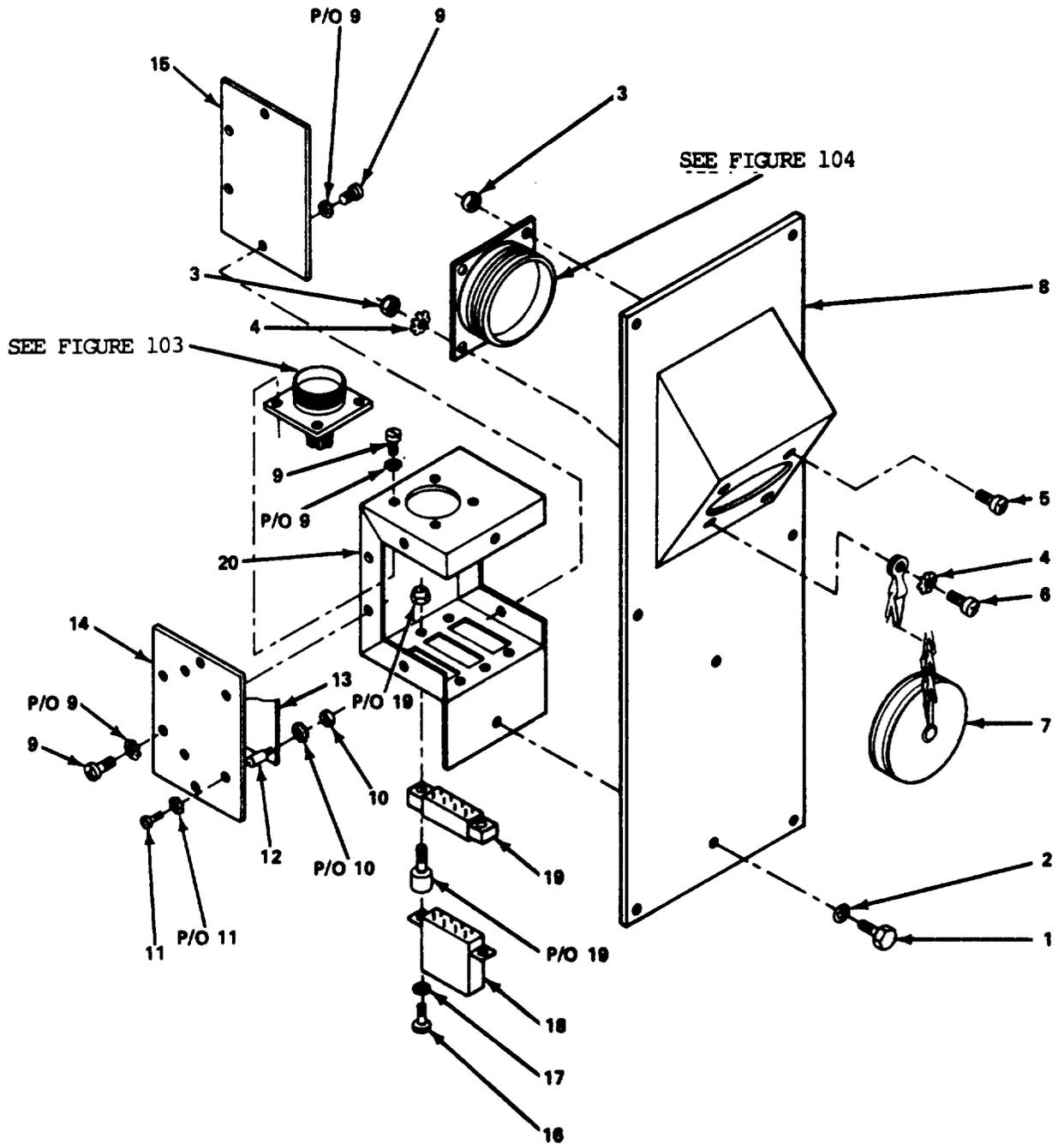
Figure 105. Connector Plate Assembly and Cover Plate Assembly (Sheet 1 of 2)
