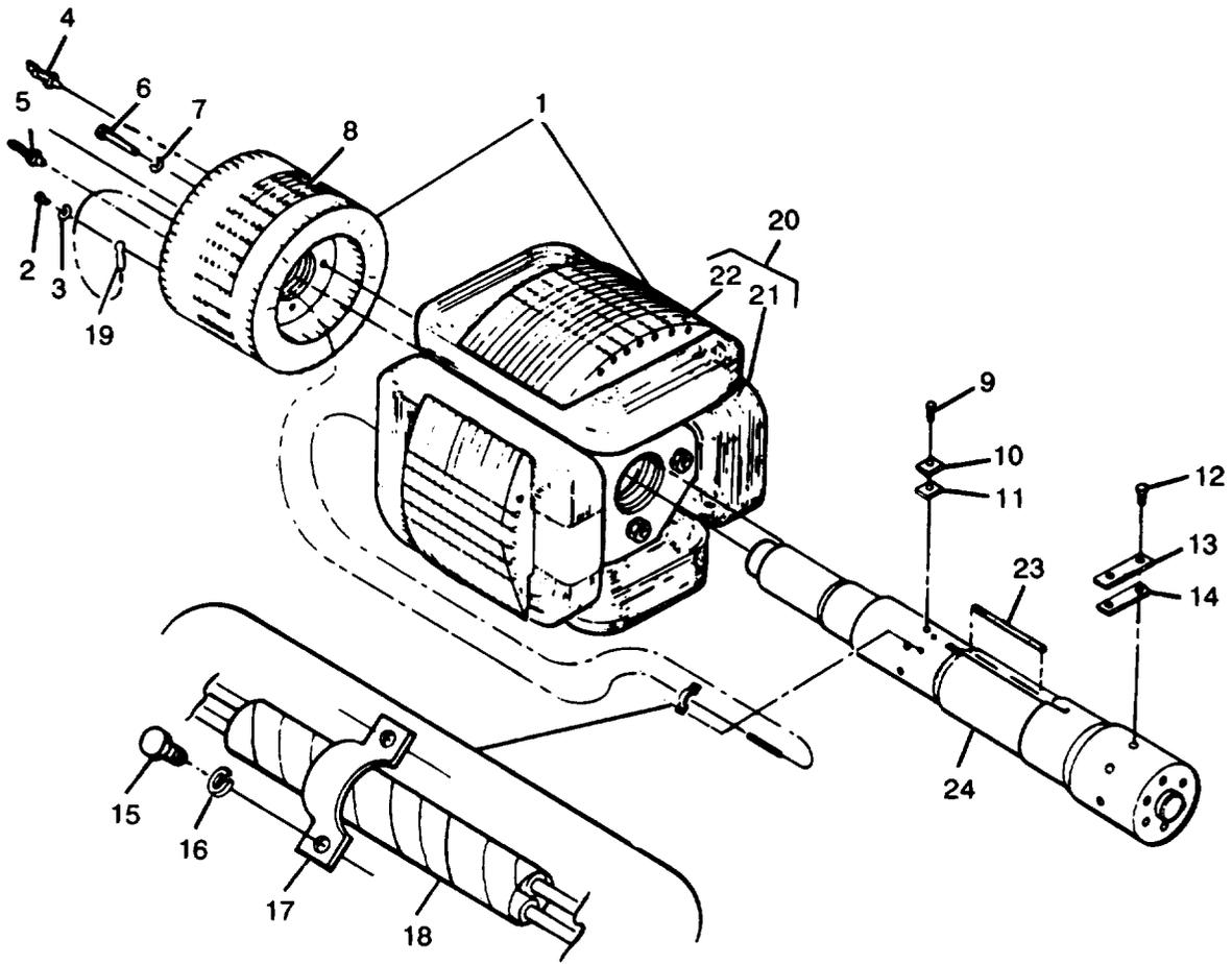
Figure 46. 50/60 Hz Rotor Assembly
