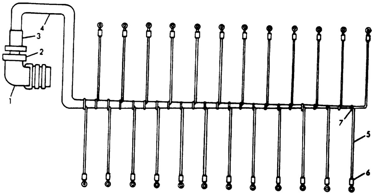
Figure 102. Bottom Load Bank Wiring Harness
