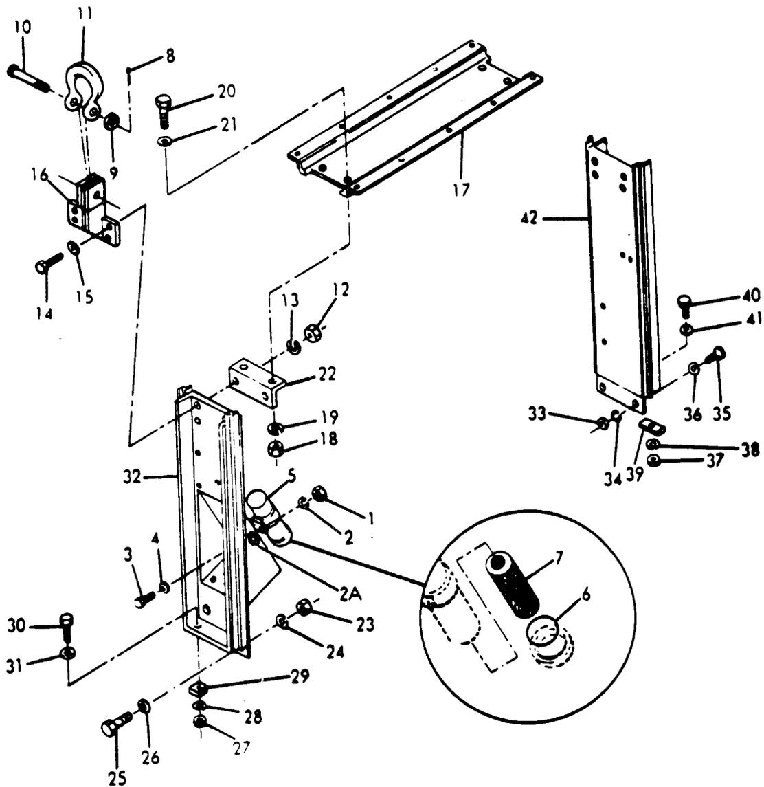
Figure 51. Center Support and Fuel Pumps
