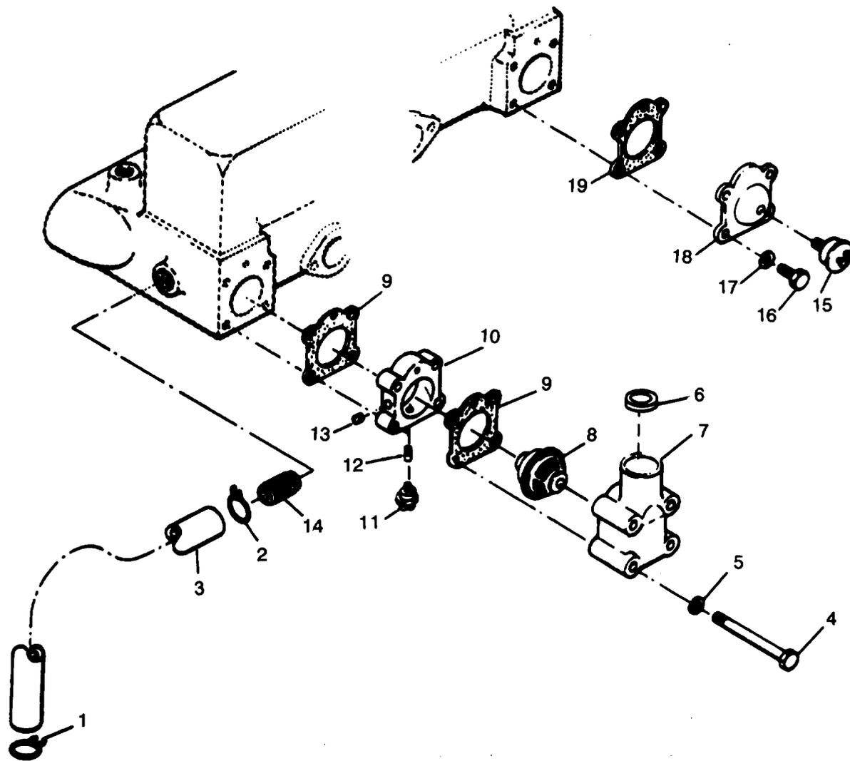
Figure 74. Coolant Thermostat and Sensors
