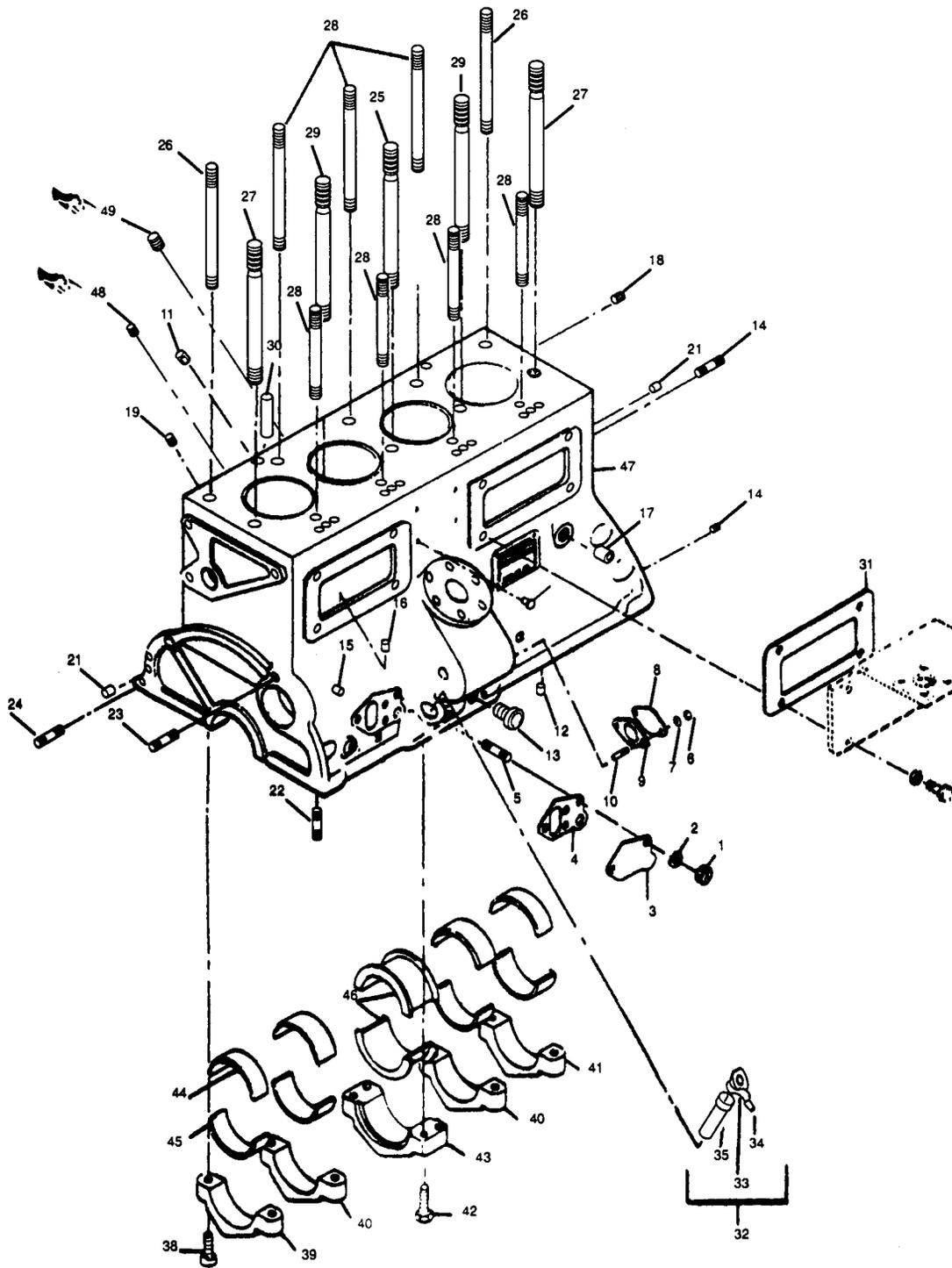
Figure 82. Cylinder Block Assembly
