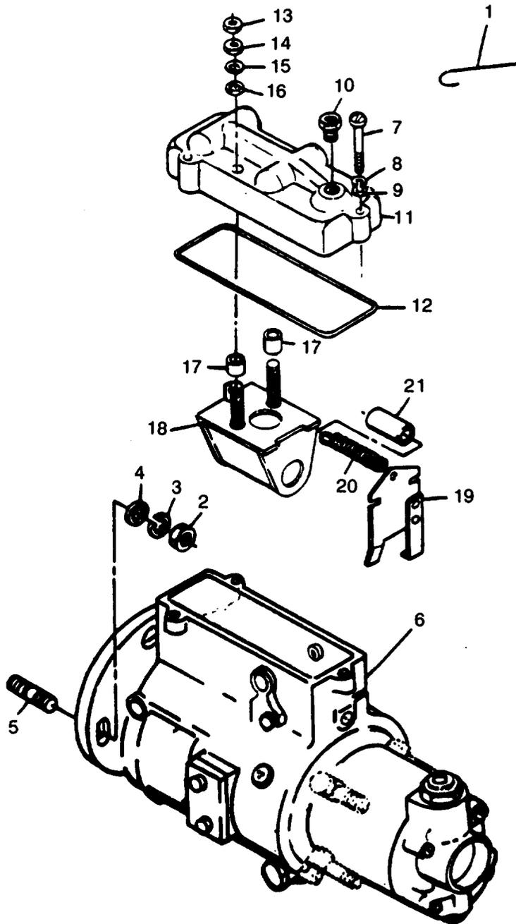
Figure 66. Fuel Injection Pump
