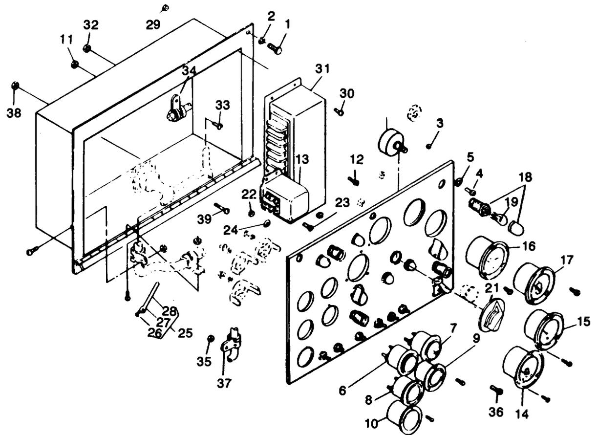
Figure 8. Control Cubicle Assembly and Manual Speed Control (Sheet 1 of 2)
