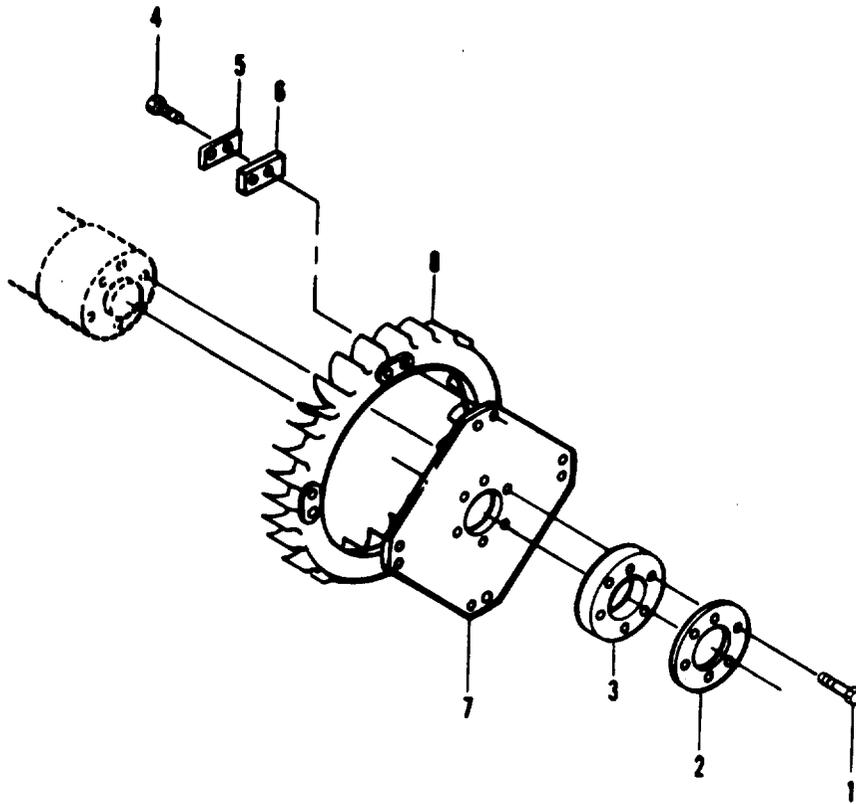
Figure 40. Blower and Coupling Disc
