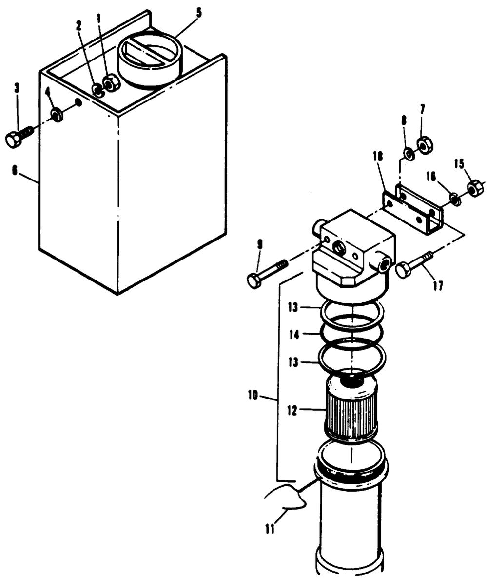
Figure 56. Hydraulic Sump and Filter
