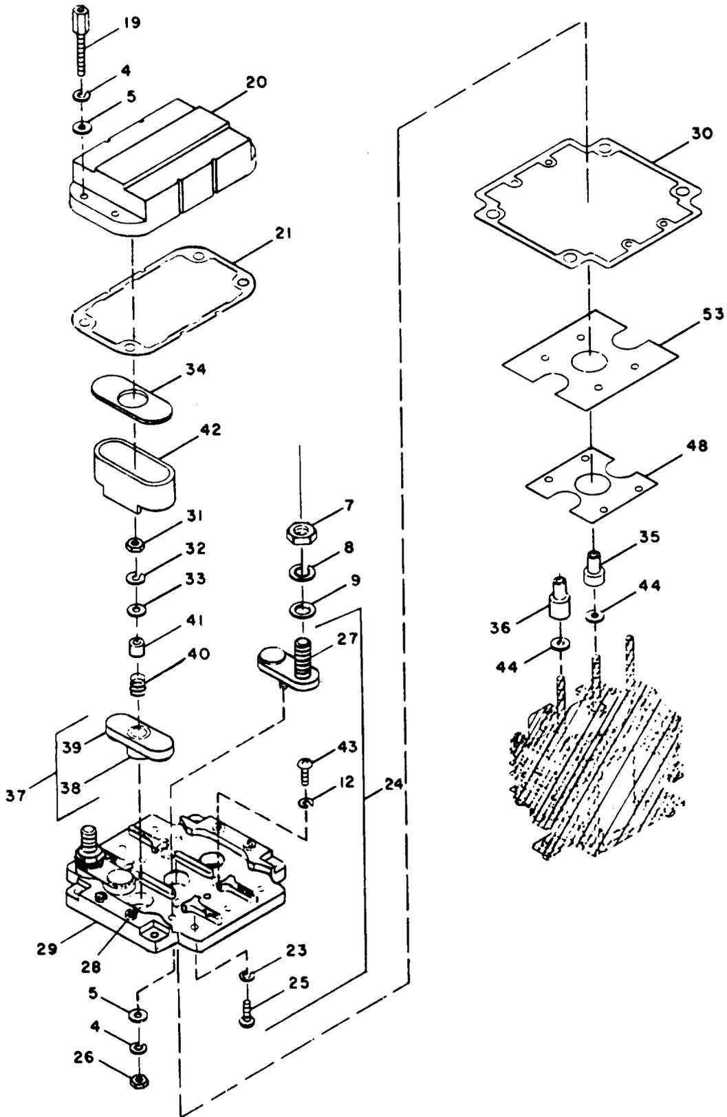
Figure 19. Main Load Contactor (Sheet 2 of 3)
