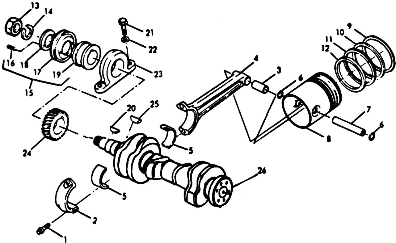
Figure 80. Piston, Connecting Rod, Crankshaft, Pulley, and Front Support
