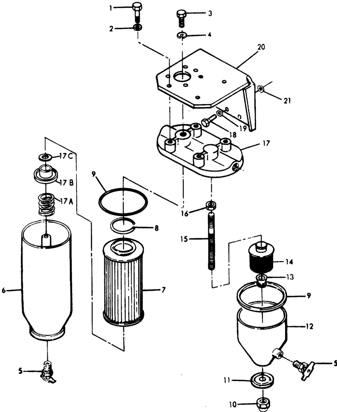
Figure 49. Primary Fuel Filter and Strainer
