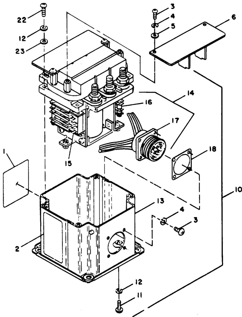
Figure 19. Main Load Contactor (Sheet 1 of 3)
