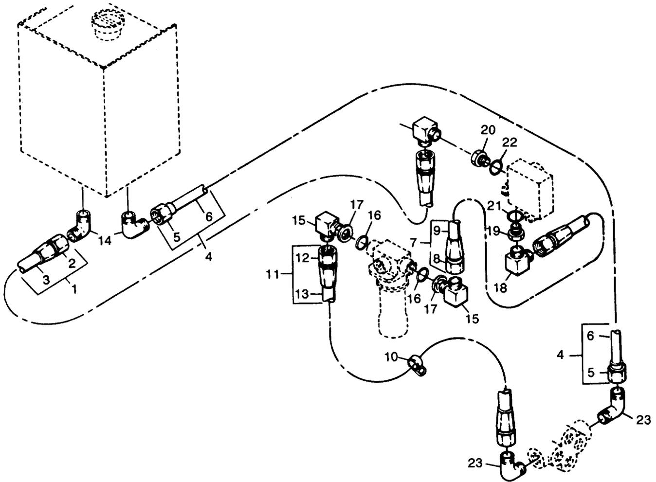
Figure 55. Hydraulic Lines and Fittings
