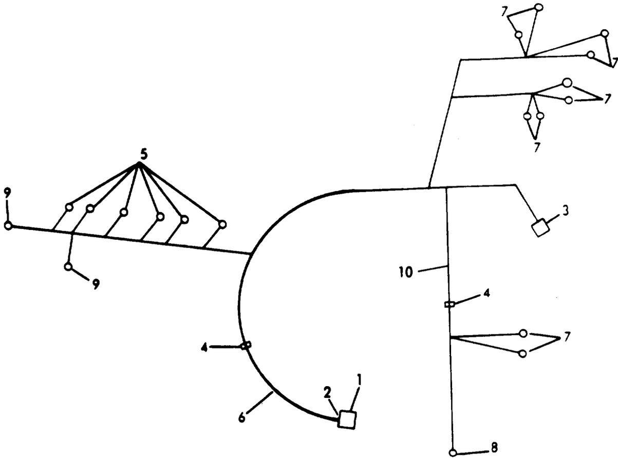
Figure 10. AC Power Control Wiring Harness
