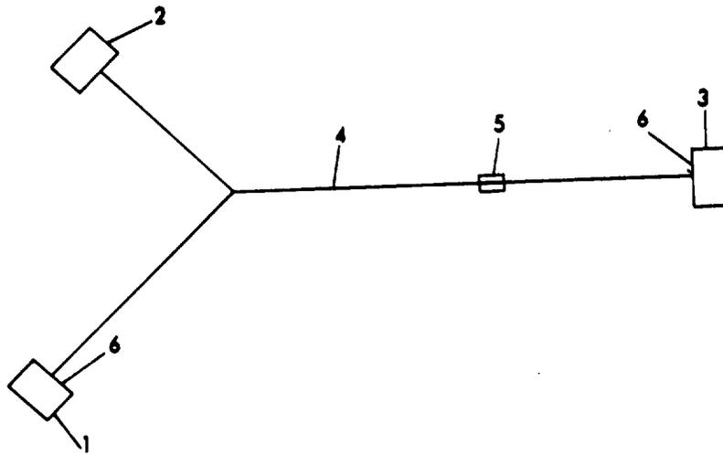
Figure 33. Precise Relay to Governor Control Unit Wiring Harness
