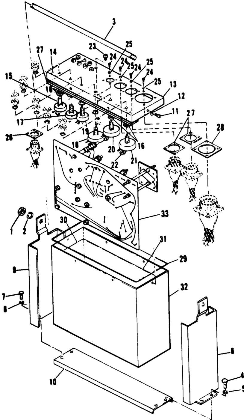
Figure 22. Governor Control Unit (Sheet 1 of 3)
