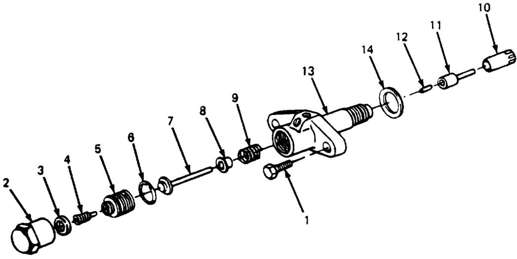
Figure 65. Fuel Injector Assembly
