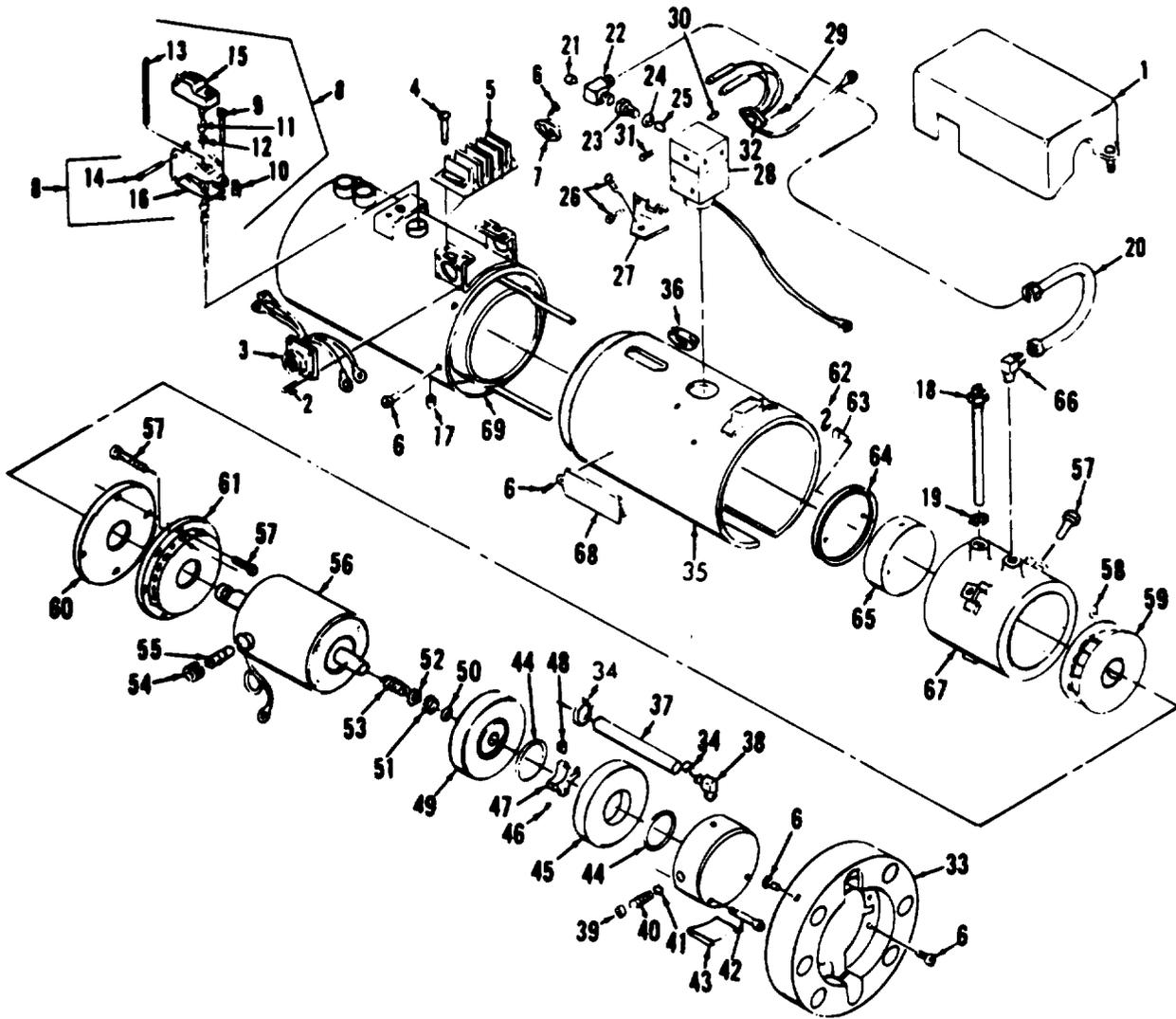
Figure 89. Engine Heater
