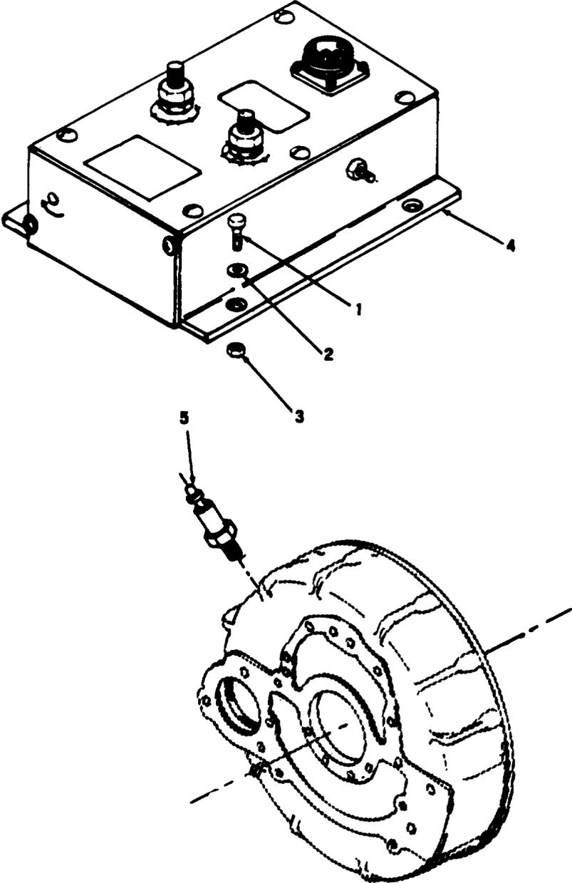
Figure 23. Governor Control Unit and Magnetic Pickup
