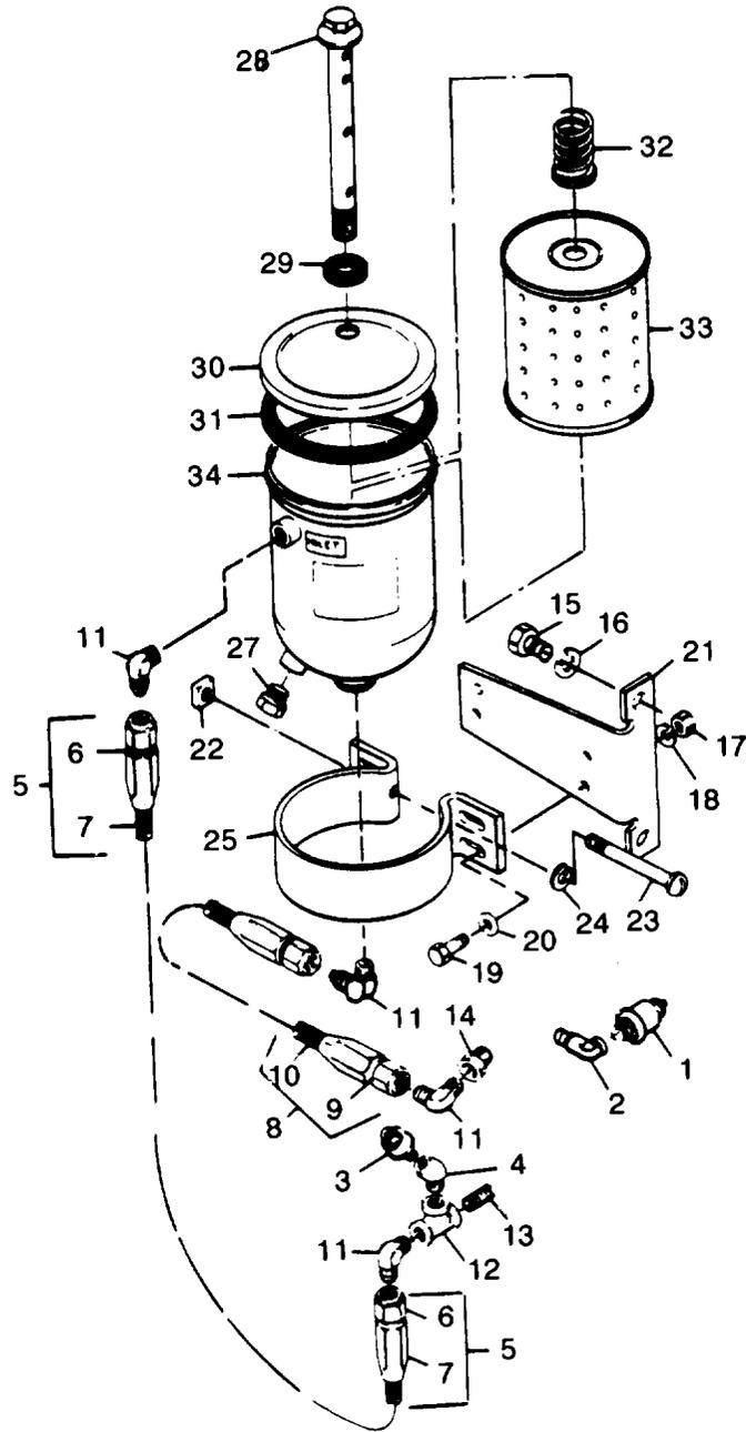
Figure 61. Oil Filter, Sensors, Hose and Fittings
