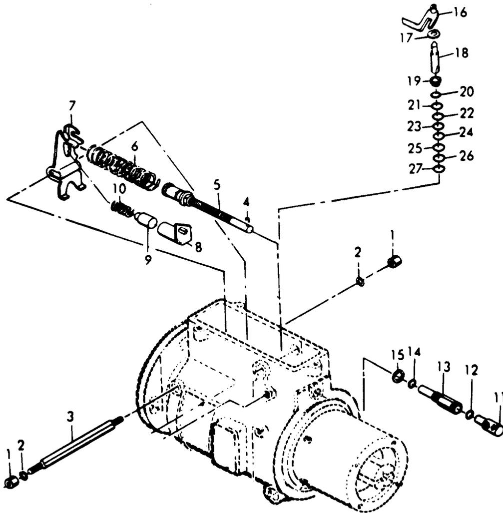
Figure 69. Fuel Injection Pump, Pivot Shaft and Arm Assembly
