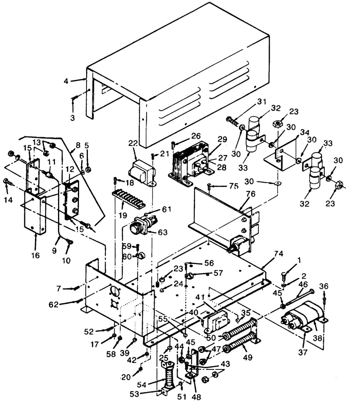
Figure 34. Static Exciter and Voltage Regulator (Sheet 1 of 4)
