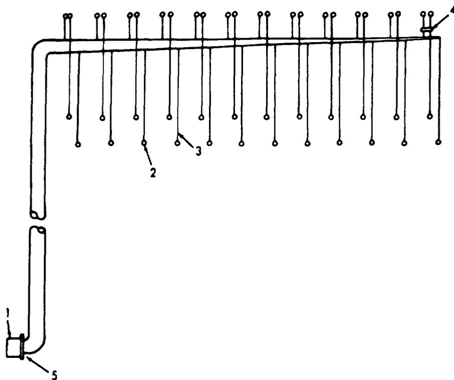
Figure 104. Top Load Bank Wiring Harness
