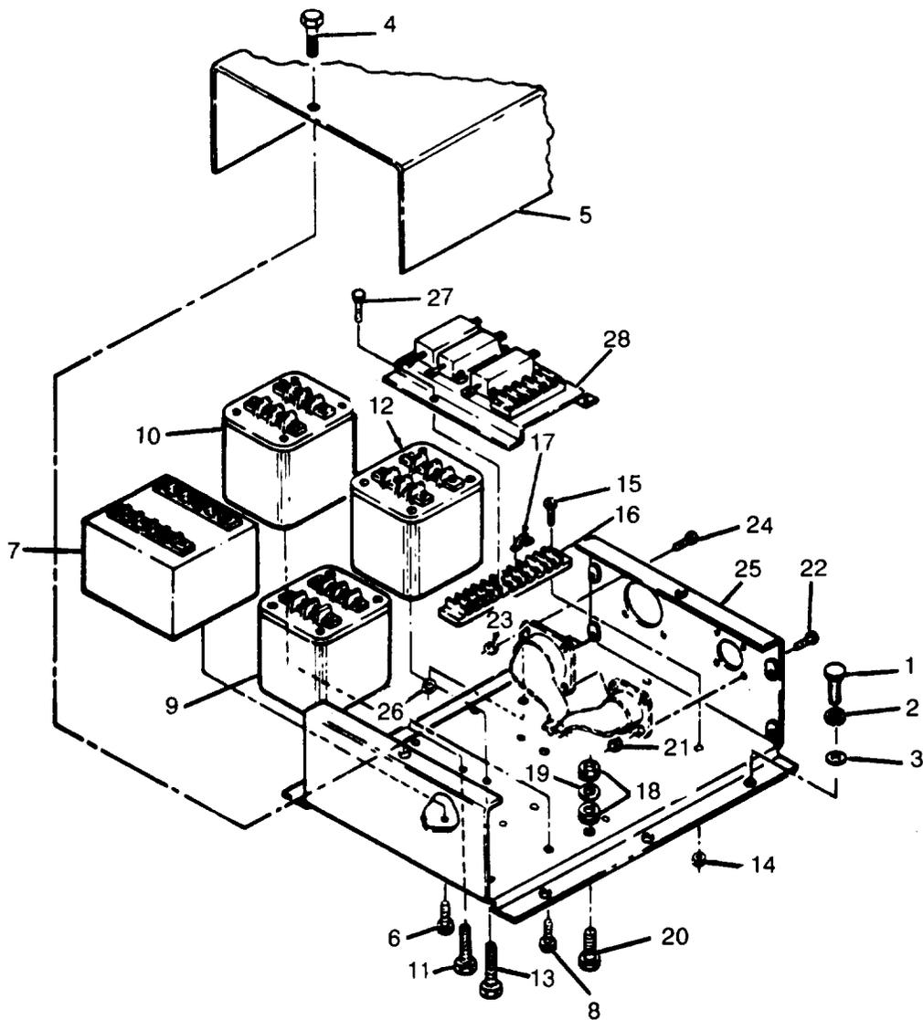
Figure 26. Tactical Relay (Sheet 1 of 3)
