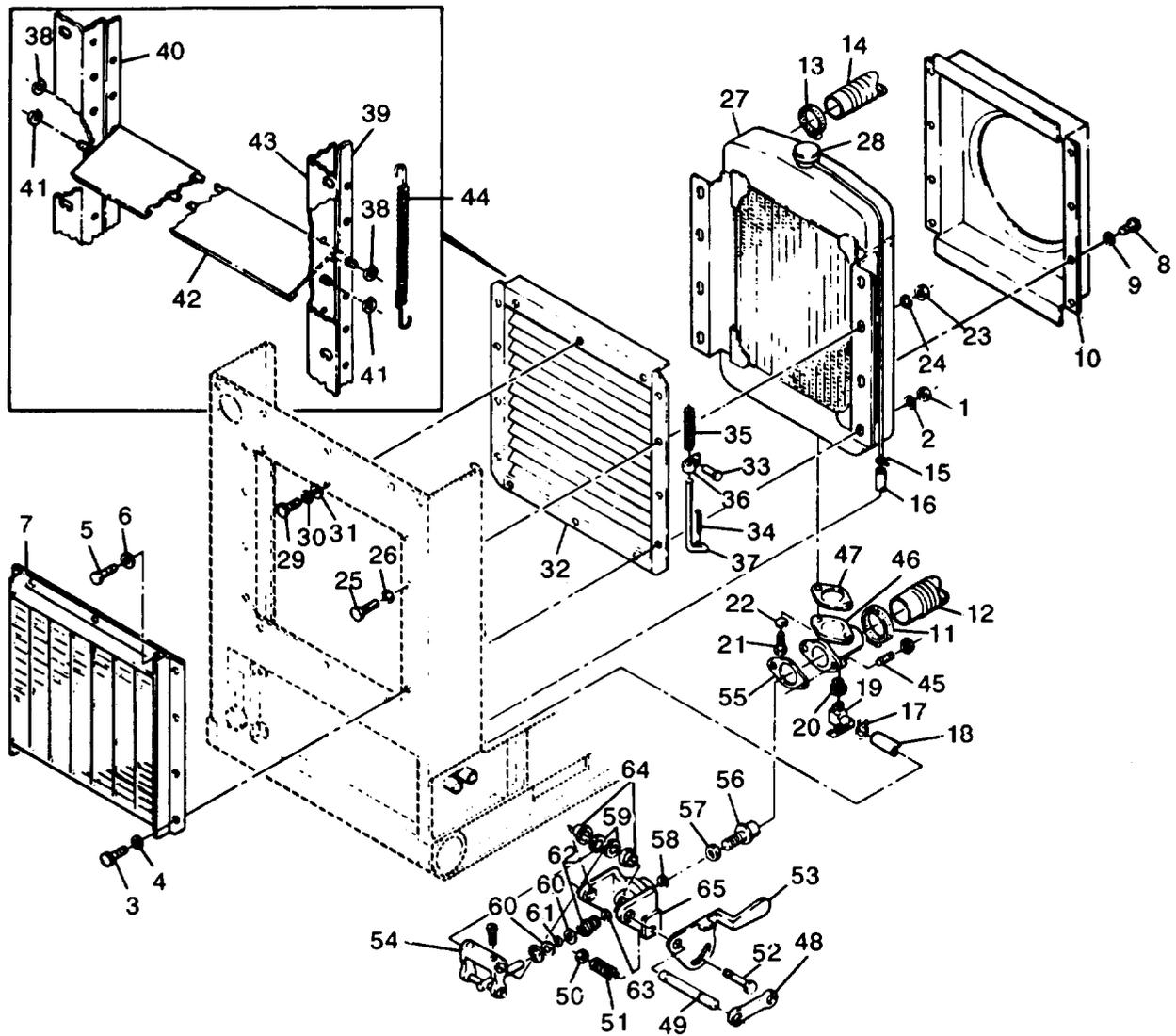
Figure 52. Radiator and Shutter Assembly
