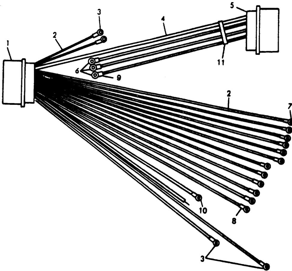
Figure 101. Control Box Wiring Harness
