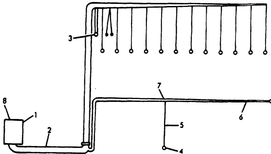
Figure 103. Load Bank Wiring Harness
