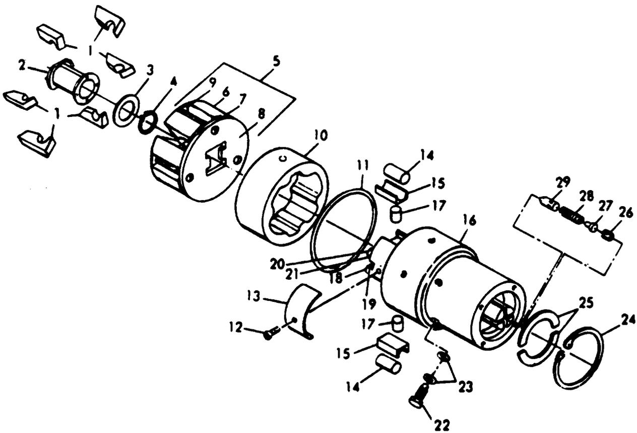
Figure 71. Fuel Injection Pump Rotor Assembly
