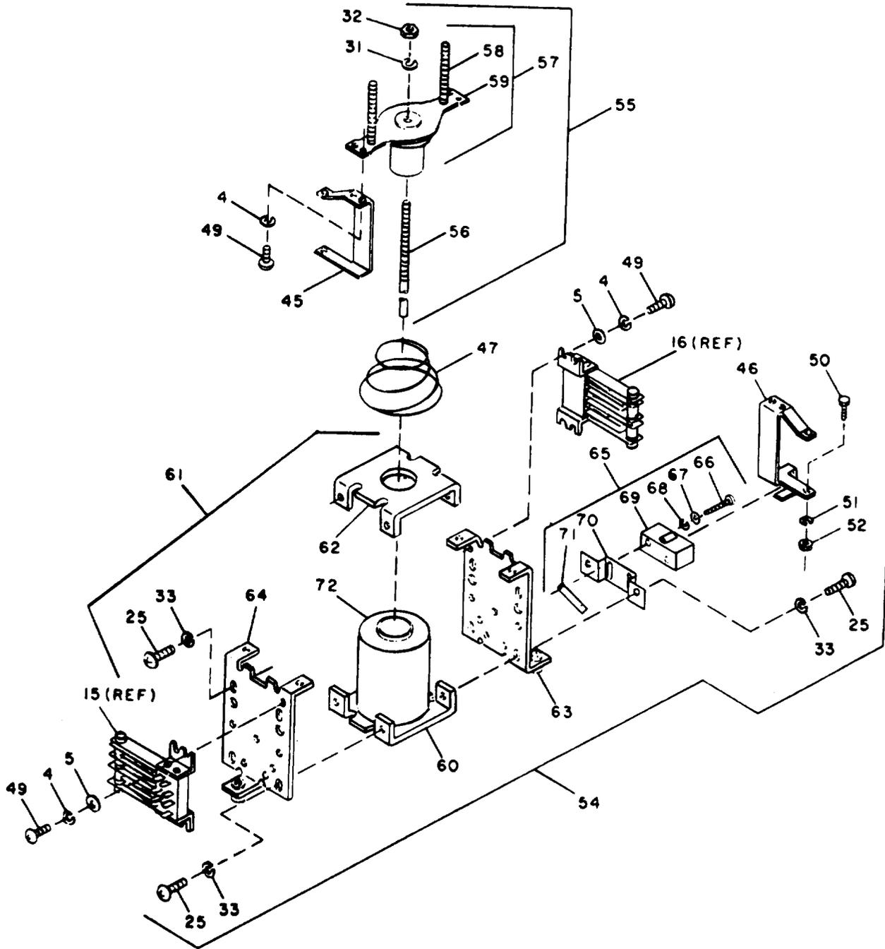
Figure 19. Main Load Contactor (Sheet 3 of 3)
