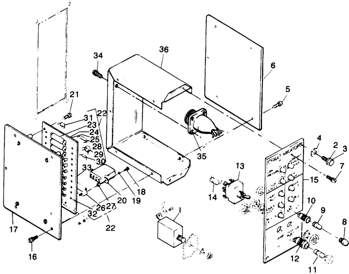
Figure 7. Fault Locating Indicator and DC Circuit Breaker
