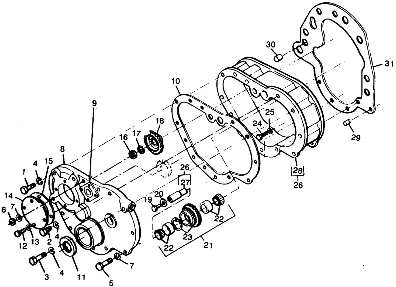
Figure 79. Gear Case and Timing Gears
