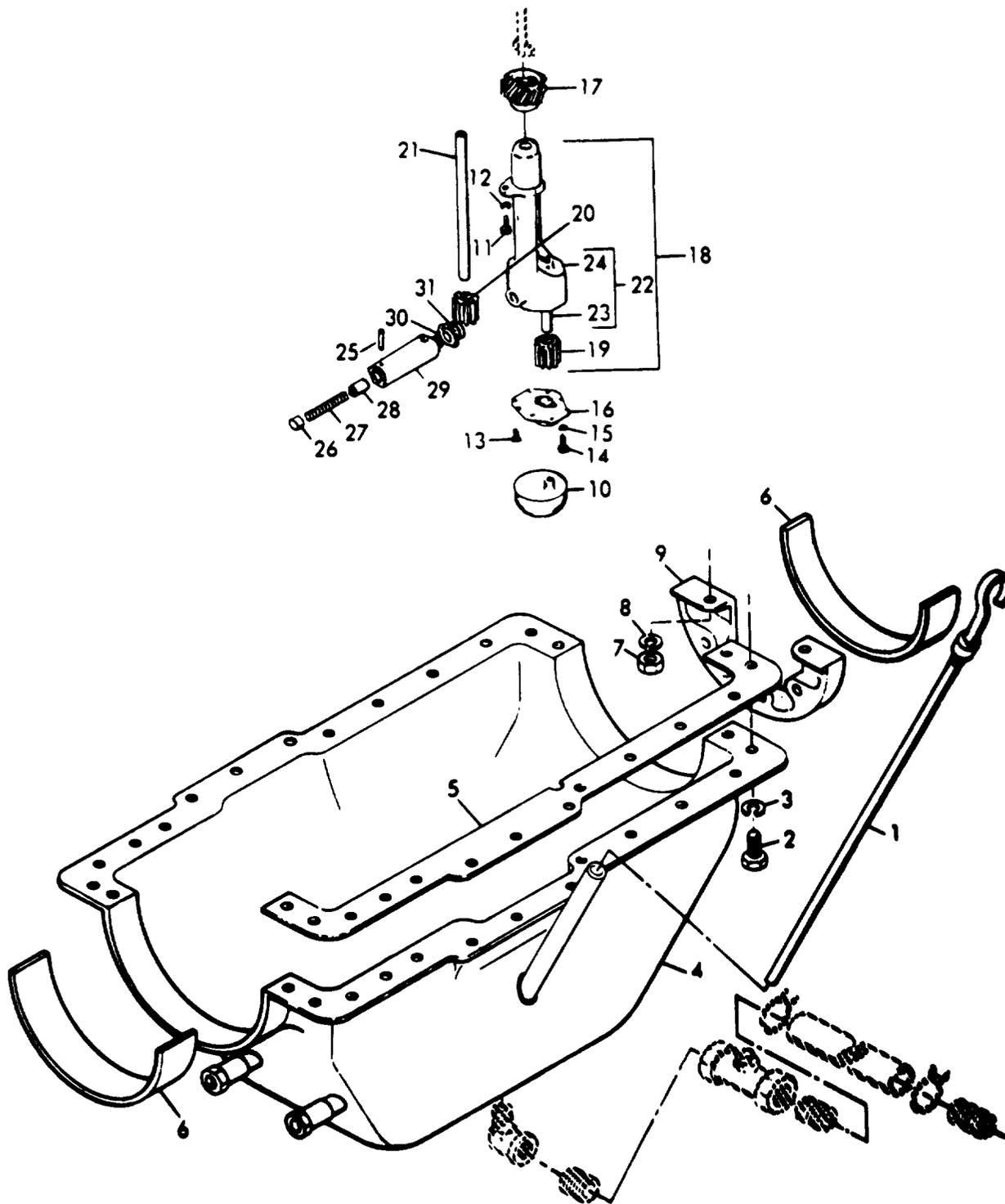
Figure 77. Oil Pan and Oil Pump
