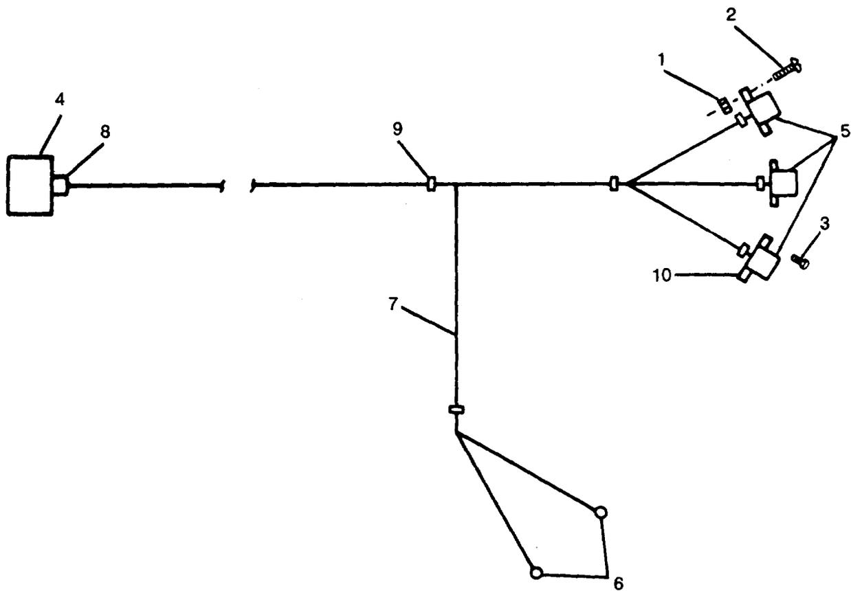
Figure 4. Paralleling and Convenience Receptacles Wiring Harness
