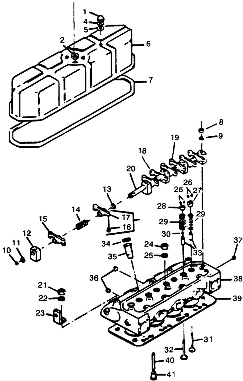
Figure 76. Cylinder Head Cover, Cylinder Head Valve Operating Mechanism.
