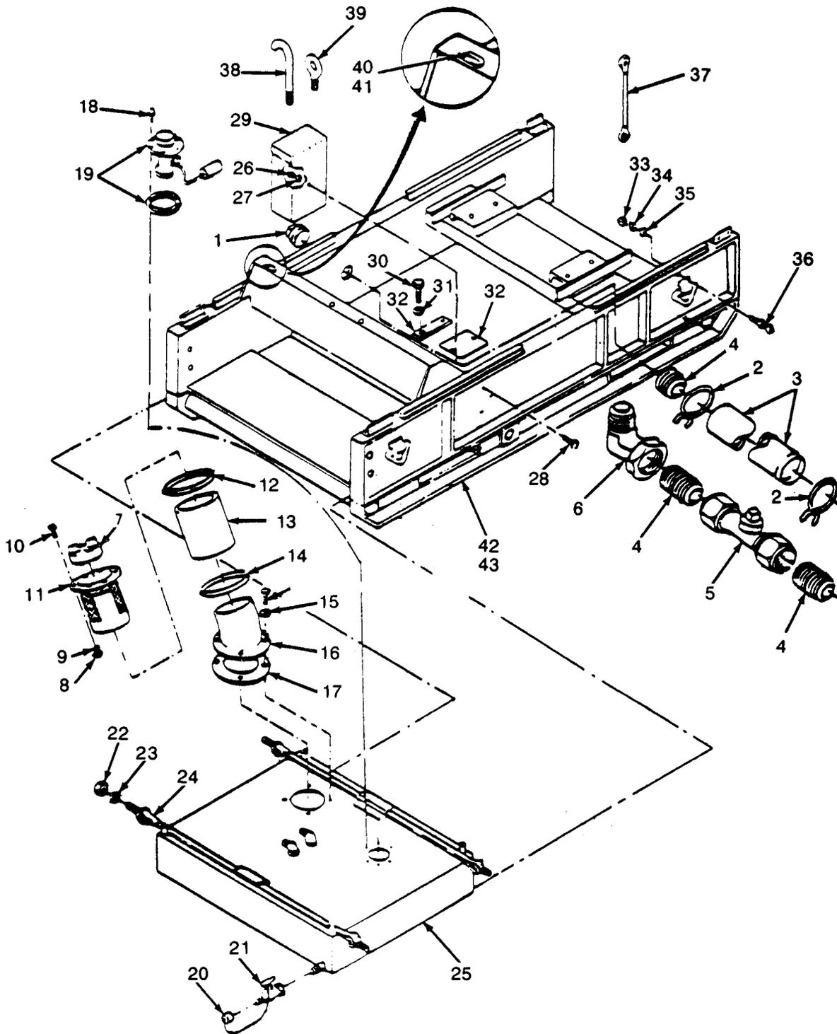
Figure 83. Fuel Tank, Skid Base and Oil Drain
