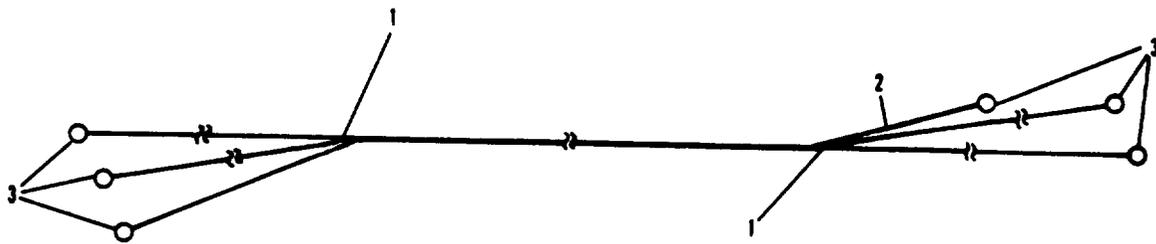
Figure 20. Reconnection Board to Contactor Harness
