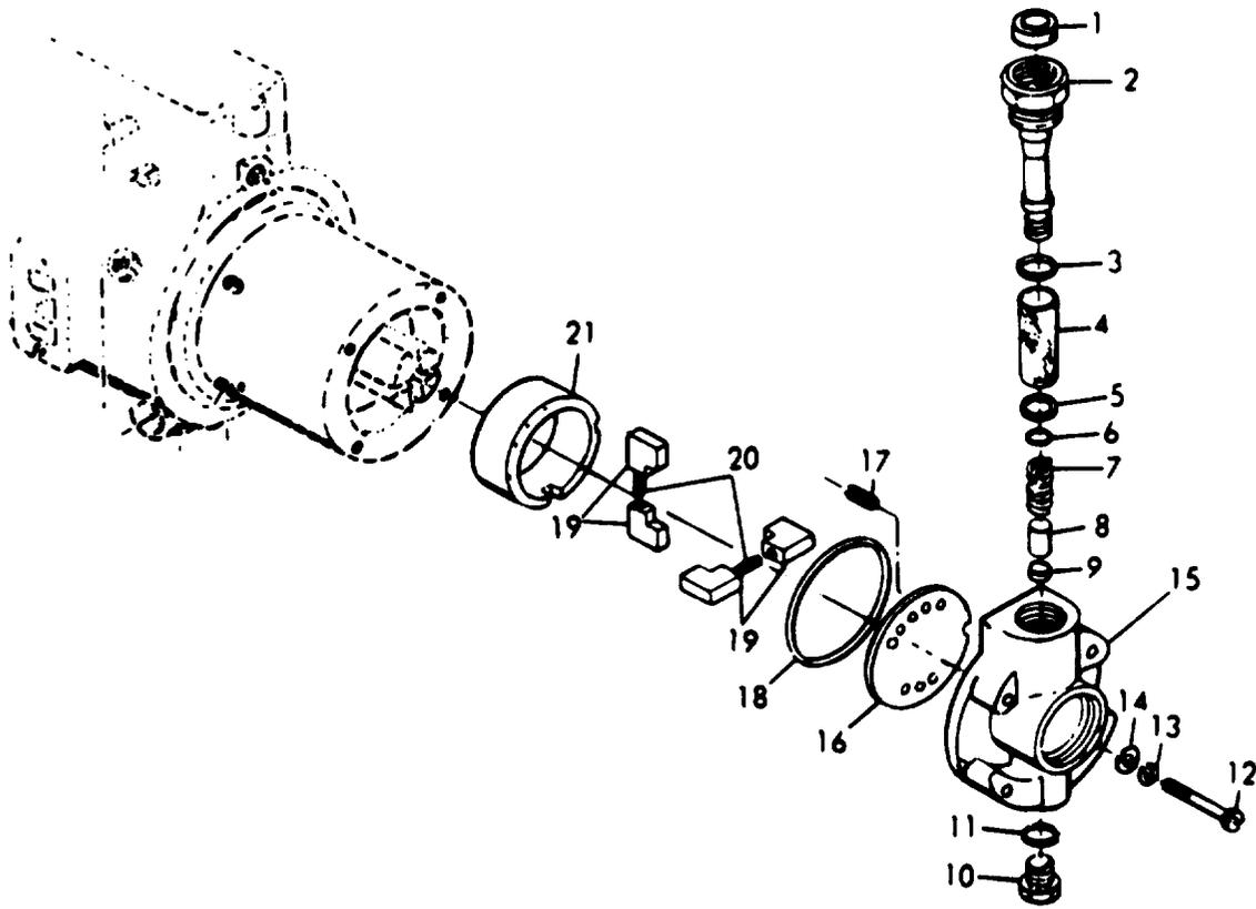
Figure 68. Fuel Injection Pump End Plate and Blades
