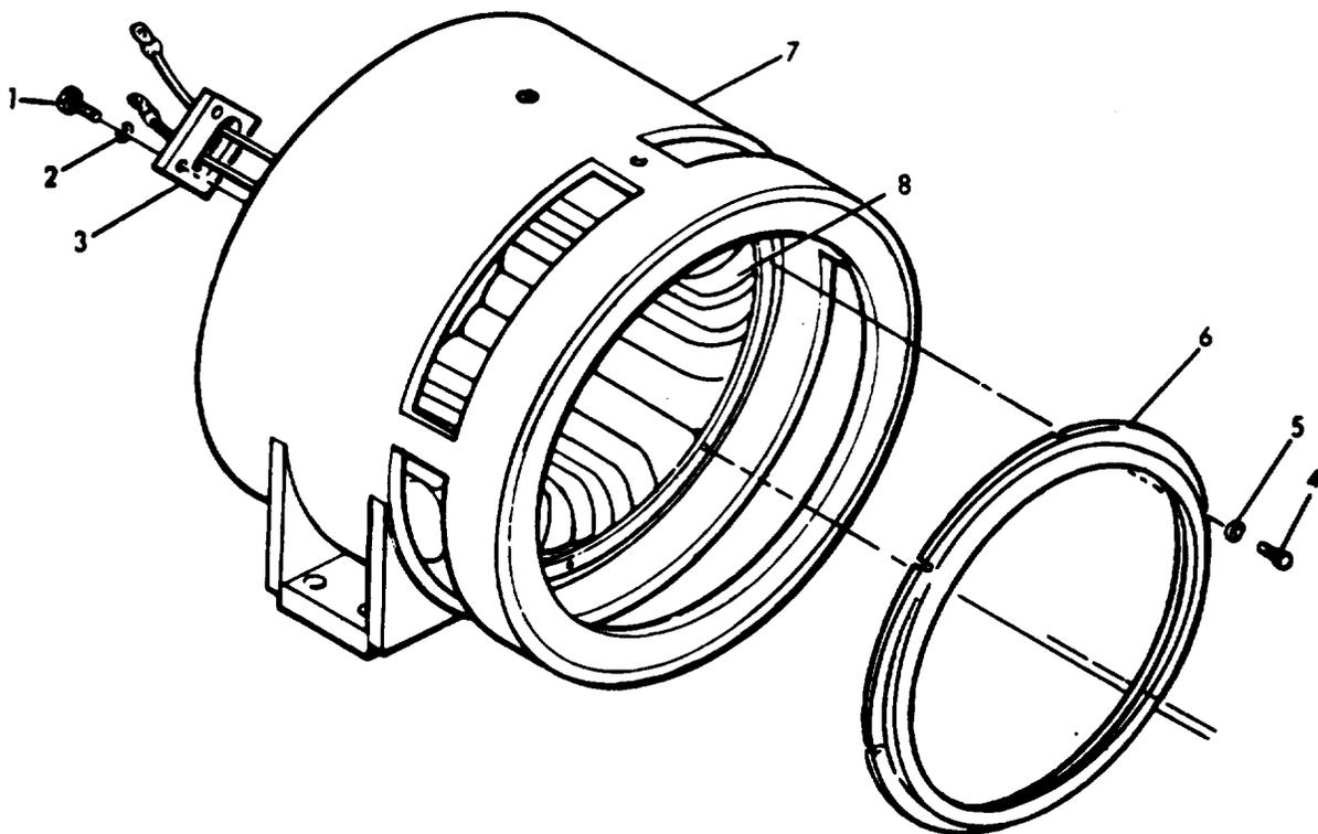
Figure 45.400 Hz Stator Assembly
