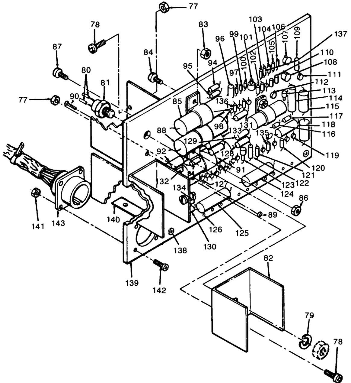
Figure 34. Static Exciter and Voltage Regulator (Sheet 3 of 4)
