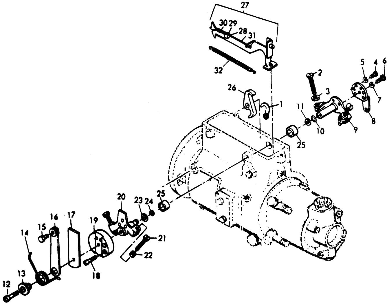
Figure 67. Fuel Injection Pump Linkage
