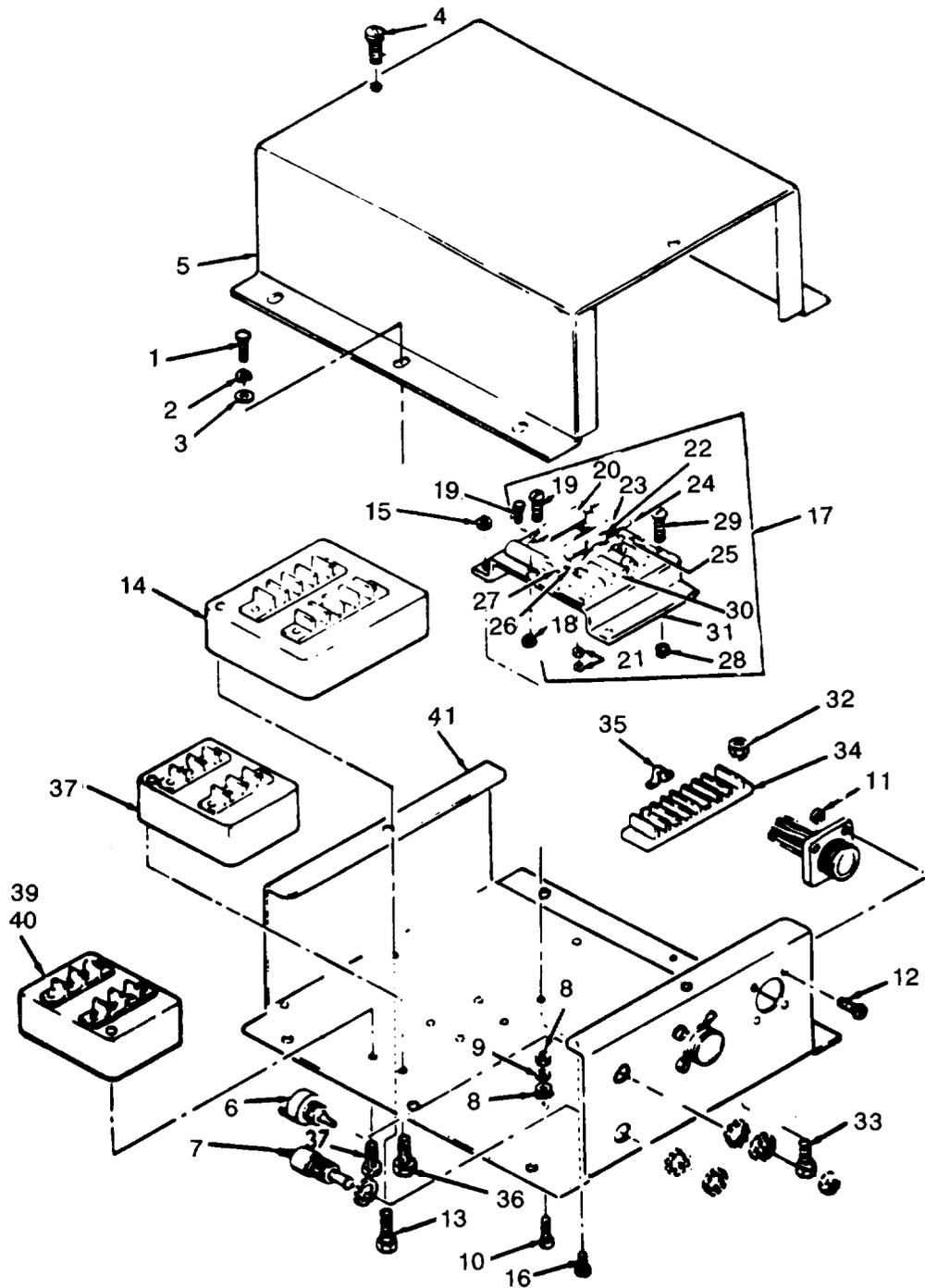
Figure 32. Precise Relay (Sheet 1 of 2)
