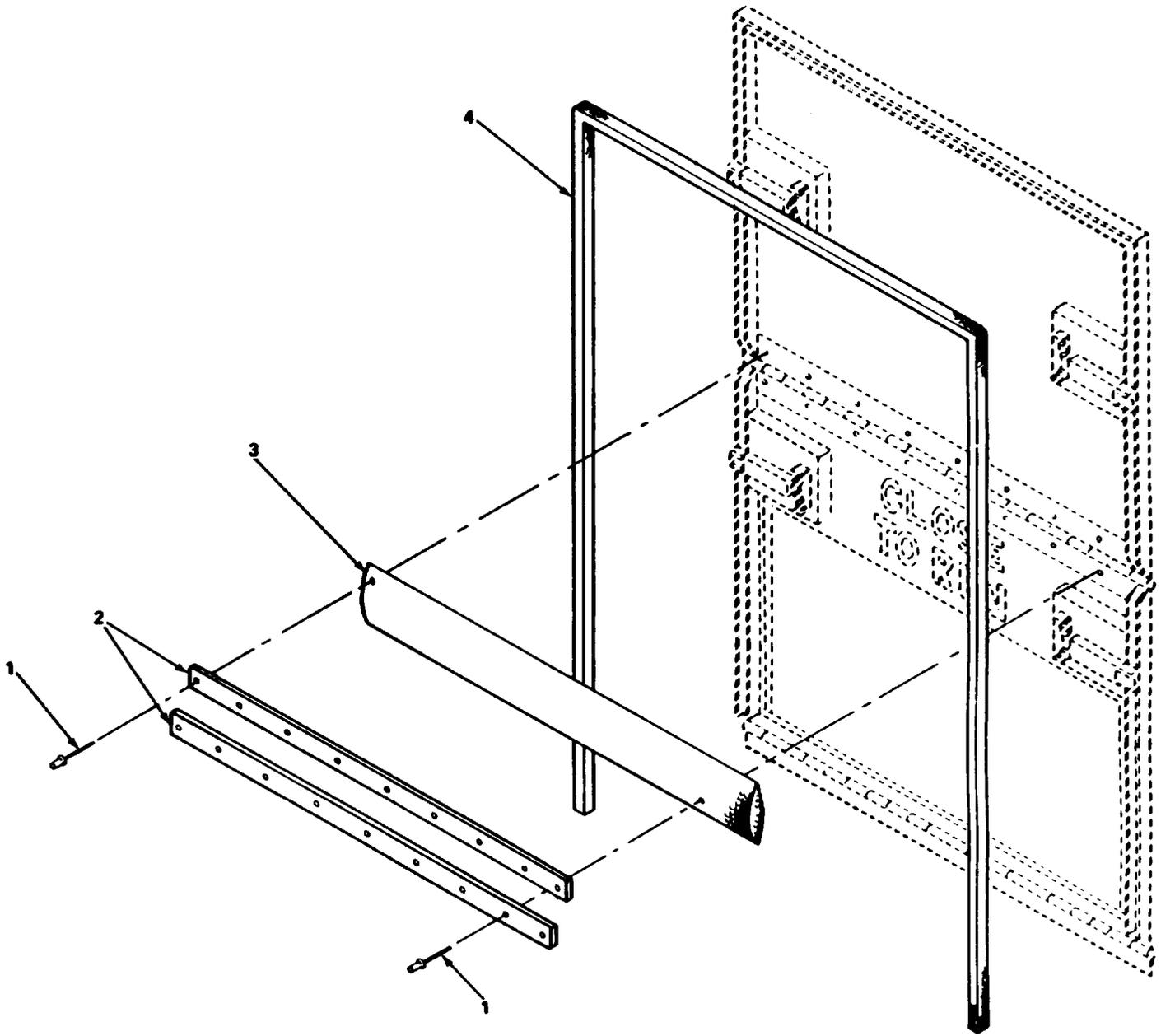
Figure 108. Electromagnetic Shielding
