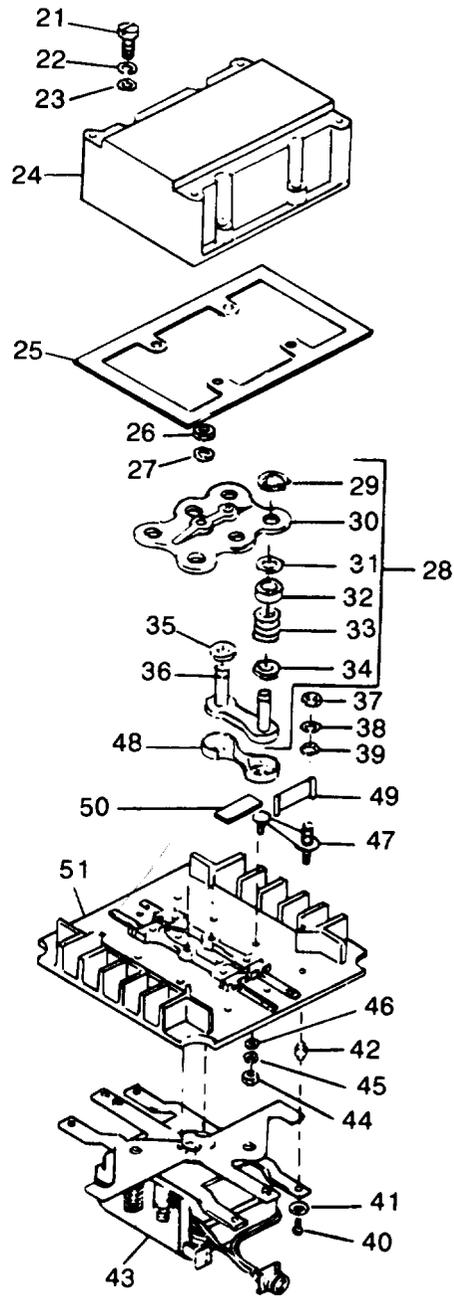
Figure 18. Main Load Contactor (Sheet 2 of 4)
