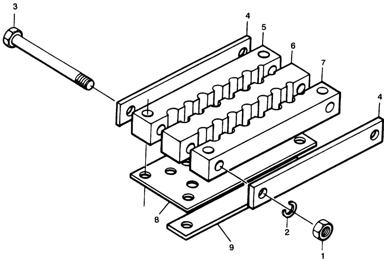
Figure 42. Lead Block Assembly
