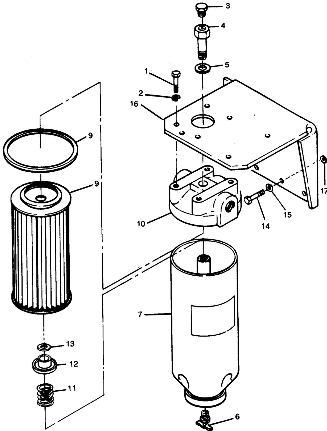
Figure 50. Secondary Fuel Filter
