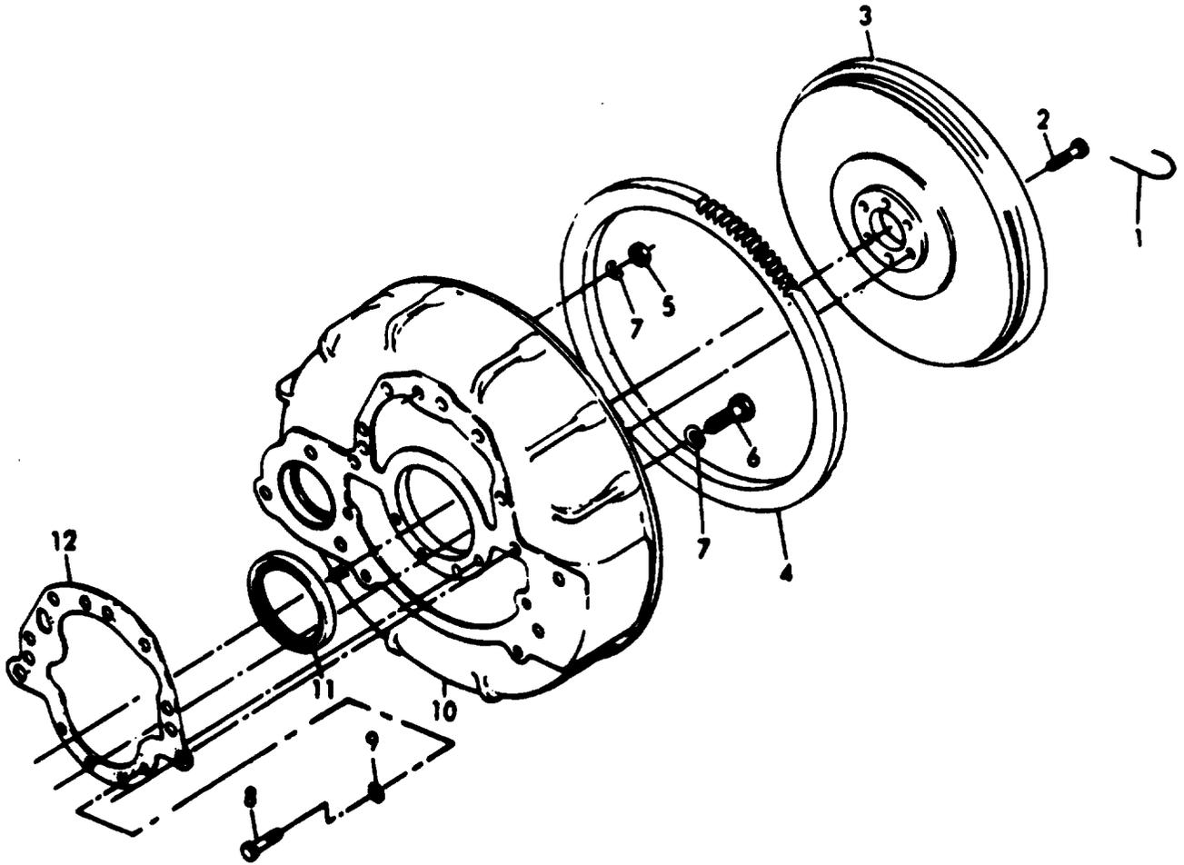
Figure 78. Flywheel, Ring Gear and Housing
