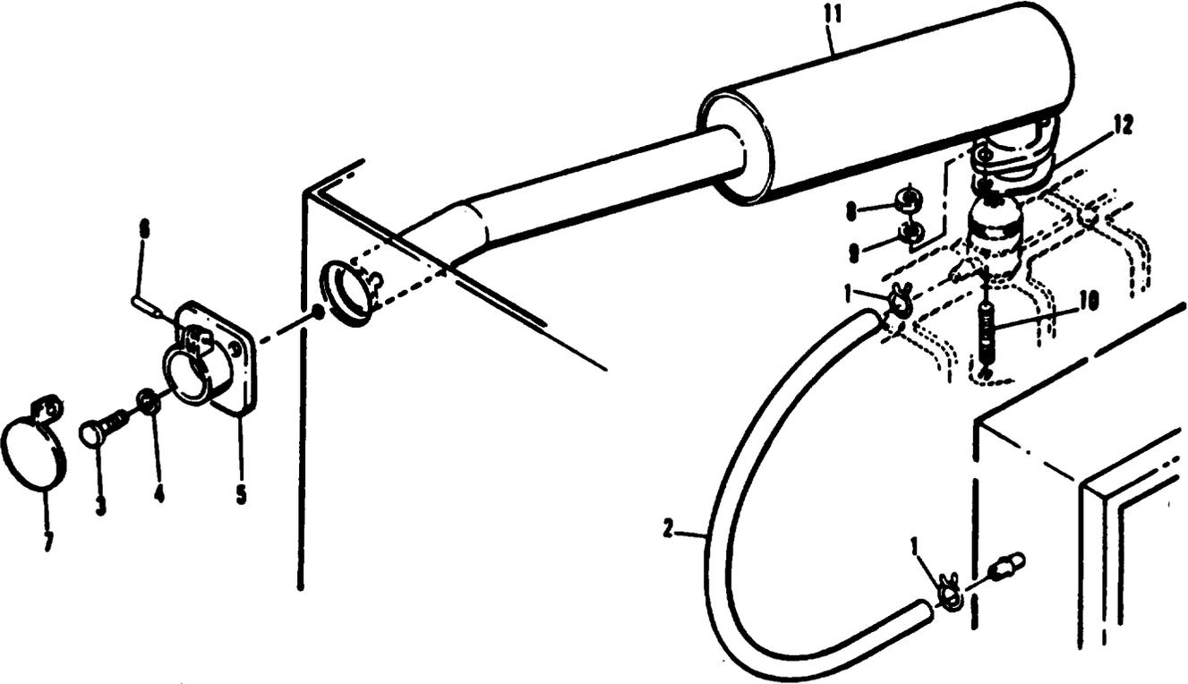
Figure 2. Exhaust Pipe, Muffler and Breather Tube
