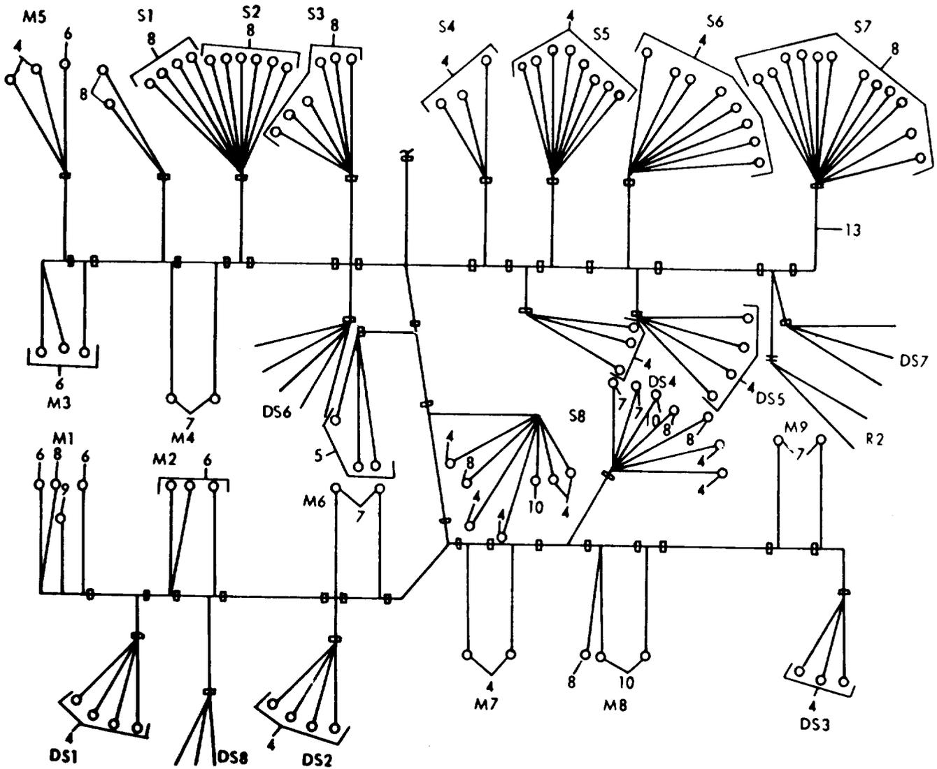
Figure 9. Control Cubicle Branched Wiring Harness (Sheet 2 of 2)
