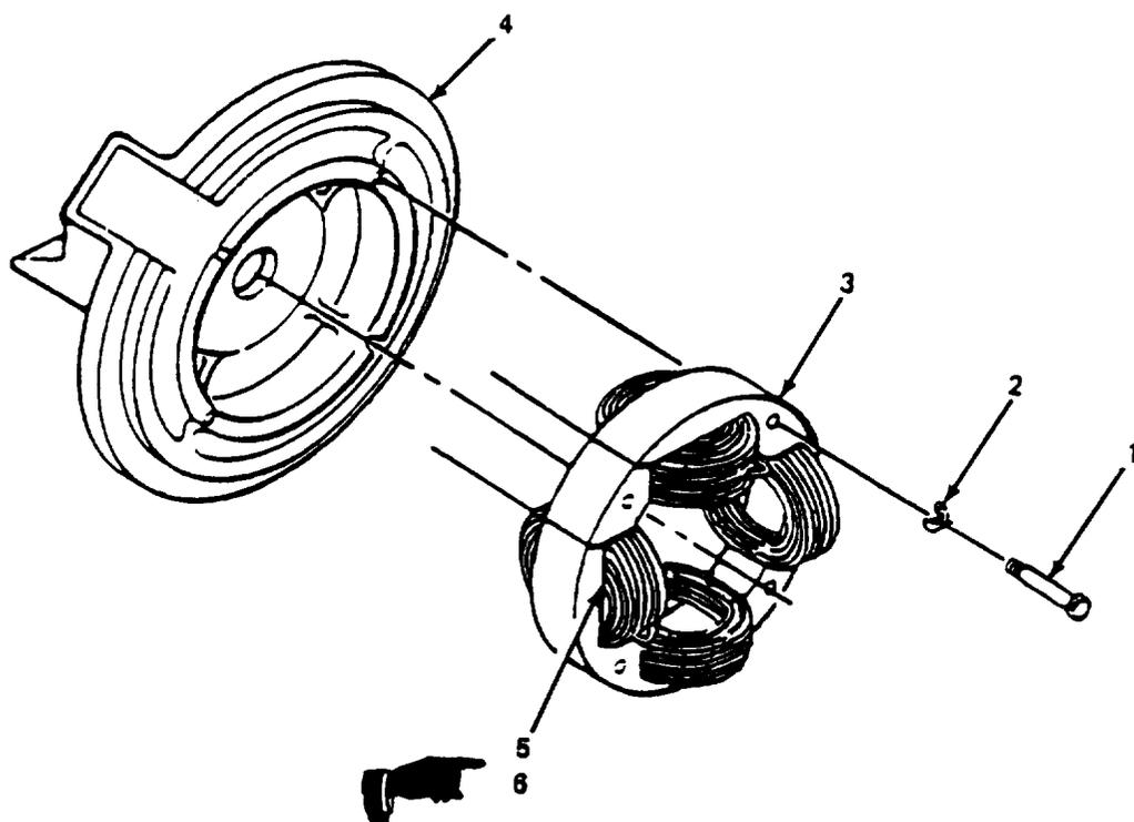
Figure 43. Bracket Assembly
