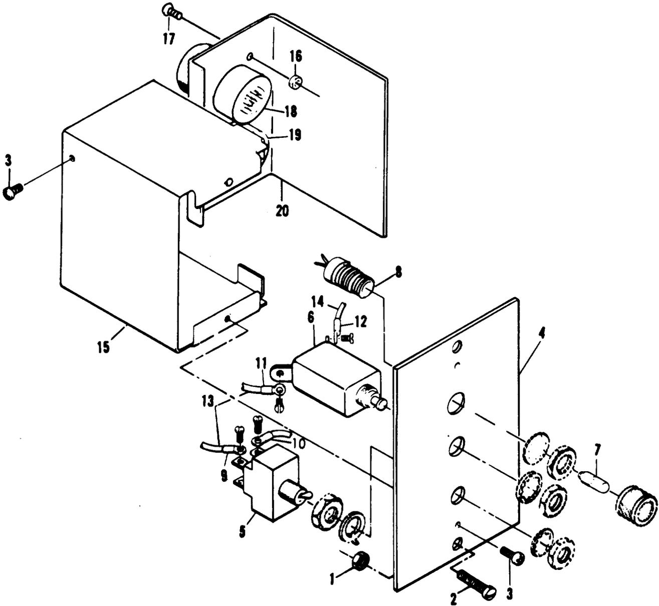
Figure 88. Engine Heater Control Box
