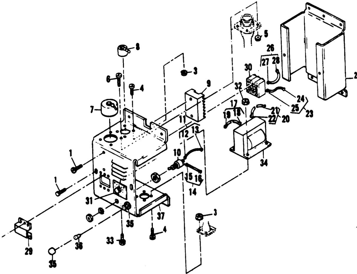
Figure 98. Load Bank Control Box
