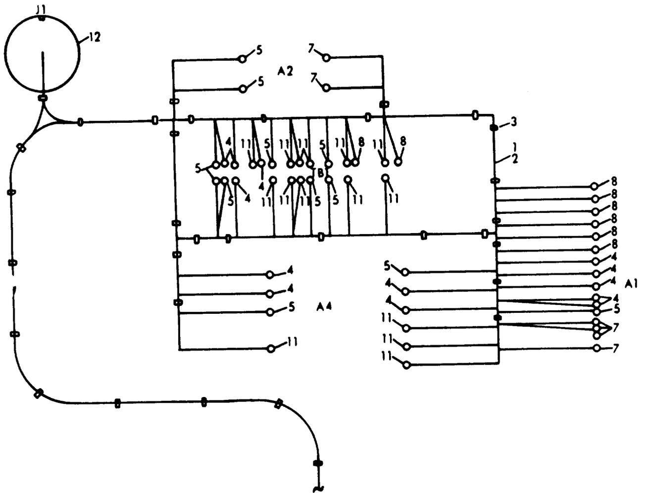
Figure 9. Control Cubicle Branched Wiring Harness (Sheet 1 of 2)
