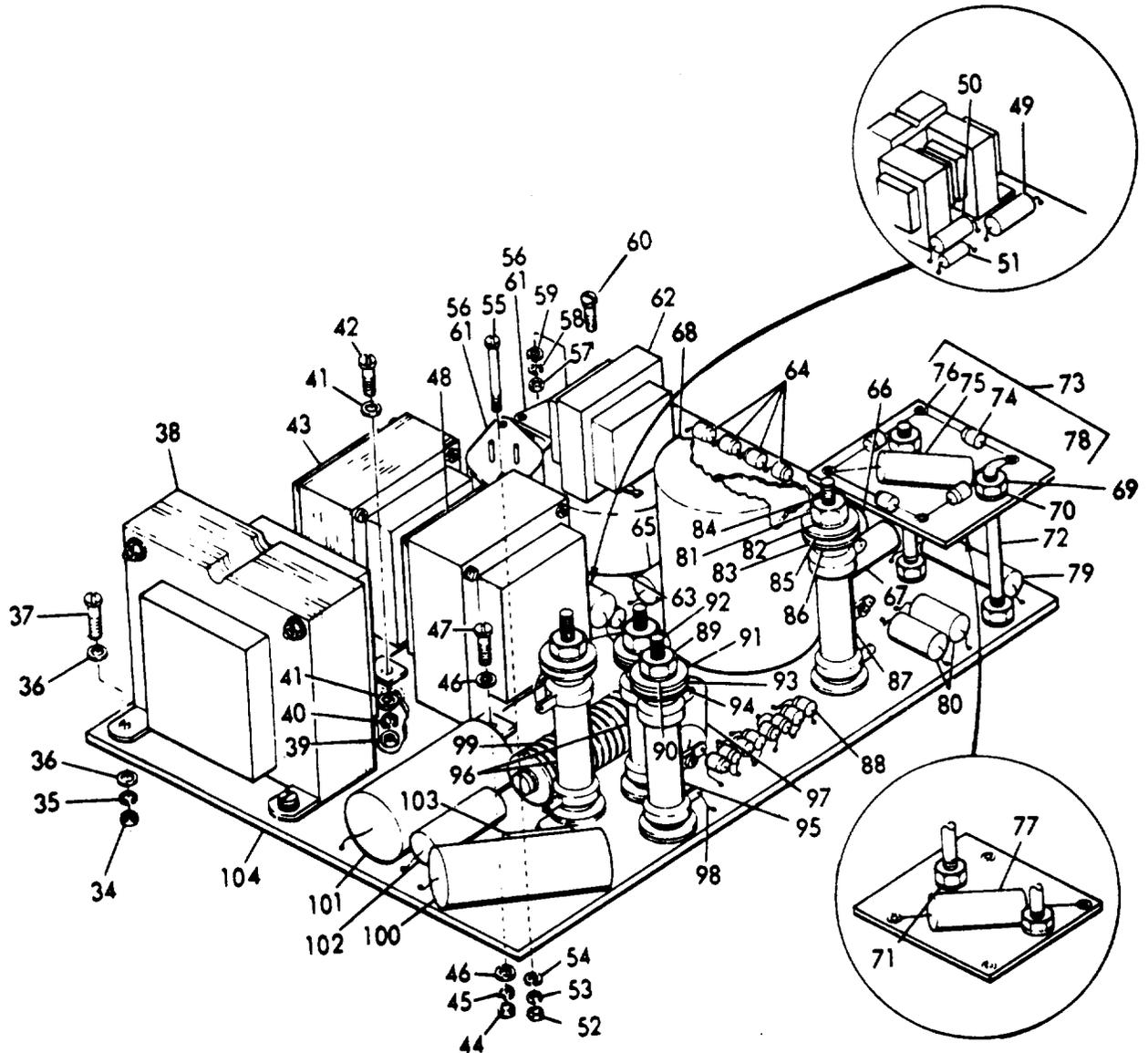
Figure 22. Governor Control Unit (Sheet 2 of 3)
