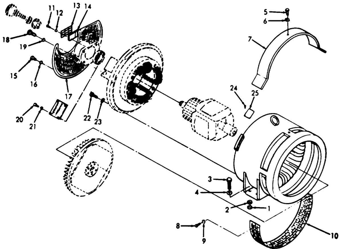
Figure 39. Generator Assembly
