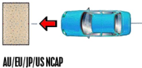
Figure 1. Scenario for the full-frontal impact test.
