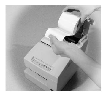
5. Be sure to note the correct direction that the paper should come off the roll.
