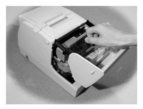
5. Turn the knob two or three times to make sure the ribbon is seated correctly. You can also look at the side of the slip unit to see if the ribbon is in the correct place. See below.
