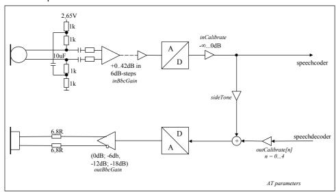
Figure 1: AT audio programming model
