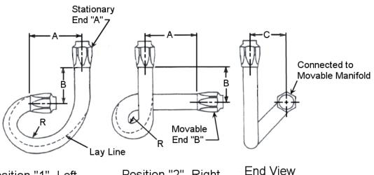
Figure 7. Flex Test Apparatus
