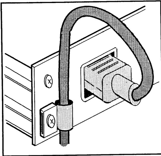
Fig. 4-2. Mount the power cord.
