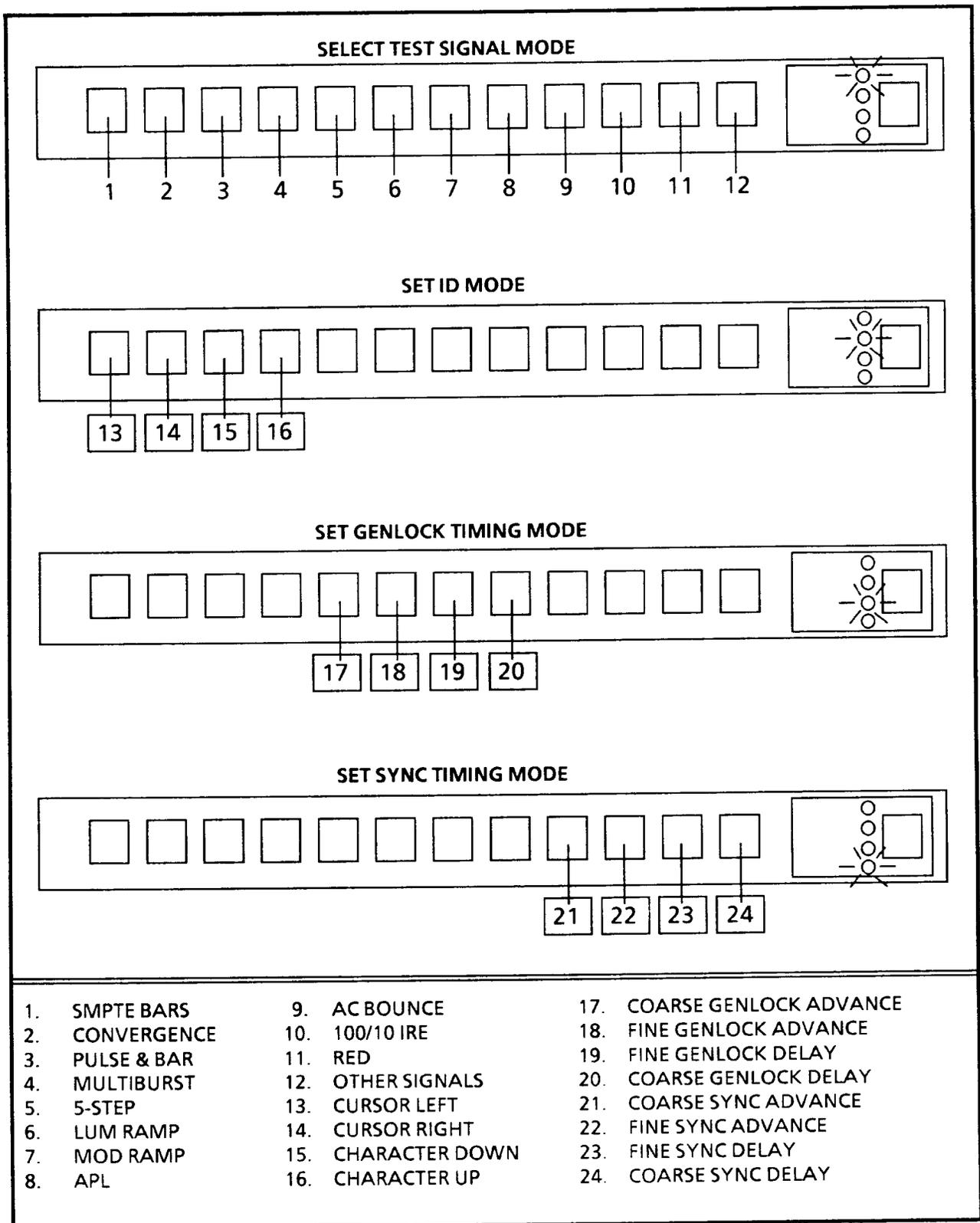
Fig. 2-2. TSG-170A front-panel switch names in the four front-panel modes.
