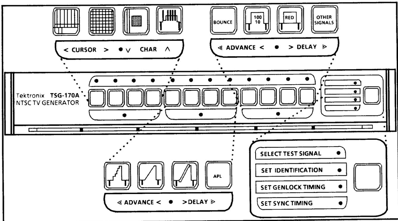
Fig. 2-1. TSG-170A front panel.
