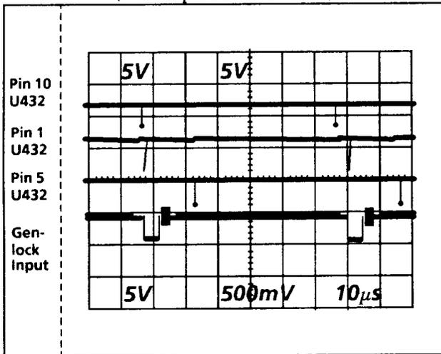
Fig. 7-12. Shows signals through the Genlock Data Acquisition circuit when it is in the UNLOCKED mode.
