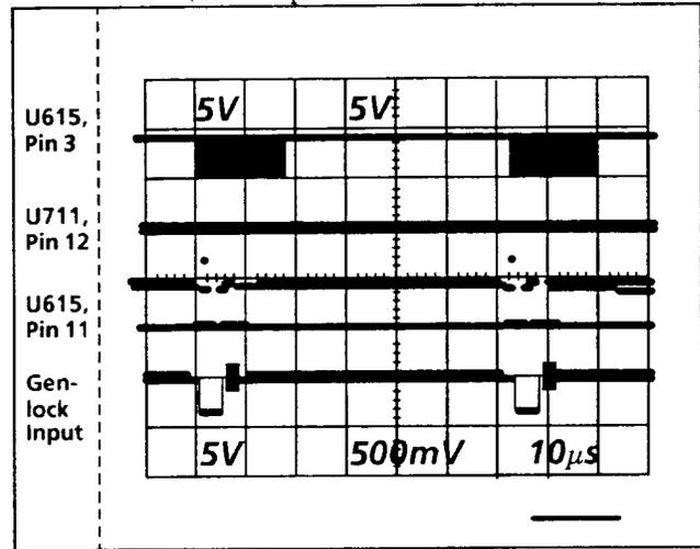
Fig. 7-13. Shows signals through the Genlock Data Acquisition circuit when it is in the UNLOCKED mode.
