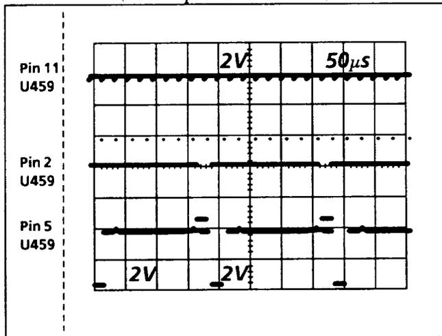
Fig. 7-4. Shows a shifting 0 through the two LSB outputs of the Genlock Offset Port (U459, Schematic 1), as well as the Enable Pulse ( $\overline{\text{GEN DEL SEL}}$ ).
