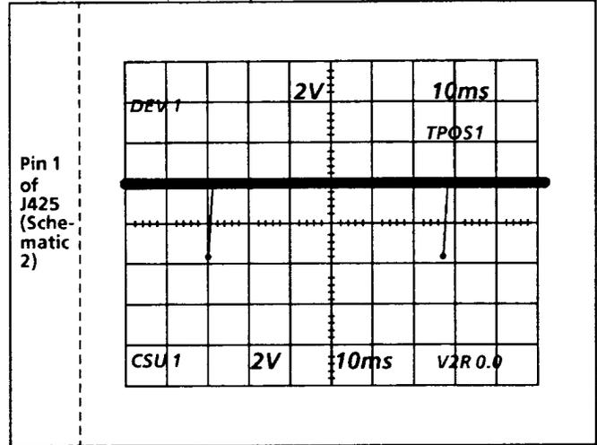
Fig. 7-17. Shows the Hard Reset pulse occurring at a 67 ms rate at the pin 9 output of U222B in the  $\mu P$  kernel.
