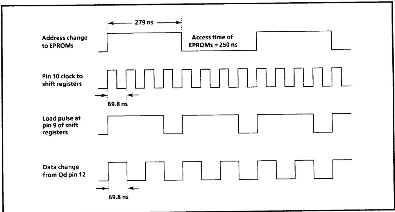
Fig. 6-6. Timing of data-multiplexing shift registers.
