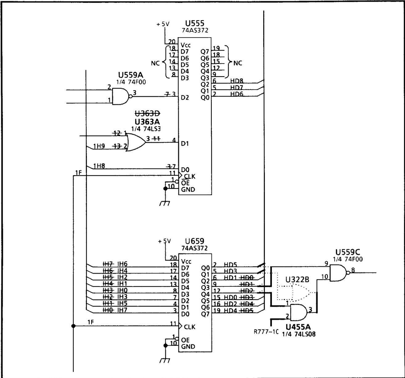
Partial drawing of Schematic 7 showing circuitry changes.
