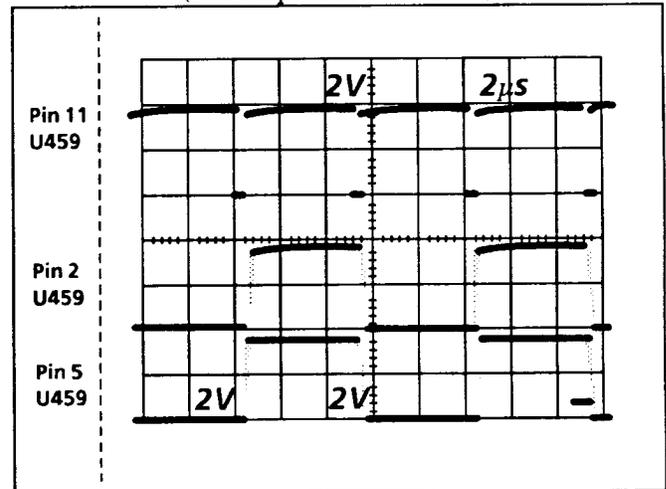
Fig. 7-6. Two LSB outputs (pins 2 and 5) of the Genlock Offset Port (U459, Schematic 1) as  $\mu\text{P}$  switches its I/O data from all 0's to all 1's. The  $\overline{\text{GEN DEL SEL}}$  pulse enables U459.
