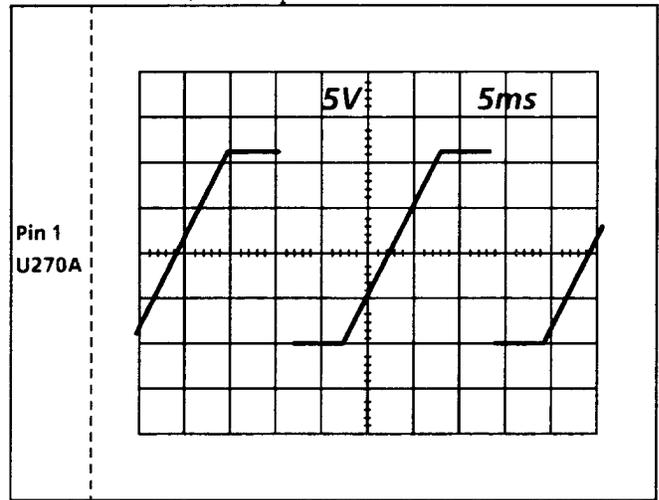
Fig. 7-9. Repeated ramp from pin 1 of integrator U270A. µP generates ramp by counting from 0-255 at a field rate.
