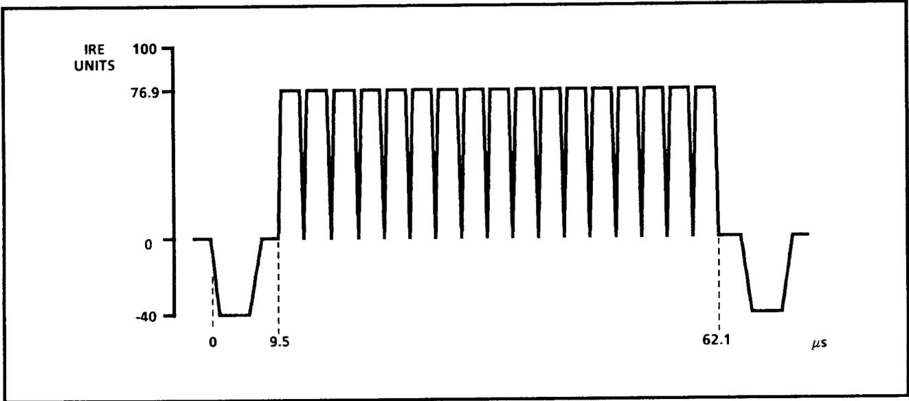
Fig. 3-2a. Horizontal component of Convergence test signal.
