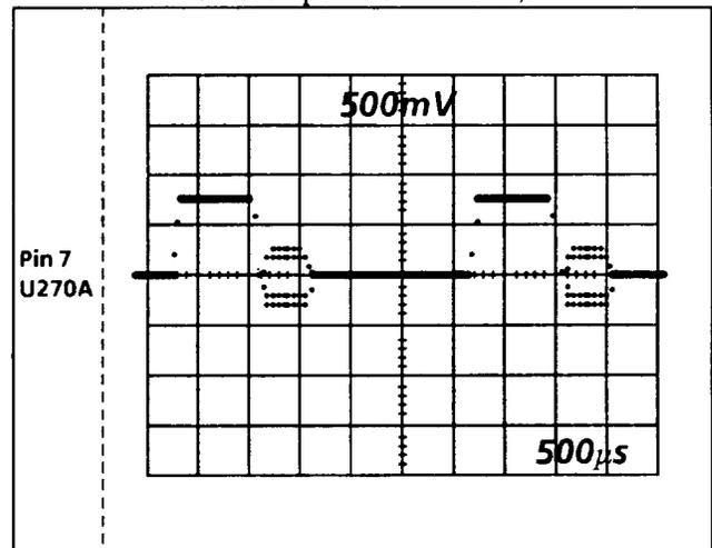
Fig. 7-10. Shows a µP-generated reconstruction of sync and burst at pin 7 of U270. Reconstruction shows the relative timing and amplitude of sync and burst.
