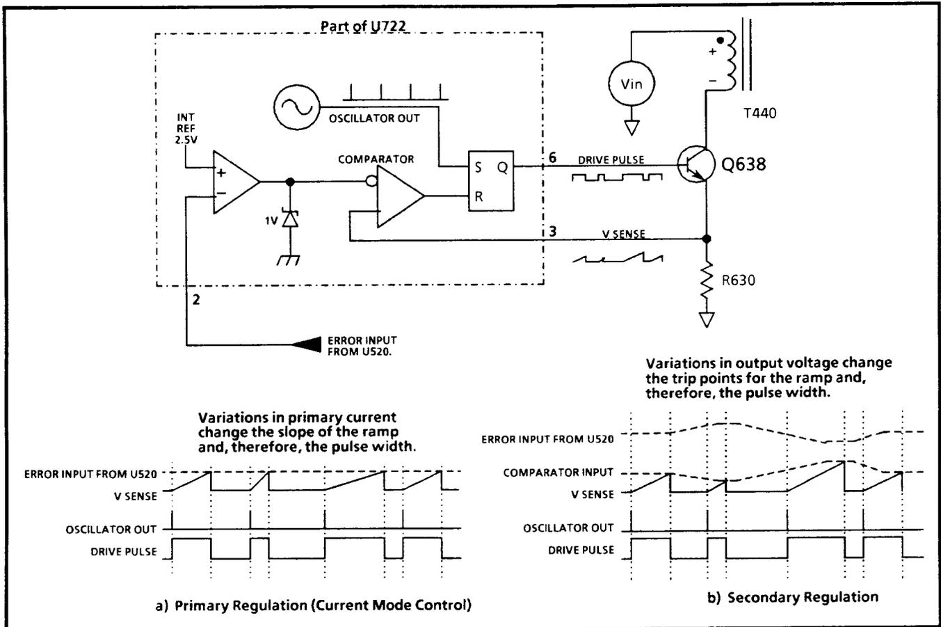
Fig. 6-9. Pulse Width Modulator operation.
