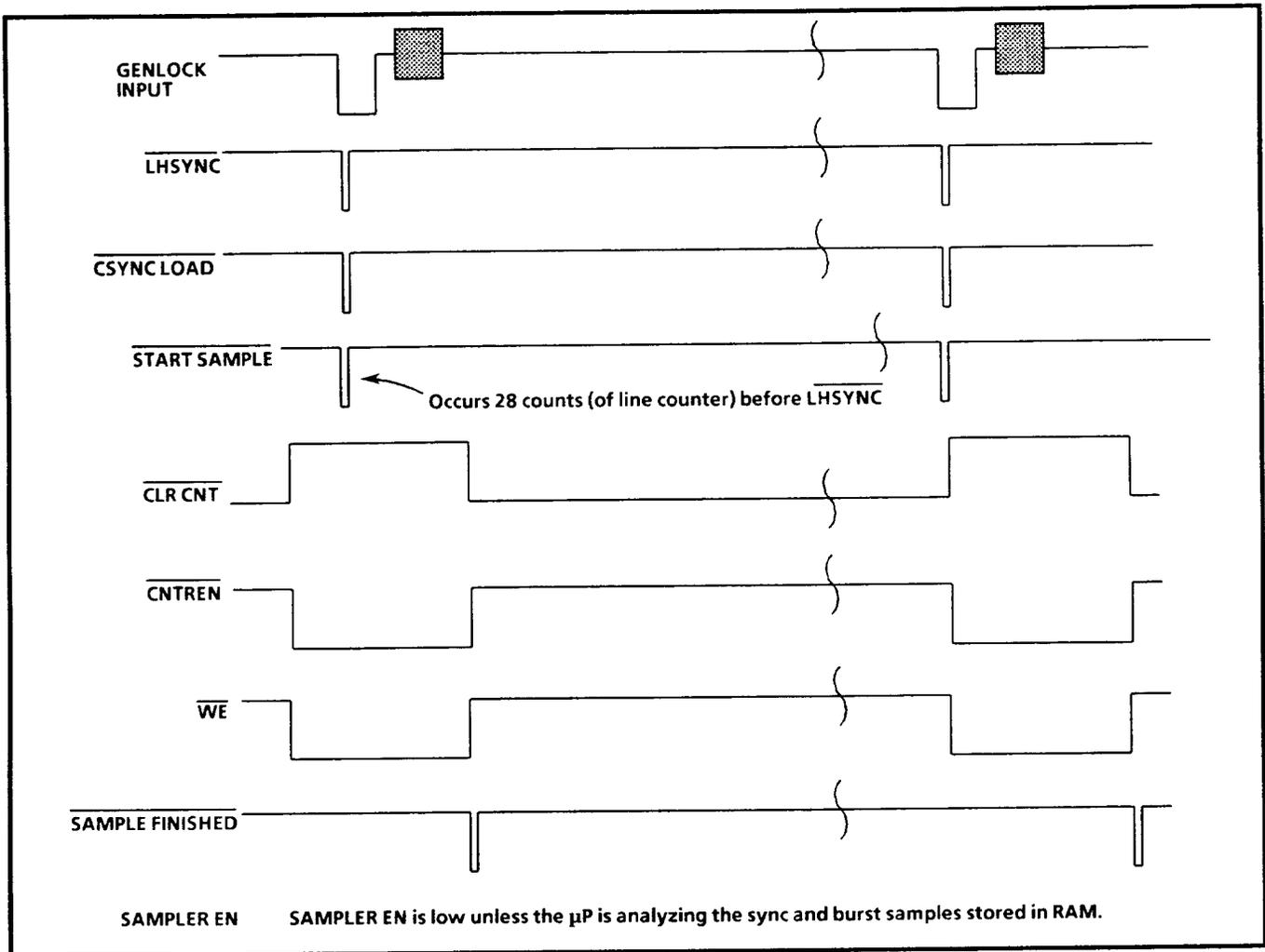
Fig. 6-2. Timing for Memory Controller and Address Counter outputs.
