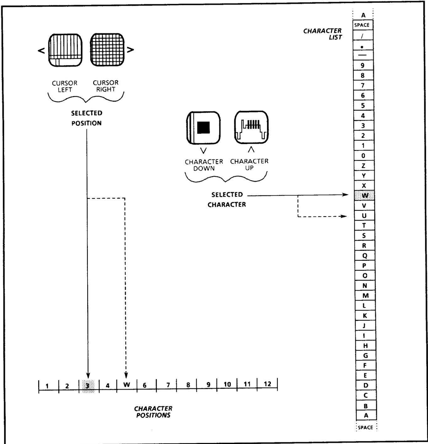
Fig. 2-4. Selecting Option 1 characters from the front panel.
