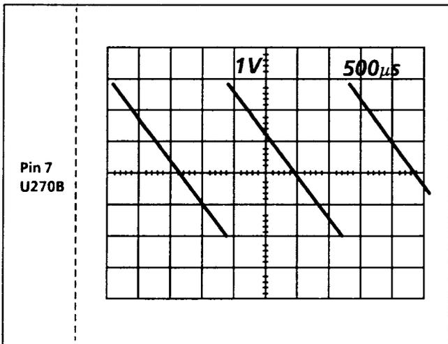
Fig. 7-8. Shows the ramp output at U270B (Schematic 4). µP generates ramp by sending a repeated count of 0-255 to Sync DAC (U370). R173 must be fully clockwise to get an unclipped ramp.
