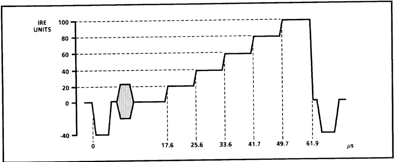
Fig. 3-5. 5-Step Staircase.
