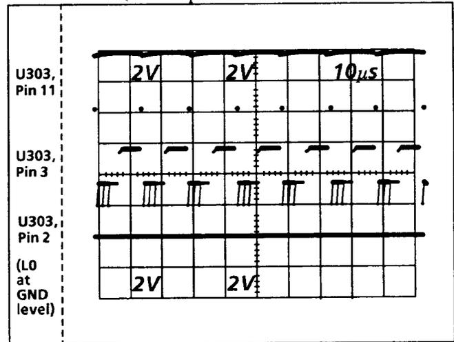
Fig. 7-14. Shows LED0 repeatedly loading a zero into the ED0 input (pin 3) of LED latch U303 (Schematic 1). This holds the L0 output (pin 2) on U303 low to light the DS229 LED. All other LEDs are tested in the same manner.
