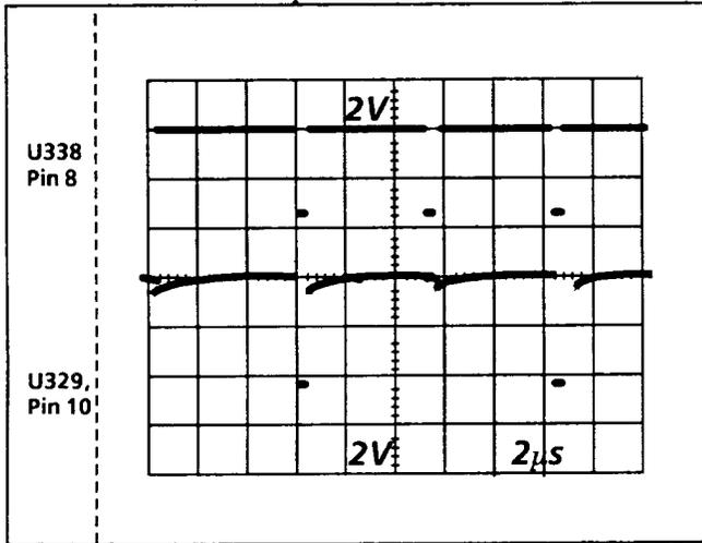
Fig. 7-15. Shows the  $\overline{WR}$  and  $\overline{IO2}$  (Schematic 2) signals asserted to load the character selection codes into the Character RAM.
