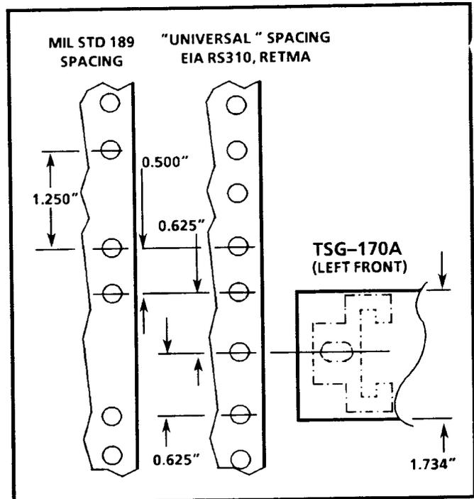
Fig. 4-3. Rail detail for mounting slide tracks.
