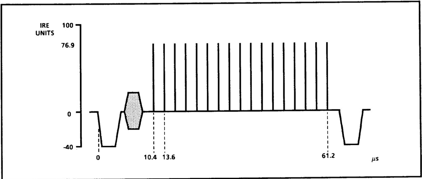
Fig. 3-2b. Vertical component of Convergence test signal.
