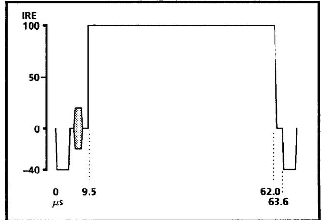
Fig. A-8. Option 1V Field Square Wave (Ver 1.2 and above).
