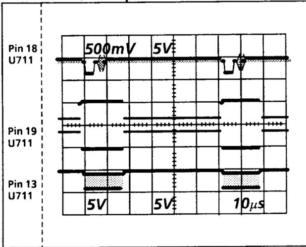
Fig. 7-11. Shows signals through the Genlock Data Acquisition circuit when it is in the UNLOCKED mode.
