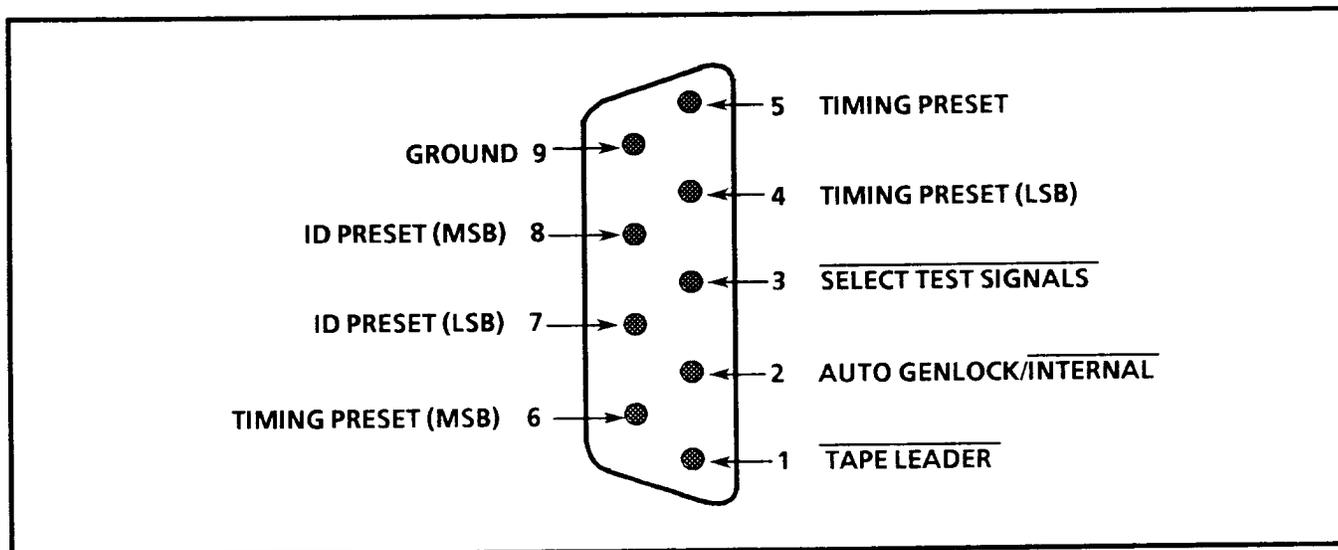
Fig. 2-6. Remote Connector (female) pinout.
