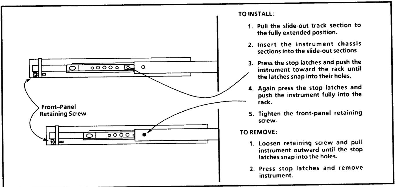
Fig. 4-6. Racking and unranking the TSG-170A.
