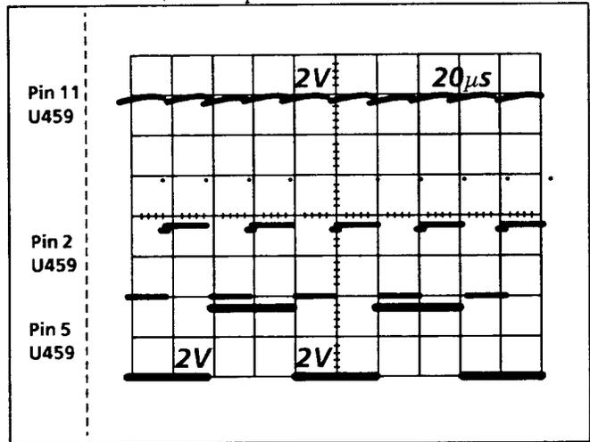
Fig. 7-5. Pin 2, U459 (output LSB), toggling twice as fast as pin 5 (next LSB) as  $\mu\text{P}$  counts from 0-255. Pin 11 ( $\overline{\text{GEN DEL SEL}}$ ) enables U459.
