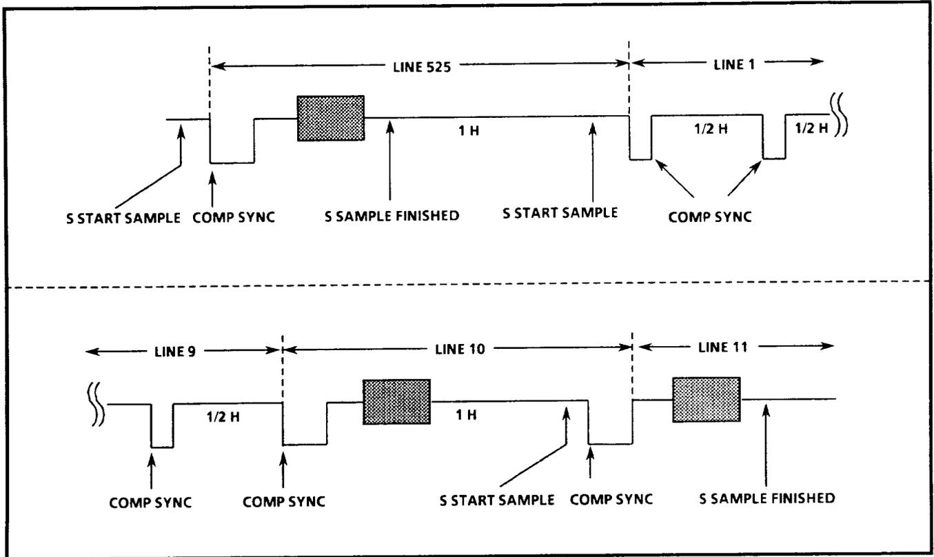
Fig. 6-4. Sequence of S START SAMPLE, COMP SYNC, and S SAMPLE FINISHED around the vertical interval (Fields 1 and 3).
