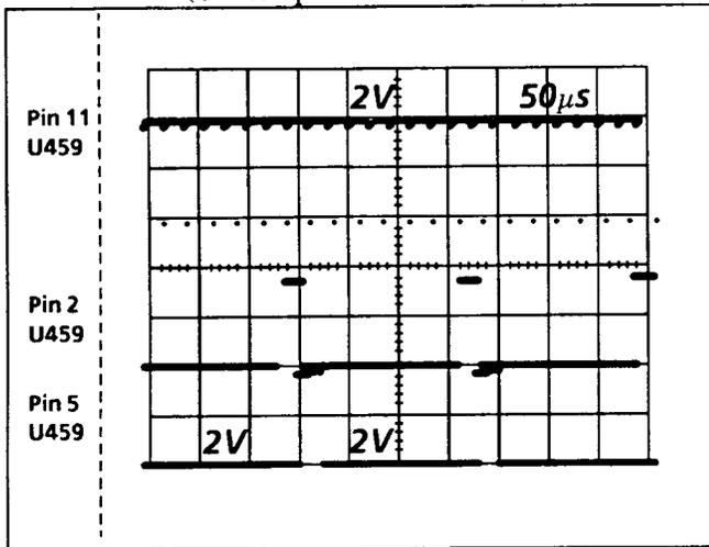
Fig. 7-3. Shows a shifting 1 through the two LSB outputs of the Genlock Offset Port (U459, Schematic 1), as well as the Enable Pulse ( $\overline{\text{GEN DEL SEL}}$ ).
