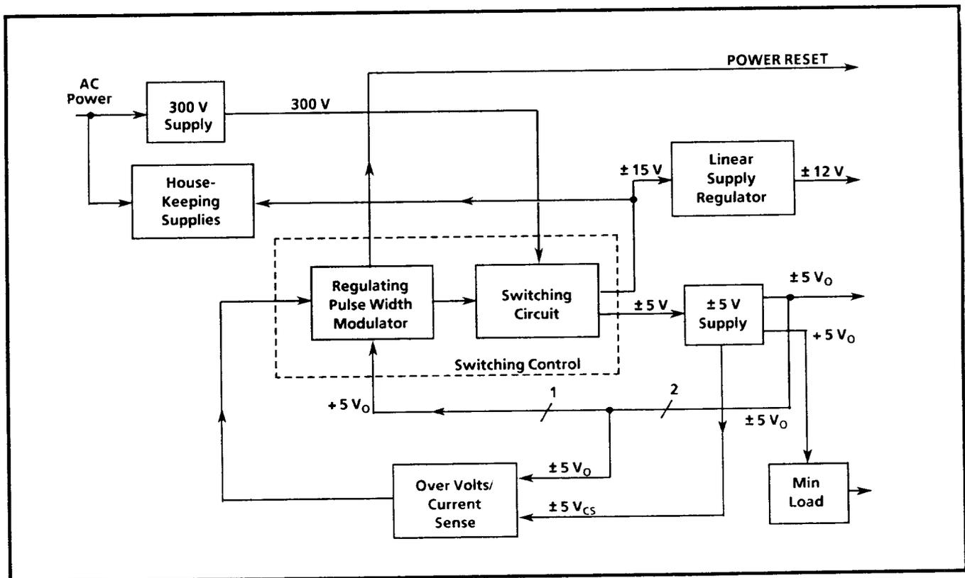
Fig. 6-7. Block diagram of Power Supply.
