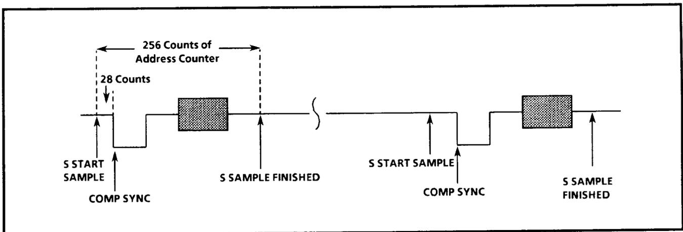
Fig. 6-3. Sequence of  $\overline{\text{S START SAMPLE}}$ ,  $\overline{\text{COMP SYNC}}$ , and  $\overline{\text{S SAMPLE FINISHED}}$  during the horizontal interval.
