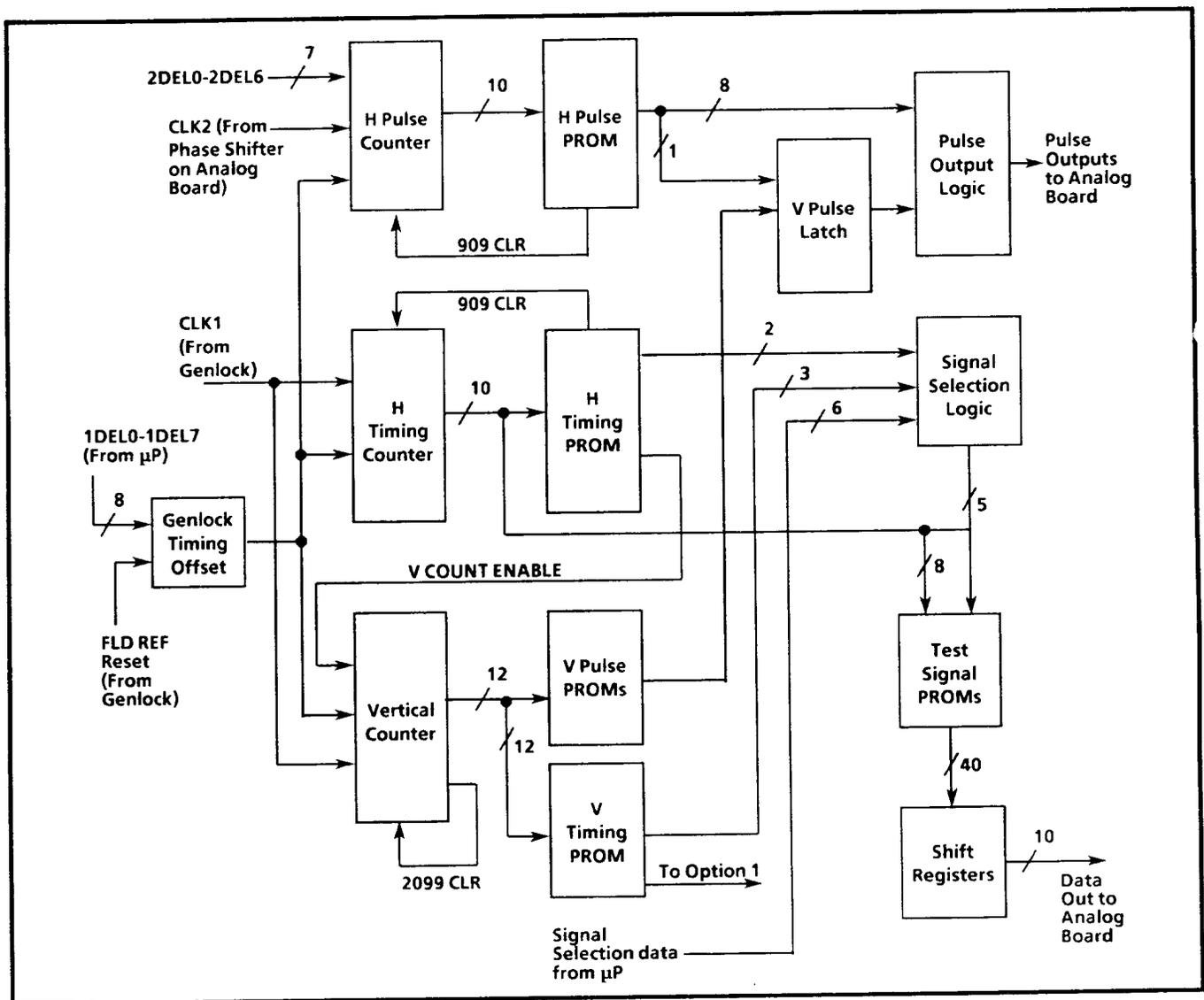
Fig. 6-5. Block diagram of Signal Generation circuits.
