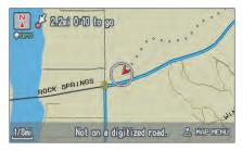
The map screen starts displaying a series of dots (breadcrumbs) to show the path you have taken if **Off-road Tracking** on the Setup screen (second) is set to **ON** (see page 101).
