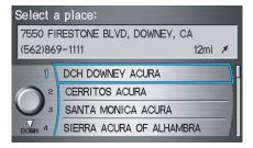
The distance and direction to the destination at the top of the list are shown in the screen. The distance shown is straight line distance (as the crow flies), not driving distance. Say or select the number (1-4) of the desired destination from the list.
