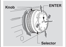
The Interface Dial moves left, right, up, and down. Use the Interface Dial to look around a displayed map. Moving the Interface Dial up or down can also be used to scroll up or down a page in a list. You can also rotate the Interface Dial knob to move the highlighting around the display or to scroll through a list. After making a selection in a menu or list, push in on the Interface Dial (ENTER button) to enter the selection into the system.
