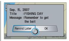
The Calendar reminder screen remains displayed until you select **OK** or **Remind Later** by rotating the **Interface Dial knob** and pushing in on the **Interface Dial**, or press the **CANCEL** button.
