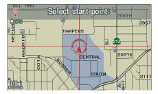
Rotate the **Interface Dial knob** to select the map scale (available scales are 1/20, 1/8, and 1/4 mile scales). Use the **Interface Dial** to move the crosshairs (red circle) to the desired start point and push in on the **Interface Dial** to "set" the start point. Then move the **Interface Dial** in a straight or diagonal direction to encompass the area to be avoided.
