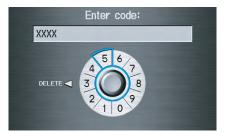
Enter the four-digit security code. If you have entered it correctly, the display changes to the Disclaimer screen. If you make a mistake, the system will display "INCORRECT PIN." Re-enter your 4-digit security code. You have ten chances to enter the correct code. If all ten are incorrect, turn the ignition to OFF, then back to ON (II) to have ten more chances to enter the correct code.
