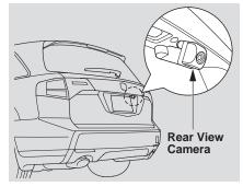
Whenever you shift to R (Reverse) with the ignition switch in the ON (II) position, the rear view is shown on the navigation system screen. For the best image, always keep the rear view camera lens clean, and be sure it is not covered
