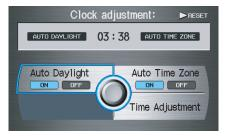
Clock Adjustment allows you to set Auto Daylight Savings, Auto Time Zone, and Time Adjustment. The factory setting is **ON** for both.
