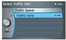
In the example above, only **Traffic lcons** is selected and will show up on the map. To also see **Traffic Speeds** flow on the map, this would need to be turned on by first selecting it and then pushing in on the **Interface Dial** to select it so it appears as below.
