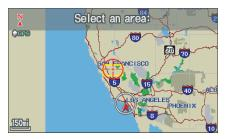
Use the **Interface Dial** to move the cross hairs to the area of the state close to your intended destination. If desired, rotate the **Interface Dial knob** to change the map scale. When you have the cross hairs in the desired area, push in on the **Interface Dial**. The map scale changes to a closer view.
