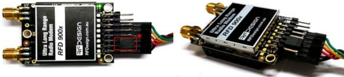
Figure 17 - Modem connected to FTDI cable (pins 1,3,5,7,9,11) to enable serial communications. *Jumper (pins 4&6).
