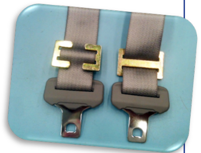
Either Installation of the Locking Clip is Correct
