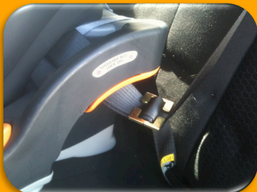
Locking Clip Installed Incorrectly on the Retractor Side of the Belt (Away from the Buckle)
