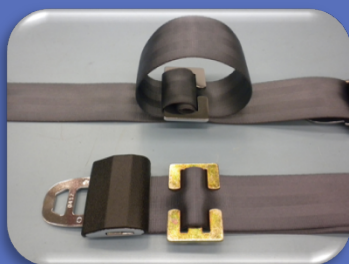
Properly Used Belt Shortening Clip (Top) and Properly Used Locking Clip (Bottom)
