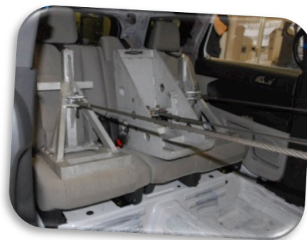
Test Devices for Lower Anchor and Top Tether Anchor Strength Testing
