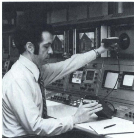
Luminance Measurement of a Monitor with J16/J6503.
