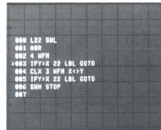
Waveform Processing: Keystroke Programming enables the user to design measurement routines tailored to individual tests or experiments.
