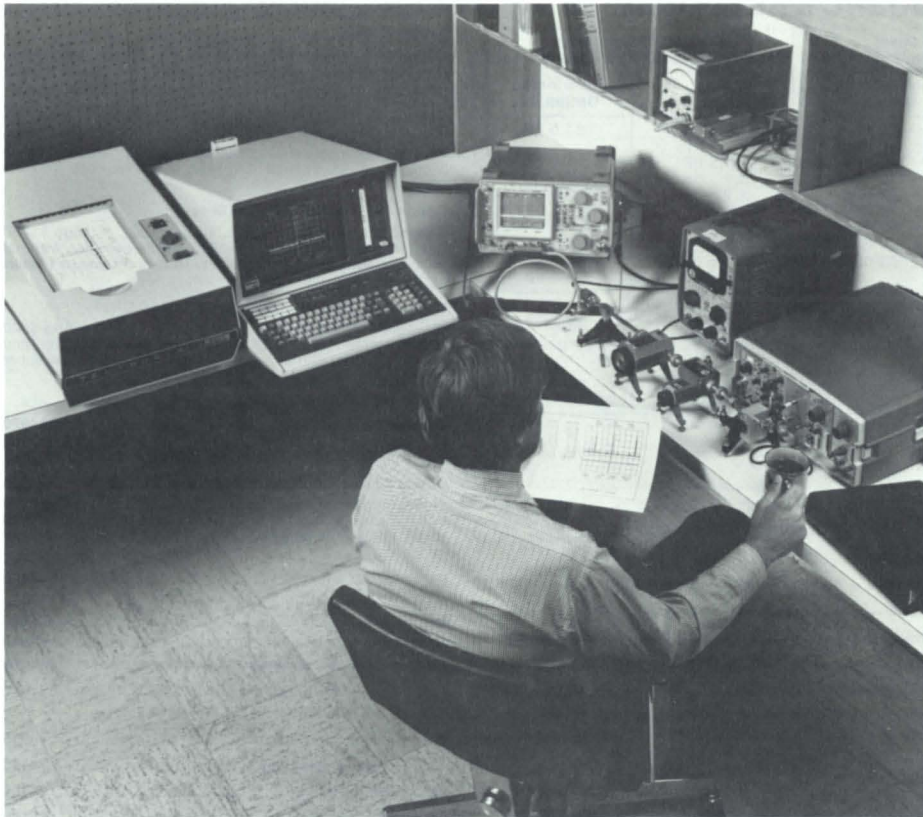
When used with the TEKTRONIX 4052 Graphic Computing System controller and 4631 Hard Copy Unit, or with the 4662 Digital Plotter, the 492P can provide test results in both graphic and numeric form for the evaluation of microwave signal sources.
