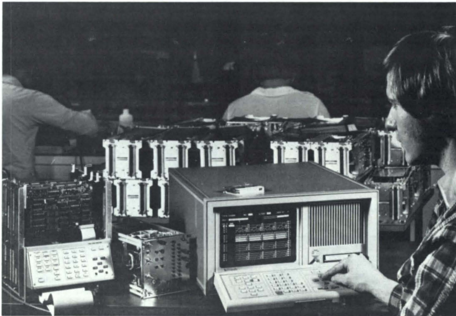
With pattern generation and data acquisition in a single instrument, the DAS 9100 is useful in manufacturing test areas.
