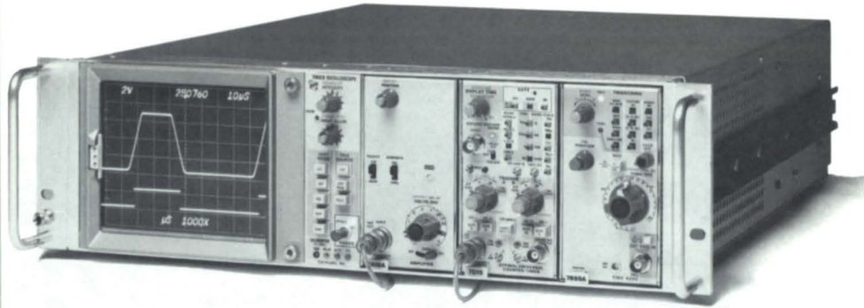
The R7603 requires only 5.25 in of rack height in a standard 19 in rack. It is fan cooled and comes complete with slide-out chassis tracks.
