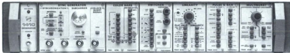
1410R Mainframe with SPG2, TSGs 7, 3, 5, 6 and TSP1 installed.
