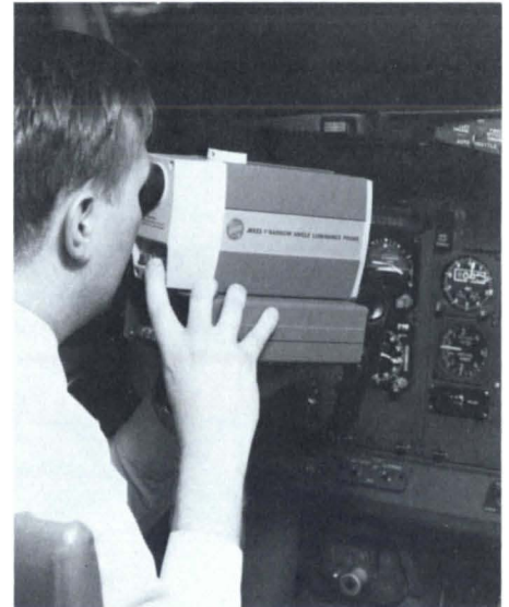
Measuring Luminance with the TEKTRONIX J16/J6523.
