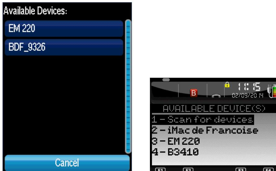
Select the device you want to pair. If the device does not appear, wait some time (GOAL terminals) or hit *Scan for devices* (Libgr terminals).
