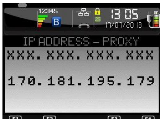
Enter the IP address of the terminal (supplied by the administrator of the local network). IP Address is composed of four digital fields, each one from 0 to 255.
