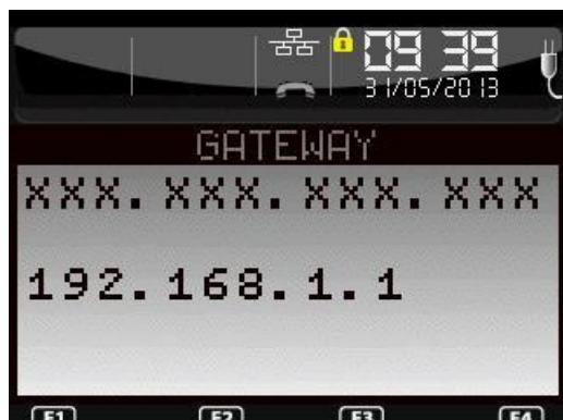
Enter Gateway address (supplied by the administrator of the local network) which is the IP address of the machine used by gateway to join other networks.
