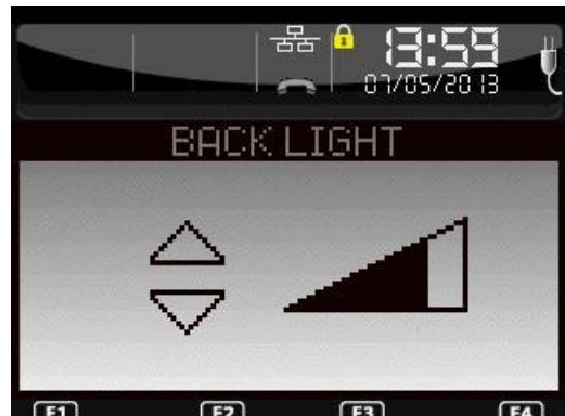
Adjust the intensity of the backlighting using the "up" or "down" keys of the navigator. Then validate.
