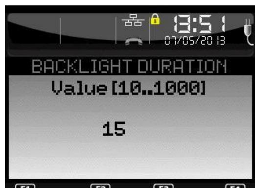
Enter the duration of the backlighting (in seconds, from 10 to 1000). Then validate.
