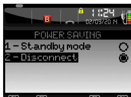
Select "Standby Mode" to maintain the Bluetooth connection with devices if the terminal is in standby mode. In this case the terminal can be woken up from smartphone or tablet. The Bluetooth connection will be maintained in a low energy mode to reduce the battery usage.
