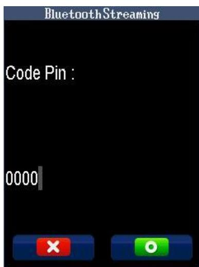
Enter the pin code furnished by the headset to unlock the connection. Then validate.
