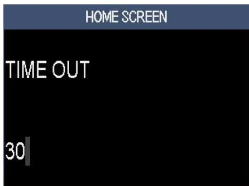
Enter the duration (in seconds) of the home screen display before switching on the "idle screen". Then validate.
