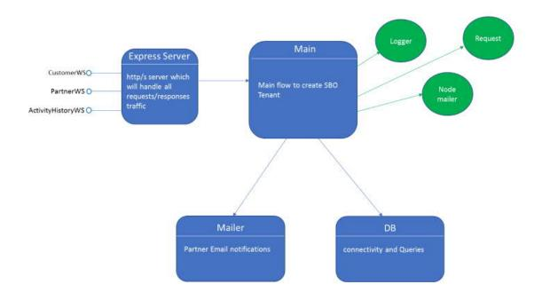
As can be seen from the diagram, the server exposes 3 interfaces to the front-end client: one for the customer configuration page, one for the tenant configuration wizard and another for the activity history – each interface has several methods in it that servers the relevant client page.
