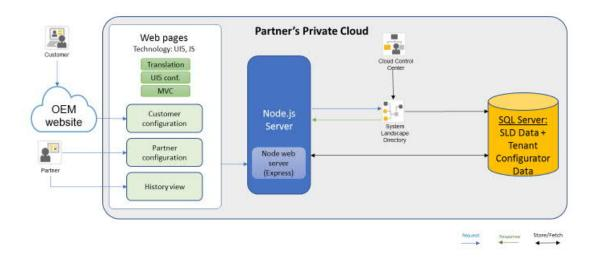
As can be seen from the diagram, the solution is composed from a front-end Java script GUI, based on Fiori, SAPUI5 and a back-end, based on Node .js. The data can be stored on any SQL Server you have. In order not to increase the TCO with a new DB server, you can store it on the same SQL server of the SLD, as illustrated in the diagram,
