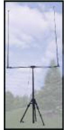
Tactical Repeater Antenna Configuration
