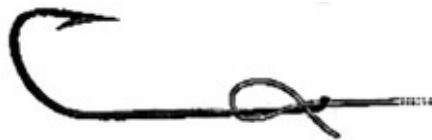
Principle of the Jam Knot on a Bare Hook, Magnified.
