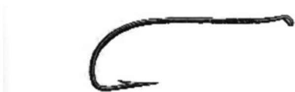
New Patent Salmon Hook with Up-Turn Shank and Down-Turned Eye.
