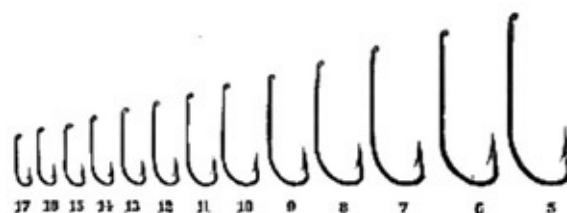
Old Pattern of Turn-Down Eyed 'Pennell-Limerick' Hooks.
