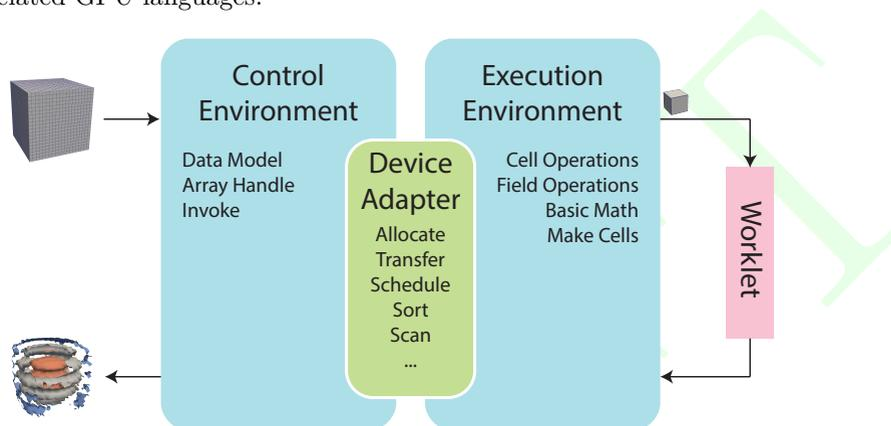
Figure 6.1: Diagram of the VTK-m framework.
