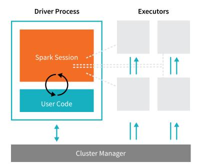
The cluster manager controls physical machines and allocates resources to Spark Applications. This can be one of several core cluster managers: Spark's standalone cluster manager, YARN, or Mesos. This means that there can be multiple Spark Applications running on a cluster at the same time. We will talk more in depth about cluster managers in Part IV: Production Applications of this book.
