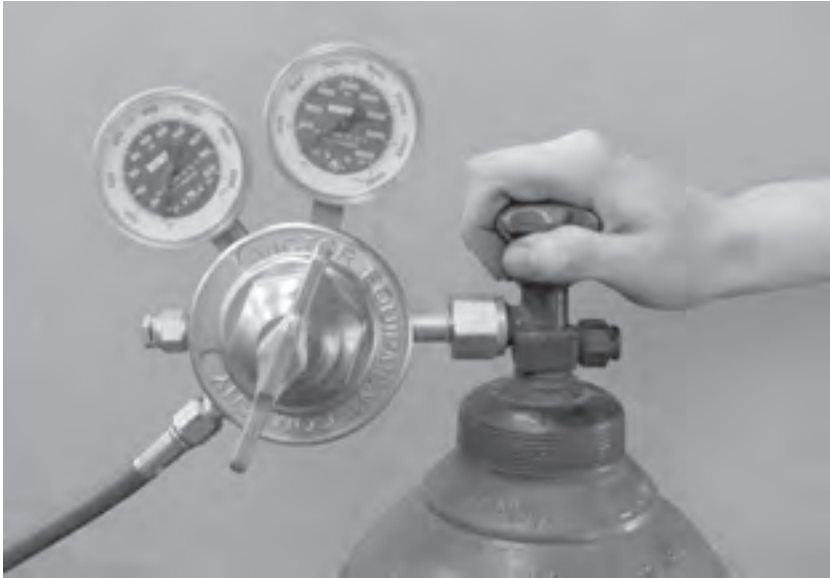
Figure 10: Opening the Cylinder Valve
