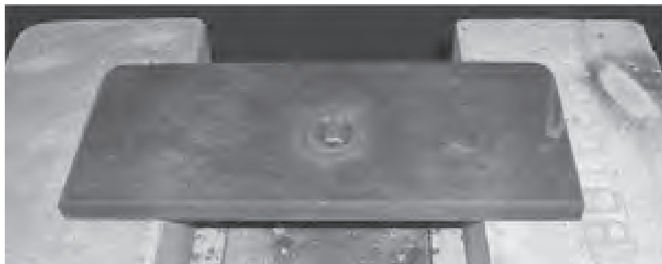
Figure 22: Cutting by Piercing
