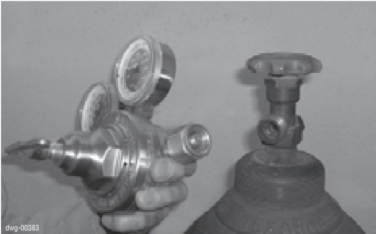
Figure 9: Inspecting the Cylinder and Cylinder Valve
