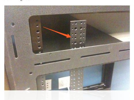
The back and middle mounting points are where you typically want to attach the rack rails to your rack. If you don't have a middle mounting point, then you'll have to use the front mounting point.
