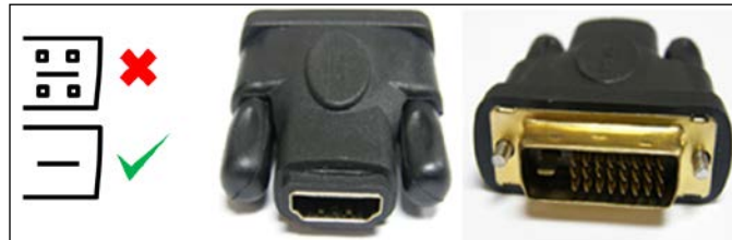
HDMI-to-DVI connection (DVI-D adaptor)
