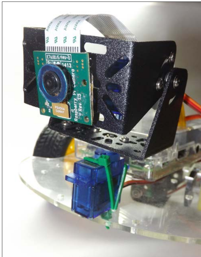
The Raspberry Pi camera can be controlled using a servo mount
