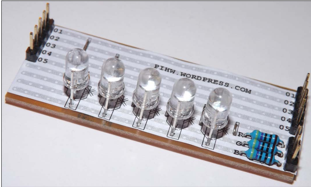
The RGB LED module from PiHardware.com
