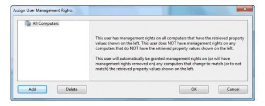
This dialog displays the current set of computers that can be managed by the selected Console operator and lets you add or delete computers from that set. There are two buttons in this dialog:
