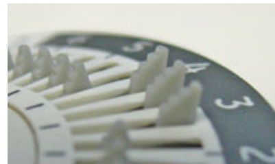
Pins out = Timer ON
