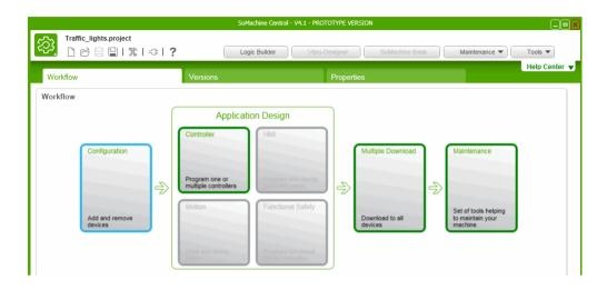
Controller selection is done from the Configuration block and is typically the next step in developing a project. If you select the Configuration block, it turns green. Click Manage devices to open thee device catalog
